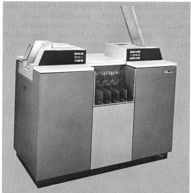
Figure 5. IBM 2540 Card Read-Punch
