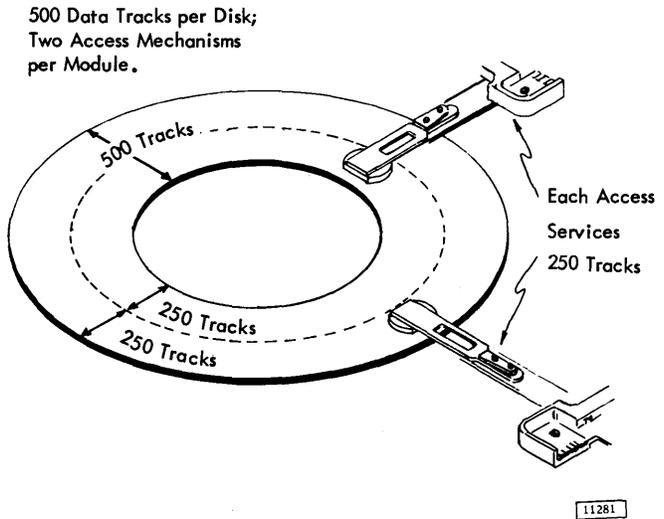
Figure 15. Access Mechanisms
