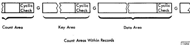
As data is transferred from the CPU to an attached storage device, the 2841 removes the parity bit from each byte. The 2841 then computes two Cyclic Check (cc) bytes which are added to the end of each Data Area. The two Cyclic Check bytes are arithmetically coded to represent the data in the associated area.
