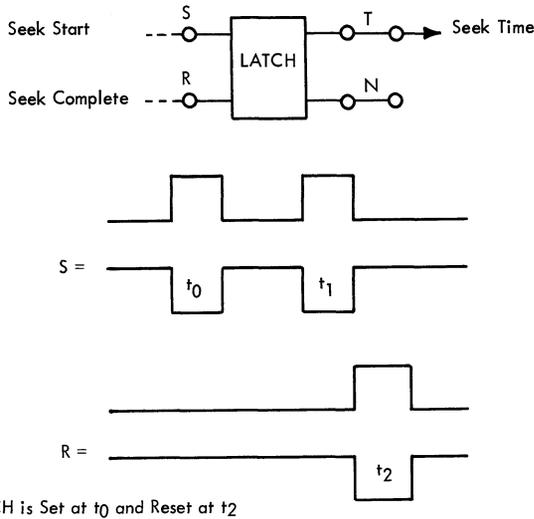
Figure 17. Example of LATCH Function
