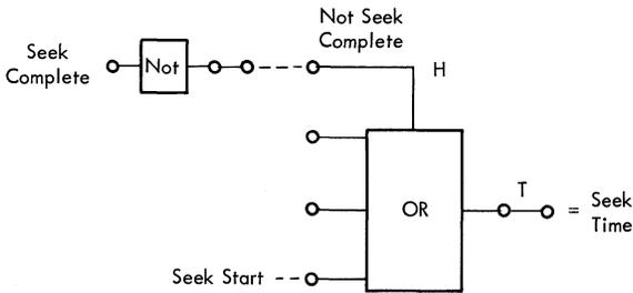
Figure 18. Example of OR LATCH Function
