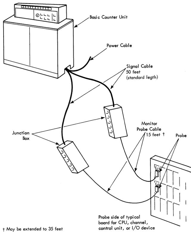
Figure 3. Basic Counter Unit Configuration
