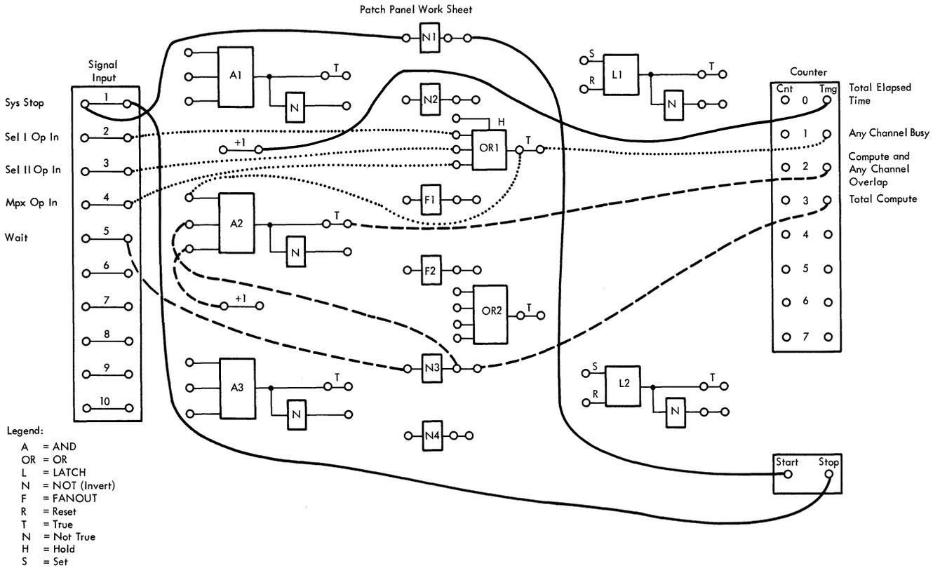
Figure 31. Wiring for Example 1
