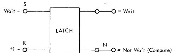
Figure 20. Example of LATCH used as a FANOUT Function
