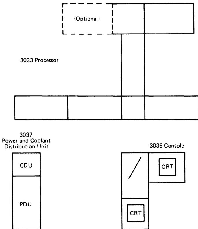
Figure 05.1. Major components of the 3033 Processor Complex
