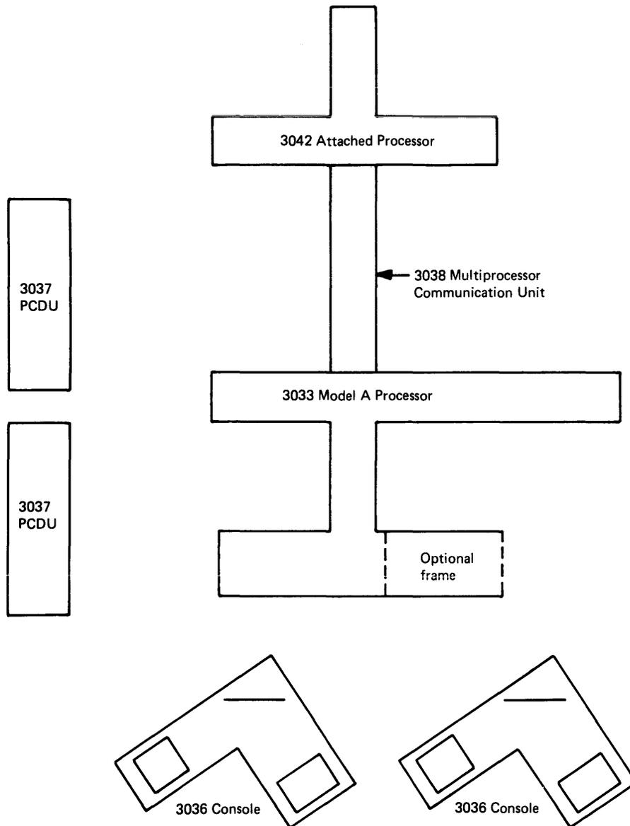
Figure 40.05.1. Components of the 3033 Attached Processor Complex
