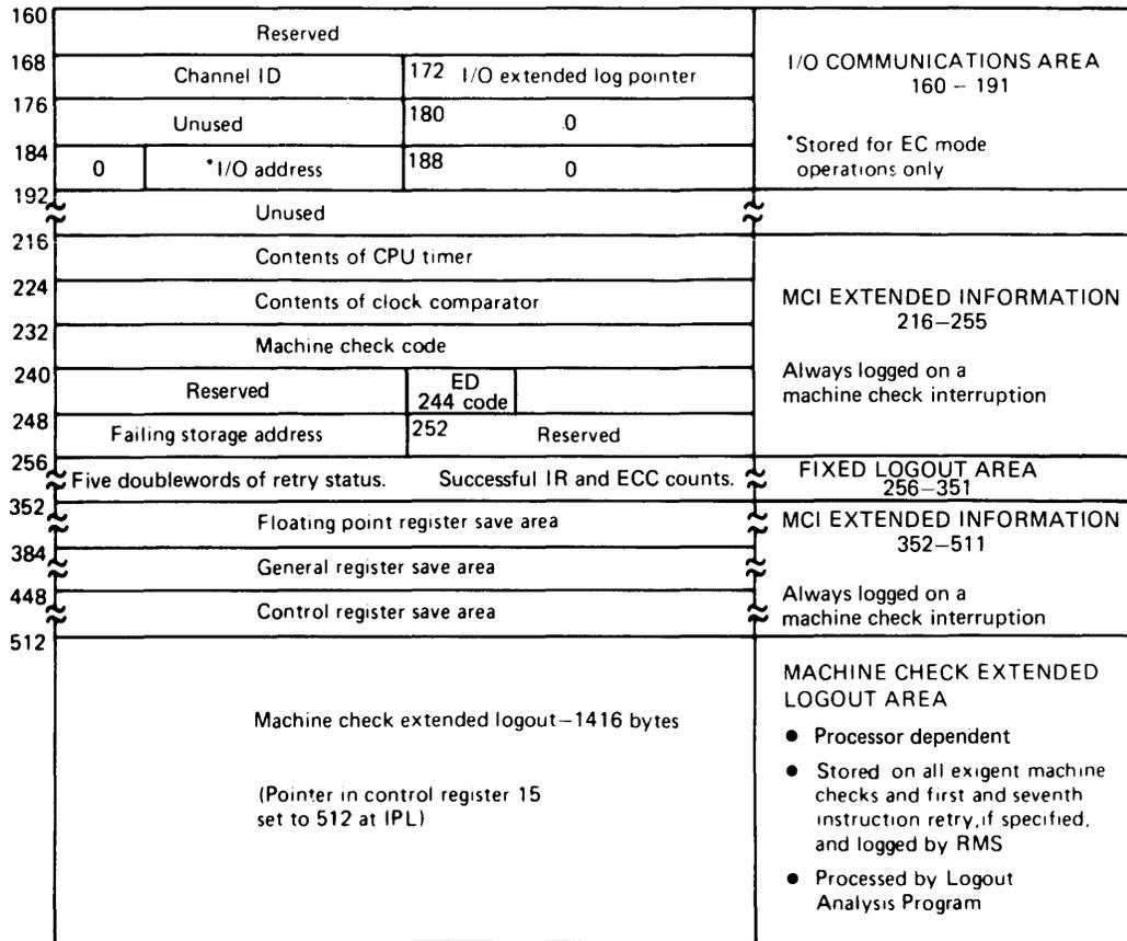
Figure 10.10.1. Processor-dependent fixed storage locations
