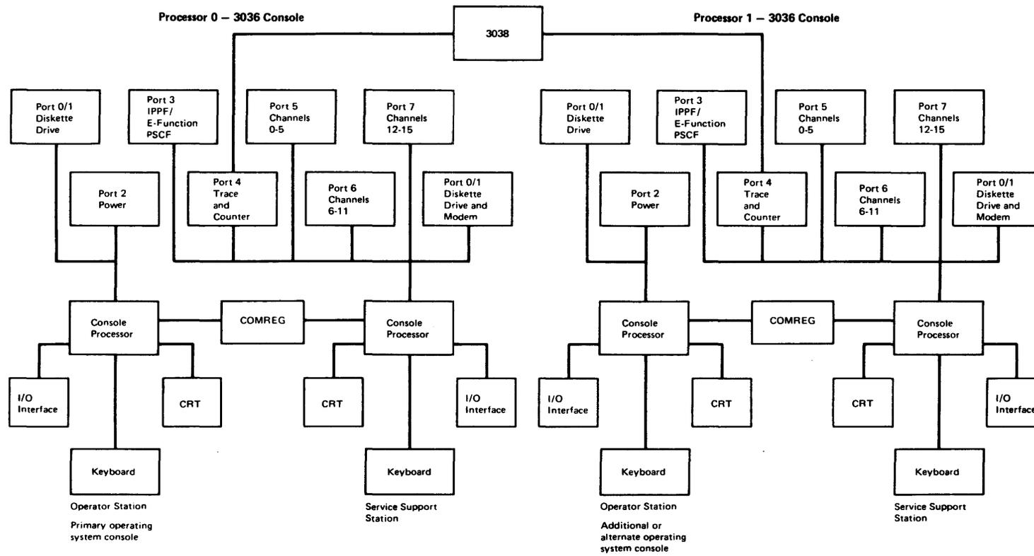
Figure 30.05.2. The normal console configuration for the 3033 Multiprocessor Complex
