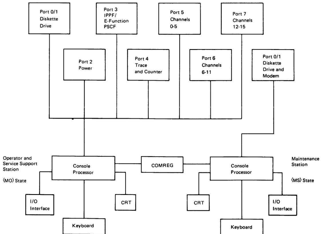
Figure 20.30.2. A maintenance mode 3036 Console configuration
