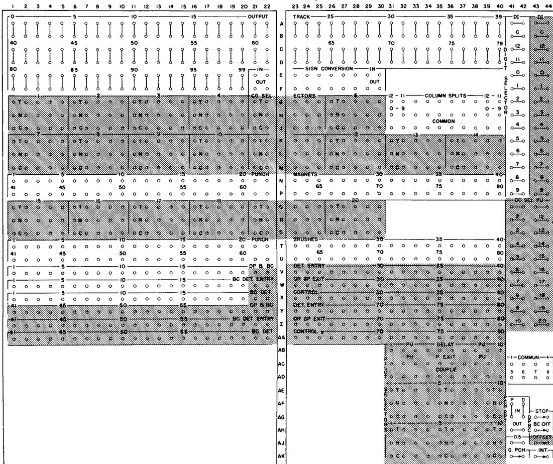
Figure 105. 323 Punch Control Panel
