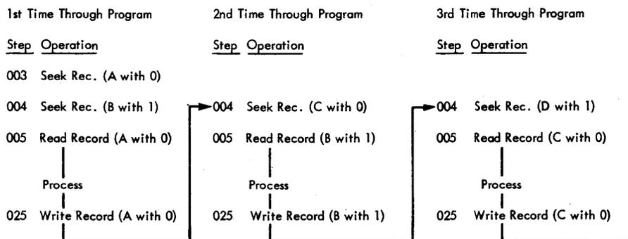
The first seek instruction following a reset condition will be directed automatically to the 0 access unit. On the next seek instruction in the program, access 1 will seek the address sent to the address register and access unit 0 will be conditioned to read or write. Therefore, the next read or write instruction issued will apply to access 0.
