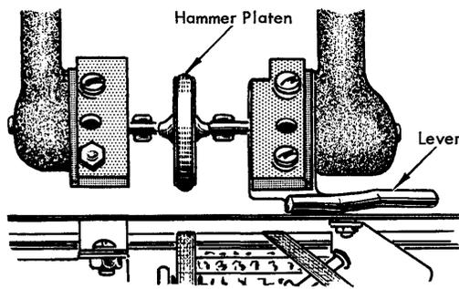
Figure 92. Printer Platen
