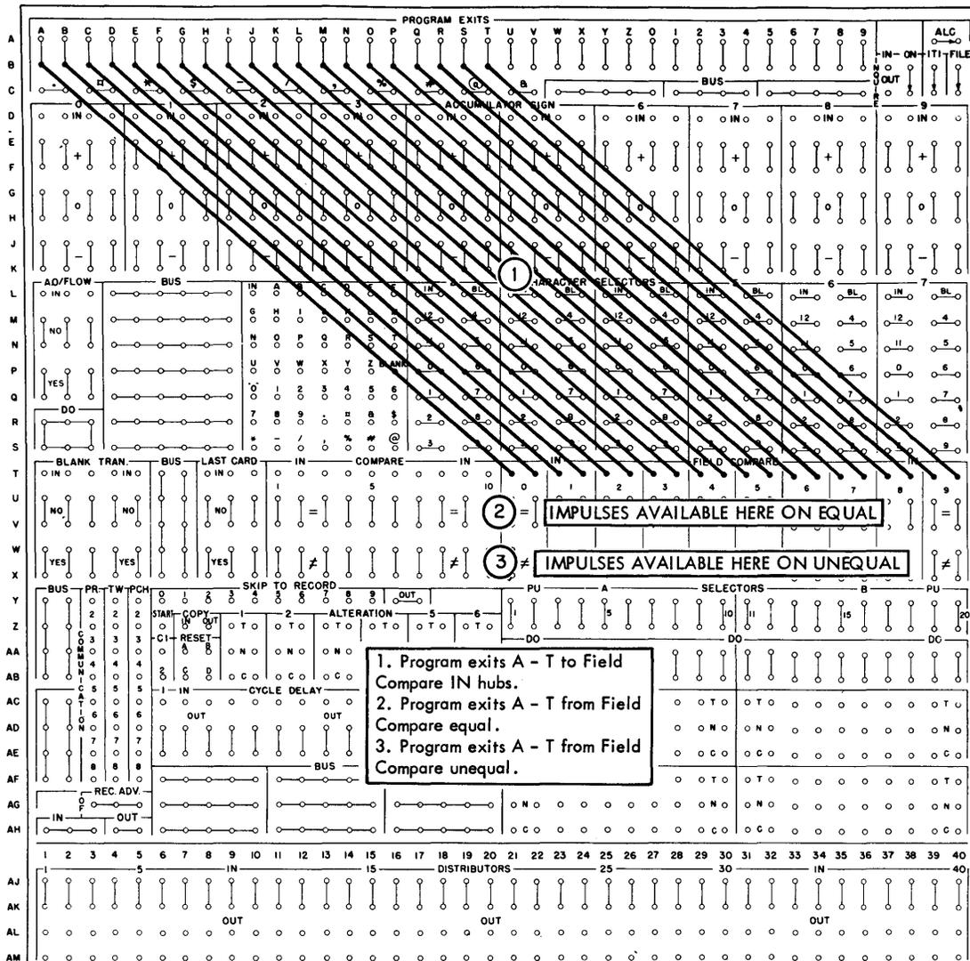
Figure 119. Program Exit Expansion-Field Compare Selectors
