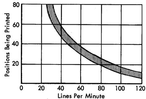
Figure 148. 370 Printer Speeds
