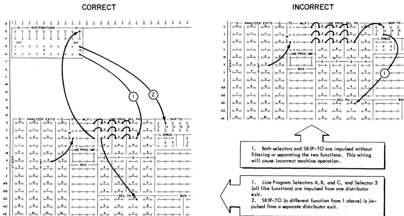
Figure 114. Correct Method of Impulsing Dissimilar Functions
