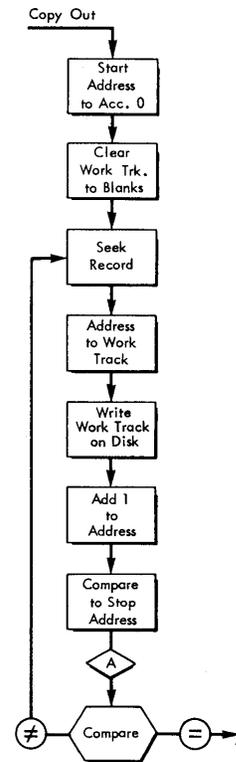
Figure 28. Block Diagram for Clearing Disk Storage
