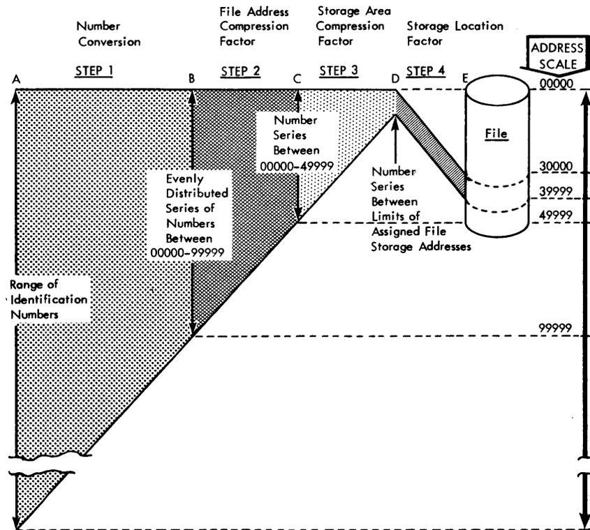
Figure 35. The Four Steps to Indirect Addressing
