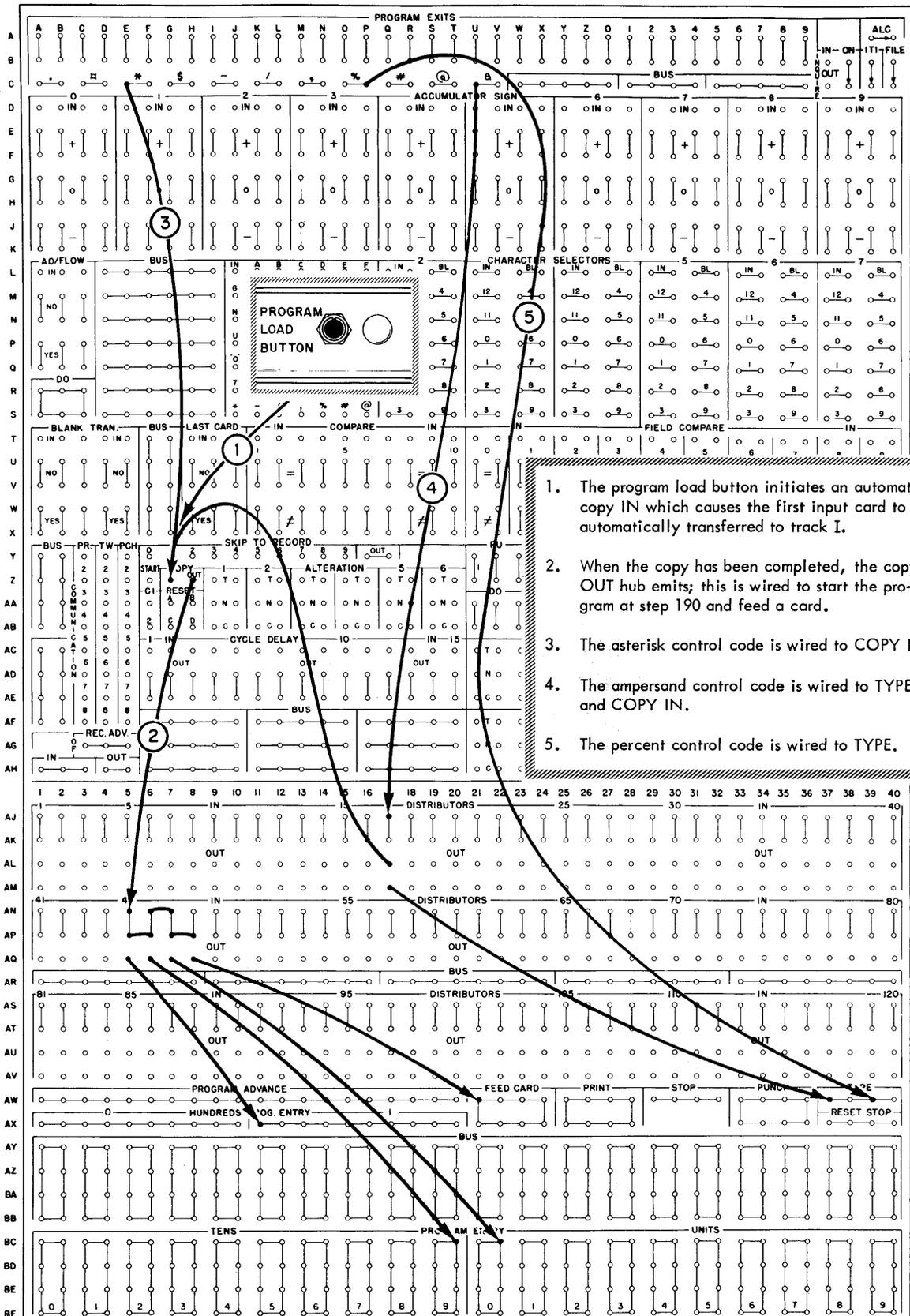
1. The program load button initiates an automatic copy IN which causes the first input card to be automatically transferred to track I.
