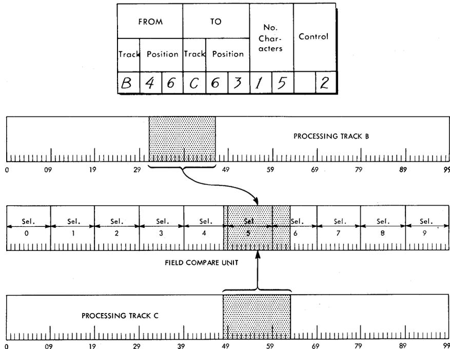
Figure 19. Schematic of a Field Compare Operation
