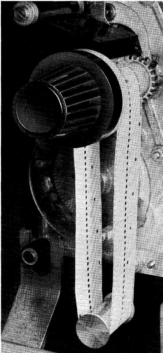
Figure 88. Forms Tractor Positioning Knob
