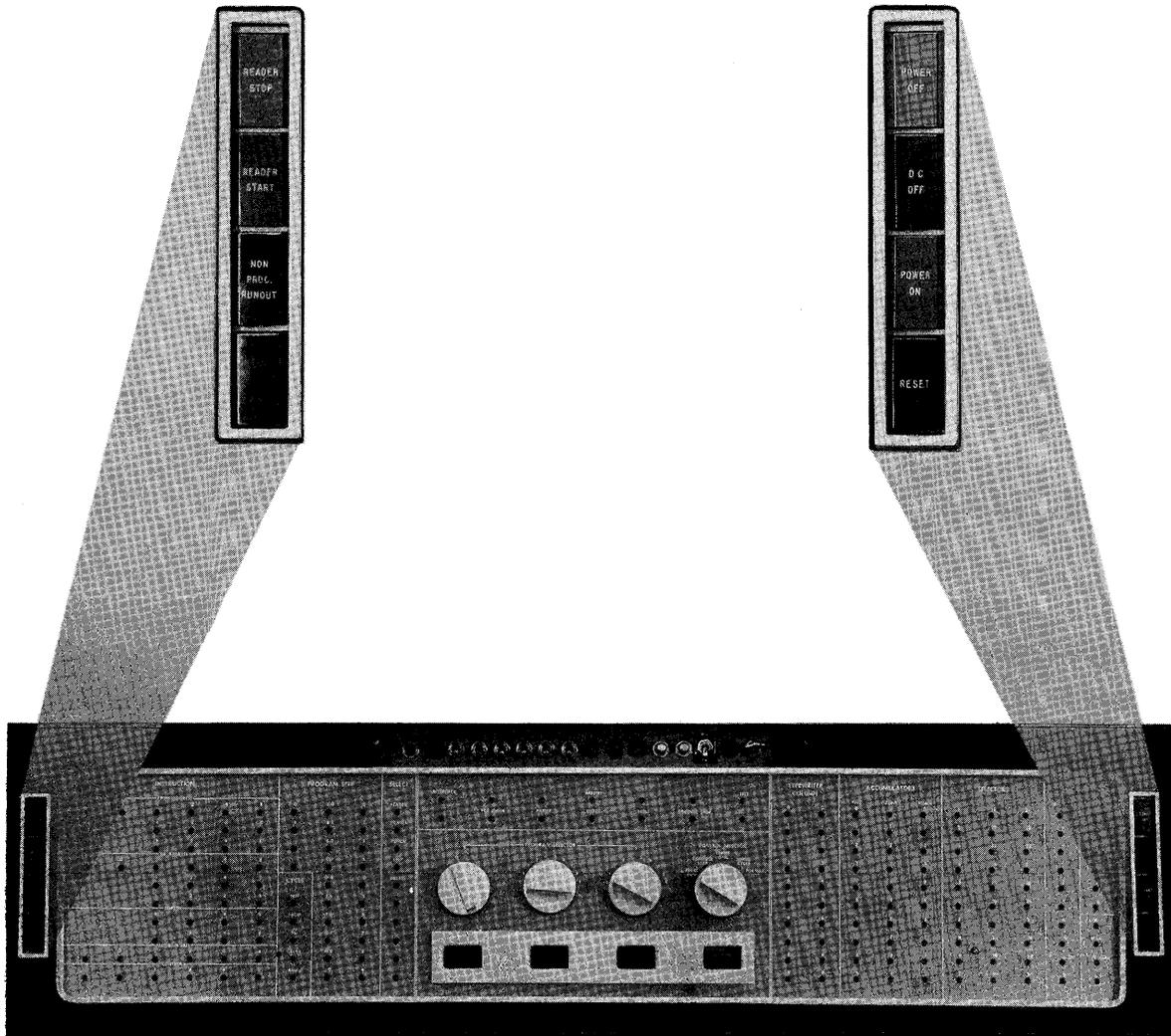
Figure 53. Power, Reset and Reader Keys
