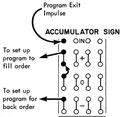
Figure 7. Method of Branching by Control Panel Wiring
