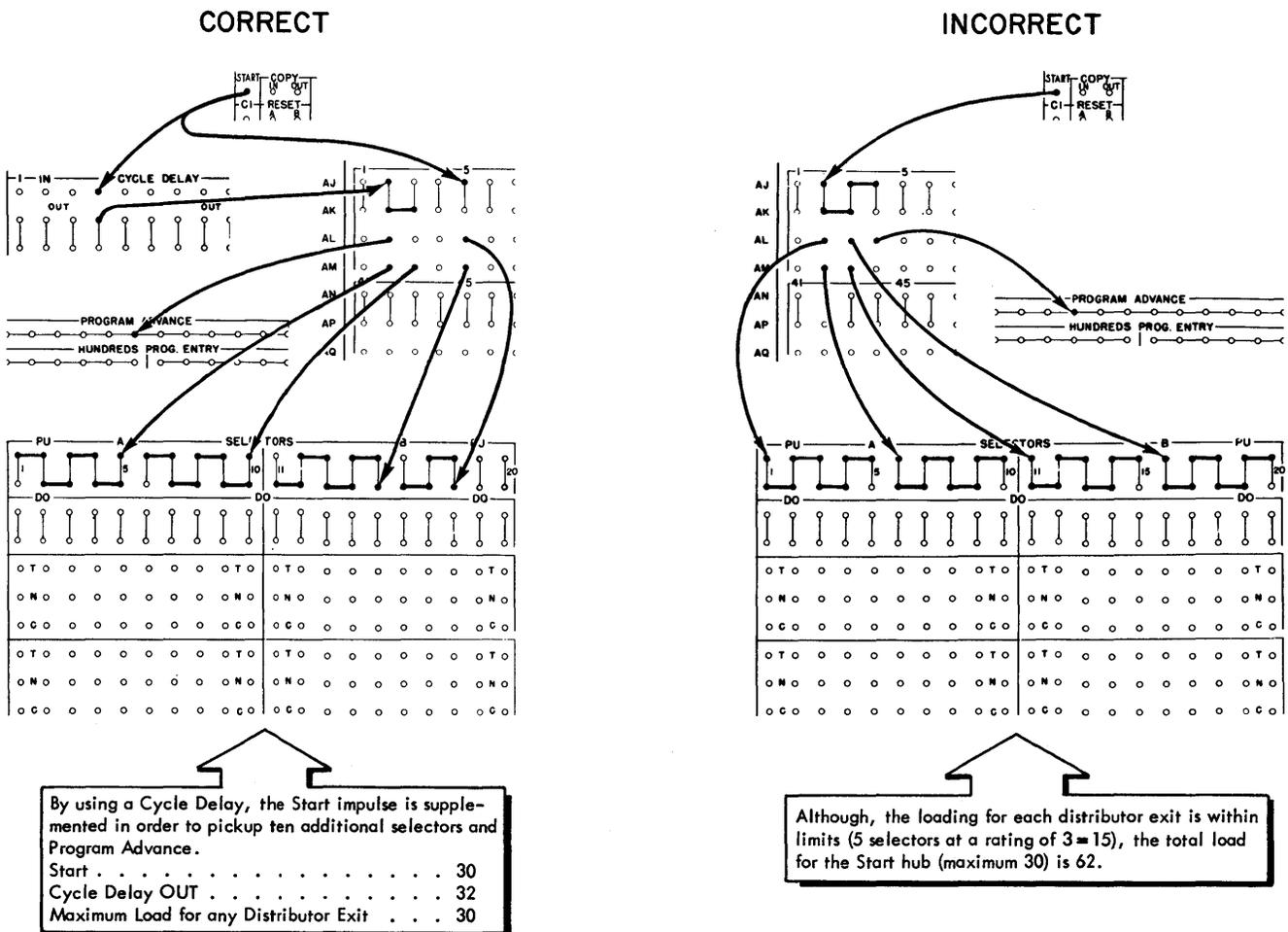
Figure 115. Wiring Based Upon Load Chart Ratings
