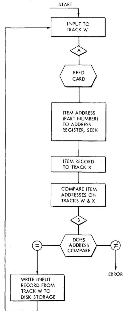
Figure 32. Block Diagram of a Disk Storage Loading Program
