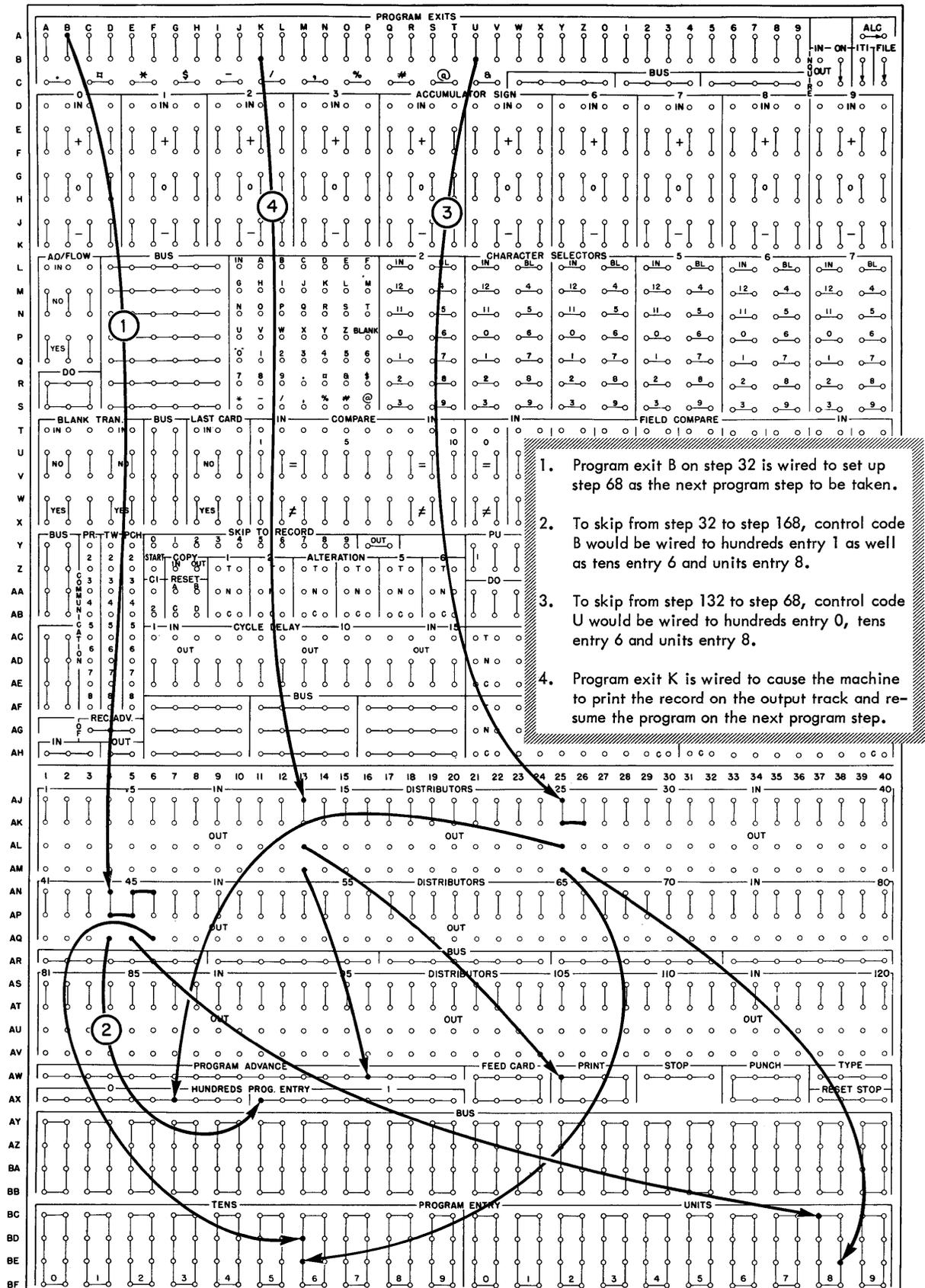
1. Program exit B on step 32 is wired to set up step 68 as the next program step to be taken.
