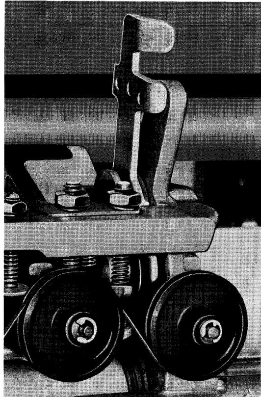
Figure 91. Forms Thickness Adjustment Device
