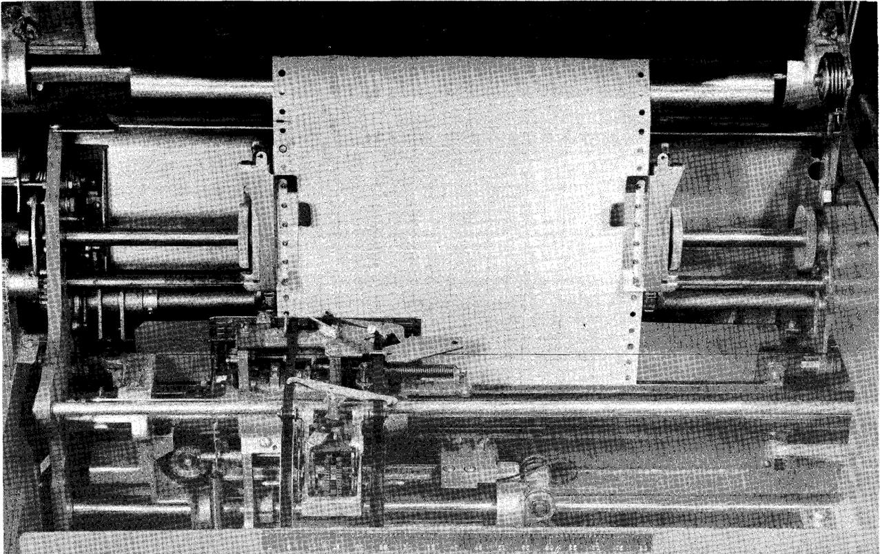
Figure 83. *Tape-Controlled Carriage*
