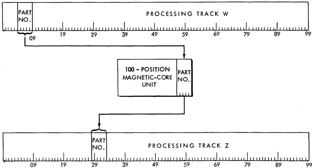
Figure 10. Schematic of a Normal Transfer Operation
