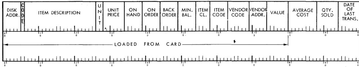
Figure 31. Track Layout of an Item in Disk Storage
