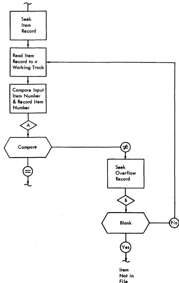
Figure 43. Chaining Method of Seeking a Record
