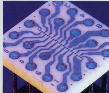
The chips are then joined to ceramic substrates on IBM-designed automated tools. The chips are flipped over, so their circuitry and the C4 pads face downward, and are aligned on the substrates so precisely that each pad makes contact with a corresponding circuit pattern previously screened on the ceramic base.
