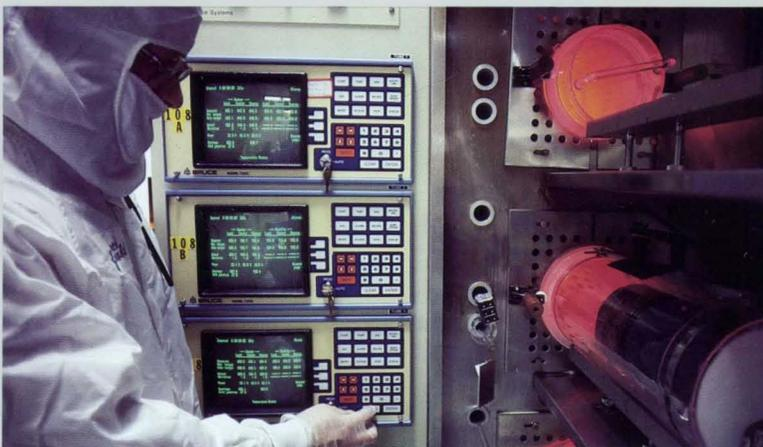
Round wafers of ultra-pure silicon are placed in an oxidation oven, which deposits a layer of silicon dioxide on which each layer of circuitry will be etched.
