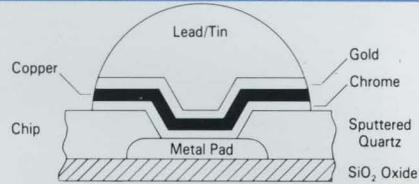
After the chip has been coated with a protective coating, tiny holes are etched down to the metallized interconnections on the chip. At each of these points, metals are evaporated onto the chip to produce small domes, called controlled collapse chip connection (C4) pads.
