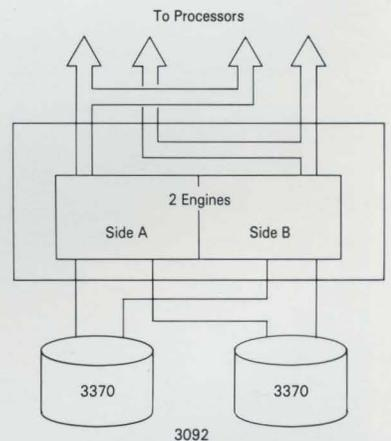
The IBM 3092 Processor Controller can contain one (on the 120E) or two independent processor engines. On the 3092 diagram shown above for a 3090 model 400E or 600E, one is in the active state, monitoring the IBM 3090 processor complex, the other is in standby ready to take over should the active one fail. Also, all key information recorded is duplicated on the two IBM 3370 disks which are connected to both processor engines in the 3092.
