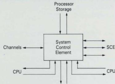
**The System Control Element accepts and processes data requests from the 3090 central processors, storage, and the channel subsystem. The enhanced design of the IBM 3090 System Control Element, implemented with advanced logic circuits, increases system performance, reduces large systems constraints, and contains even more error correction for improved availability.**
