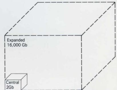
Expanded storage, using a 32-bit addressing structure, extends the system's processor storage capability to over 4 billion 4K pages, or 16 trillion bytes — many times the on-line data in a typical large system installation.
