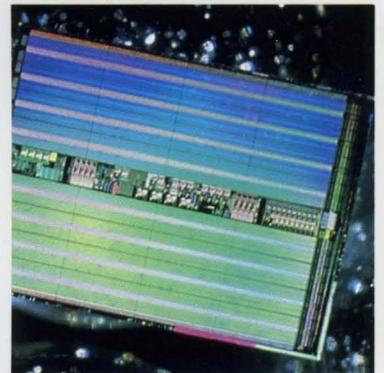
IBM-developed and built one-million-bit memory chips are used in the 3090 processors. This first generation IBM 1-megabit chip is used in 3090 expanded storage.
