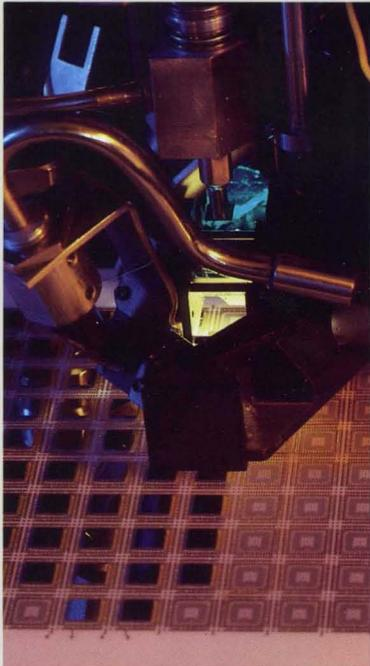
Logic and array chips are mounted on multilayer ceramic substrates and bonded using the IBM-invented C4 process.
