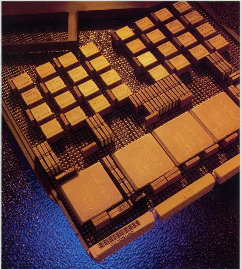
Four megabytes of memory can be stored in this field-replaceable circuit card.
