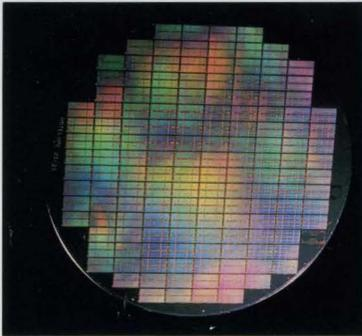
This wafer, 125 mm (five inches) in diameter contains approximately 150 of the newest IBM one-million-bit memory chips. To further enhance manufacturing productivity, IBM is first in the industry to phase in production of these advanced chips on 200 mm (eight-inch) wafers. The new 200 mm wafers can hold almost three times as many chips as the 125 mm wafer.
