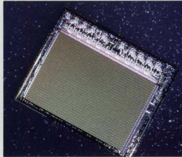
Specially-developed array chips for control storage, working storage and directory applications are packaged on the 132 position MLC substrate next to the logic chips for faster access.
