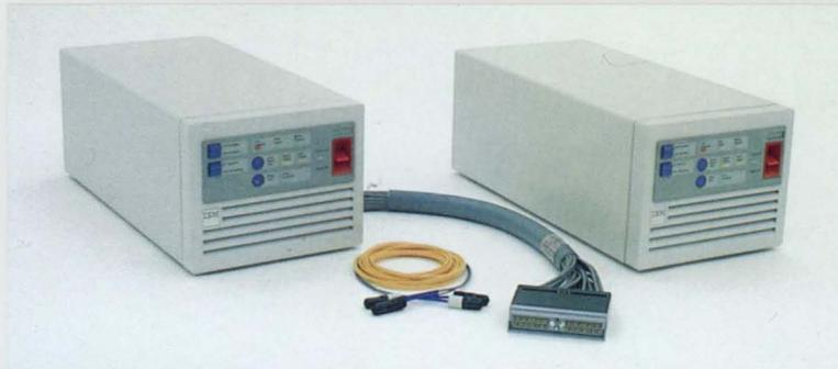
The IBM 3044 Channel Extender allows a channel to be extended up to 2km (6600 ft) at speeds up to 1.25 Mb/sec using fiber optic serial channels.
