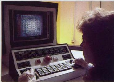
An IBM-designed closed circuit television system enables the operator to carefully align the chips before they are bonded to the ceramic substrate.
