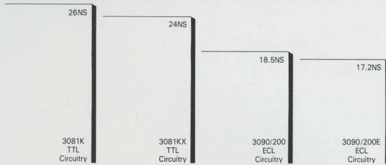
A steady progression of technology and design enhancements have allowed the machine cycle times on IBM large processors to continue to improve.
