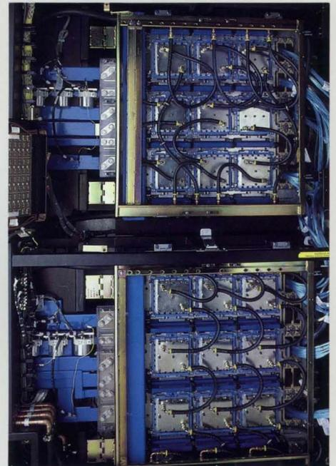
The central processor board in the triadic (300E) configuration is located above the Vector Facility board. Nine Thermal Conduction Modules (TCMs) make up each IBM 3090 Vector Facility board. Three TCMs are required for each Facility, and three Facilities are accommodated on each TCM board.
