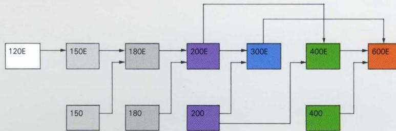
IBM 3090 upgrade options allow up to ten-fold growth in processor power.
