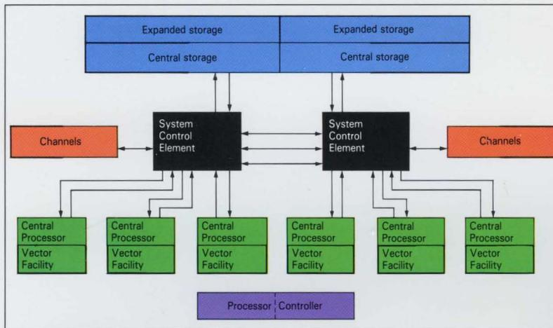
This diagram of the IBM 3090 Model 600E conceptual design shows the dynamic interaction between a System Control Element (SCE) that connects up to three central processors (with optional Vector Facilities), the channel subsystem, the processor storage, and the other side of a six-way complex. The SCE is the heart of the 3090 system since it manages the flow of information between all the elements of the processor complex.
