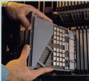
Dense four megabyte memory cards in the IBM 3090 feature fast, reliable IBM-designed and manufactured one-million-bit chips.
