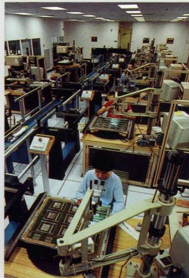
TCM boards are delivered and transferred automatically to work stations by the car-on-track conveyor system for greater operator safety and efficiency.
