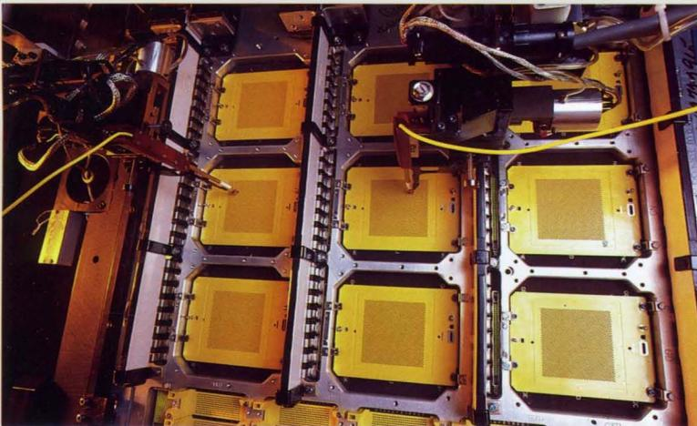
IBM robotic systems are widely used in production and testing of the 3090 TCM boards.
