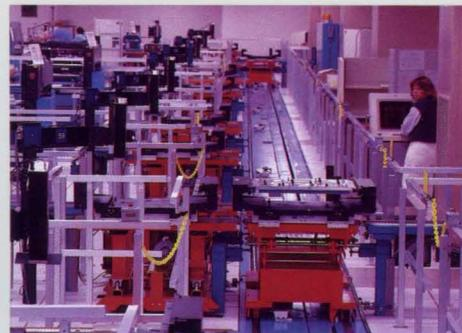
Parts move to people in the board assembly area on specially-built transport systems.
