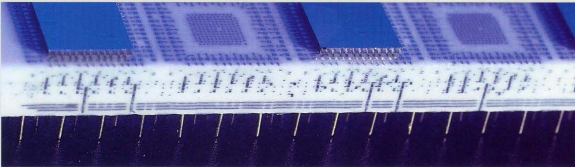
Multiple layers of buried wiring are revealed in this cutaway view of the substrate. The wires interconnect the chips soldered onto the surface using the special IBM-developed C4 process, resulting in high inter-connection reliability and density.
