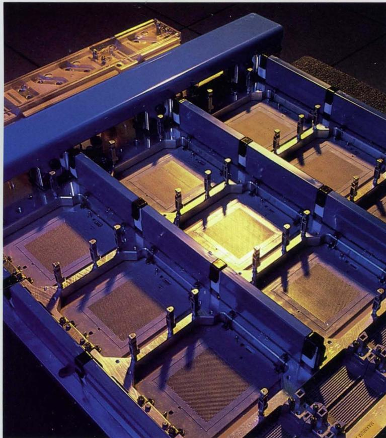
TCMs are mounted on a specially-developed 22-layer circuit board. The multilayer design incorporates over 1500 meters (nearly 5000 feet) of wire needed to provide the large number of interconnections that make up the processor complex.
