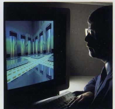
An IBM designer uses an IBM 5080 display to view a specially-developed three-dimensional model closeup of a cutaway Thermal Conduction Module (TCM). Extensive design using sophisticated imaging techniques results in highly reliable packaging for the IBM 3090.
