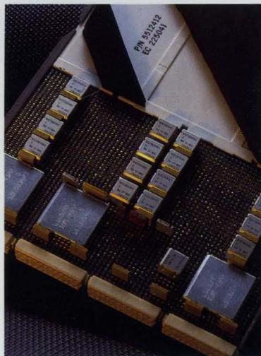
Two megabytes of memory are packaged on one card in the 3090 expanded storage. Each small module contains an IBM one-million-bit memory chip.
