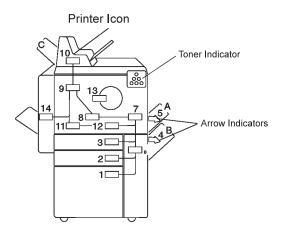
The left side of the operator panel contains a printer icon in a configuration that closely matches that of your model printer. The intervention indicator lights within the printer icon show the locations of paper jams, the locations of doors or covers to open when a paper jam occurs, and toner low conditions.
