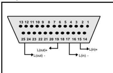
RS-422 Host/Printer Port 1 Pin Assignments
