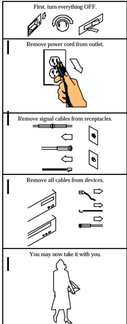
Note: In the UK, by law, the power cord must be disconnected after the telephone line cable.
