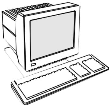
This terminal can emulate a number of ASCII and ANSI terminals, including IBM 3151, PC-Term and SCO™ Console. The keyboards supported by the terminal are the 101-key extended PC (EPC), the 106-key PC+, and the ANSI keyboards. The dual host capability of the terminal allows you to run two different applications simultaneously. A Setup option is available to view each “session” on the screen in a split or full screen display.
