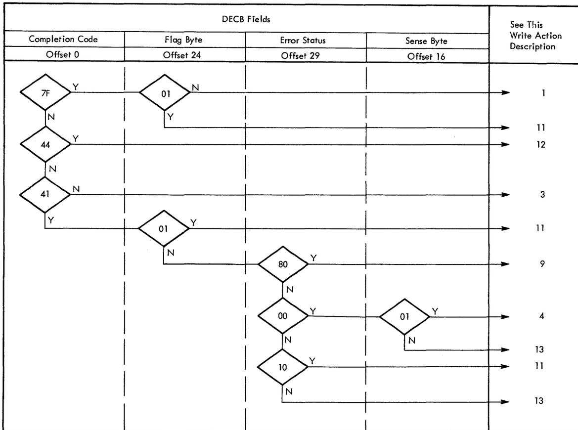
Figure 60. OS, OS/VS, BTAM Local Write Completion Analysis
