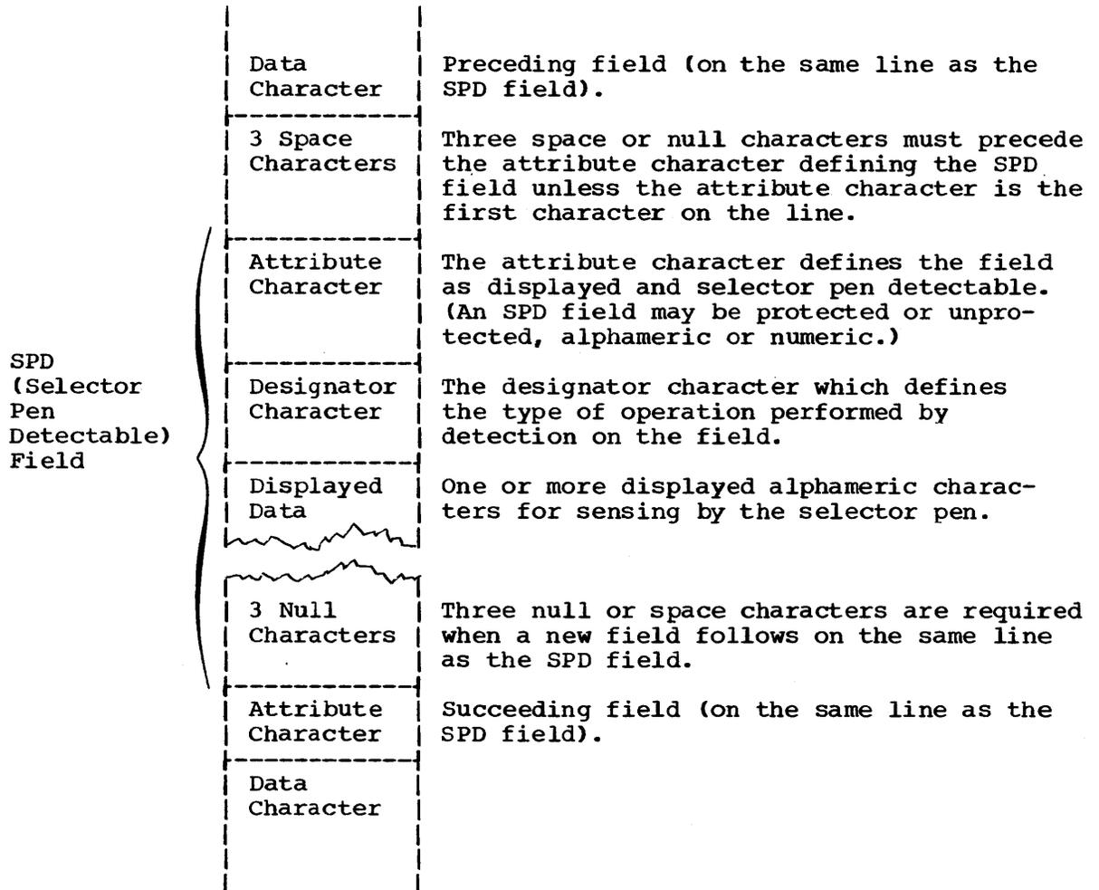
Figure 30. Definition of Field for Selector Pen Operation
