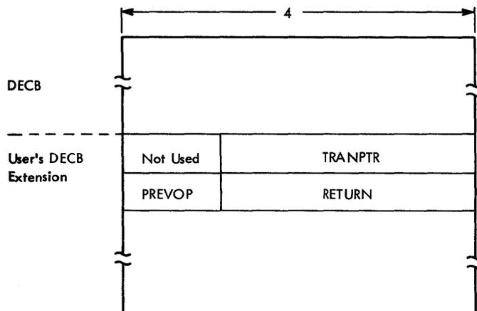
Figure 48. Example of a User-Built DECB Extension
