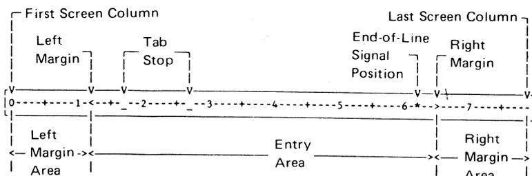
Figure 2. Entry Assist Scale Line
