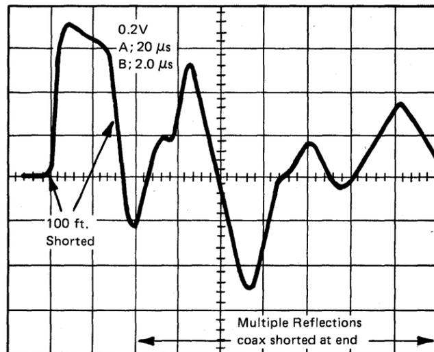
Improper setup of scope
