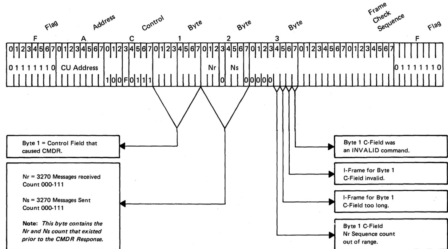
Figure 5-54. Command Reject (CMDR) Message Format
