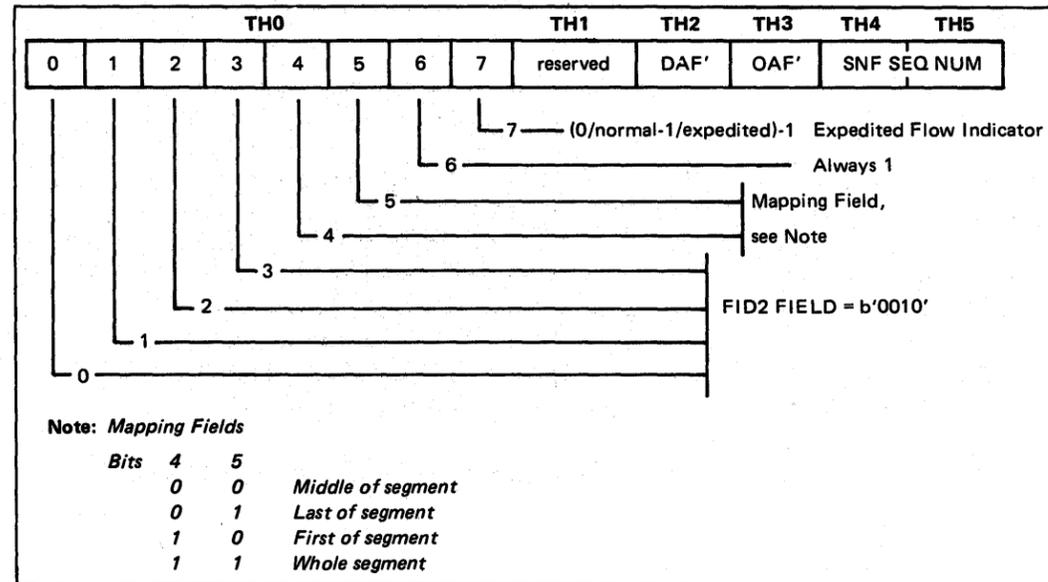
Figure 5-49. Transmission Header Format
