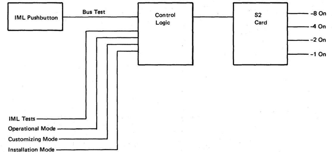
Figure 2-1. 8 4 2 1 Indicator Control Logic
