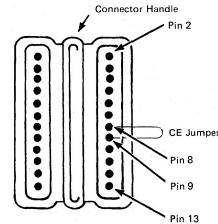
Figure 5-15. 3279 Top-Card Connector CE Jumper
