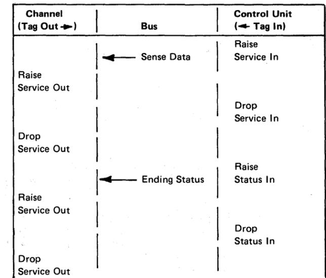
Figure 5-23. Sense—After Selection with Sense Command (Issued in Response to Unit Check Status)
