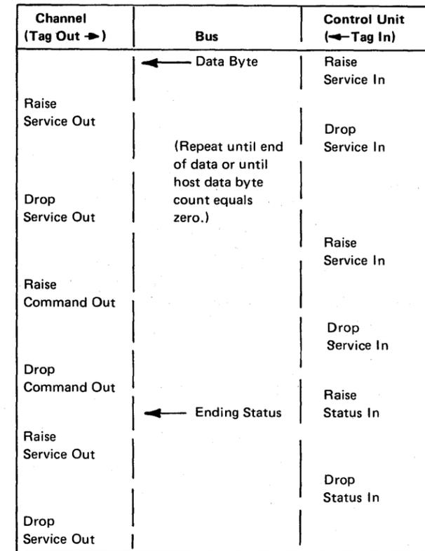
Figure 5-22. Read—After Selection with Read Command
