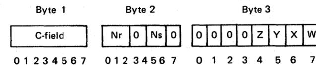
Byte 1 is the C-field that caused the CMDR response. Byte 2 contains the Ns and Nr sequence counts that existed immediately prior to establishing the CMDR response. Byte 3 indicates the reason for the CMDR.
