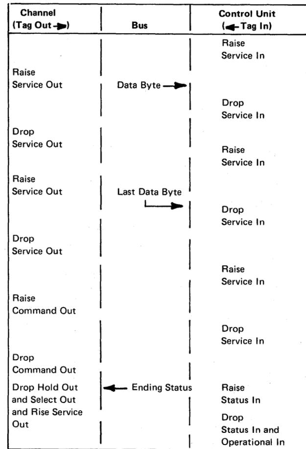
Figure 5-21. Write—After Selection with Write Command
