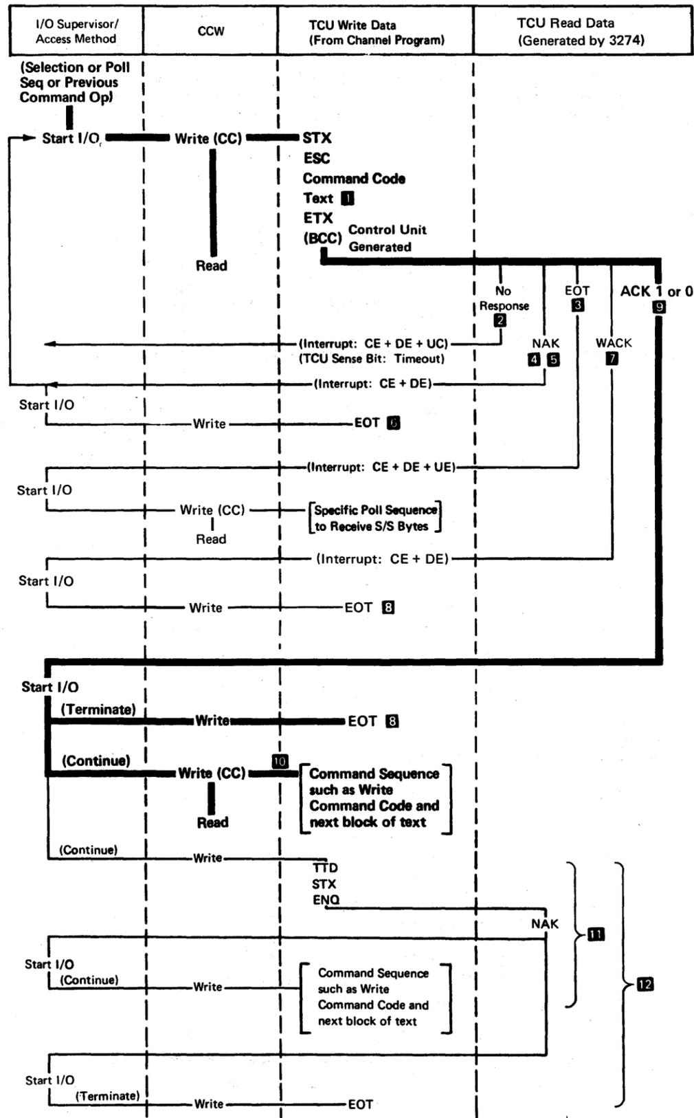
Figure 5-32. Write-Type and Control-Type Commands, Sequence/Response Diagram
