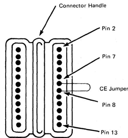
Figure 5-13. 3278 Top-Card Connector CE Jumper (Three Base Cards)
