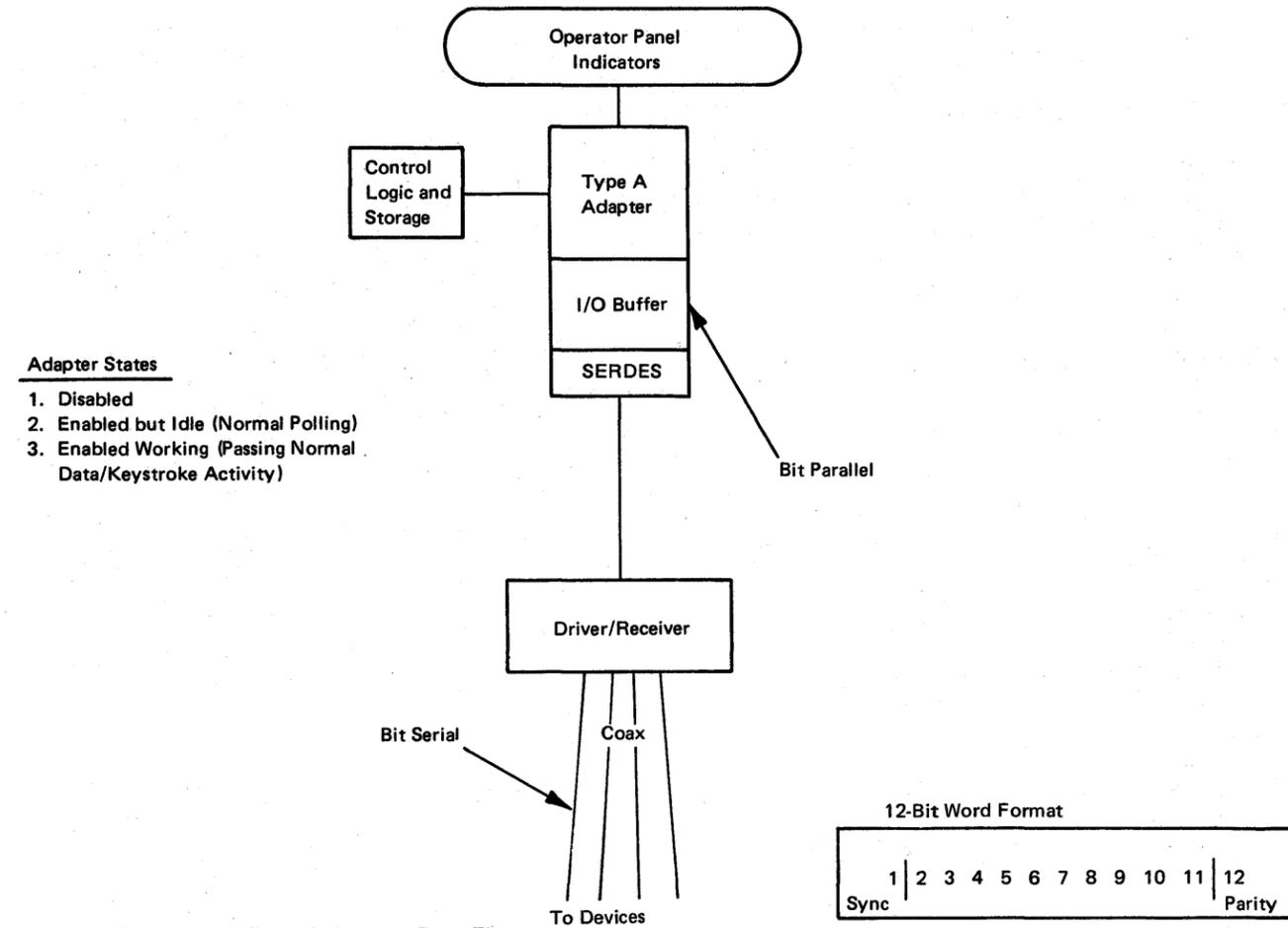
**Figure 1-13. Coax to Type A Adapter Data Flow**
