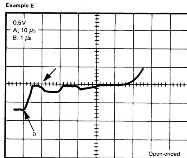
This 2400-ft cable has a 100-ohm short to shield at the 400-ft point (see arrow).
