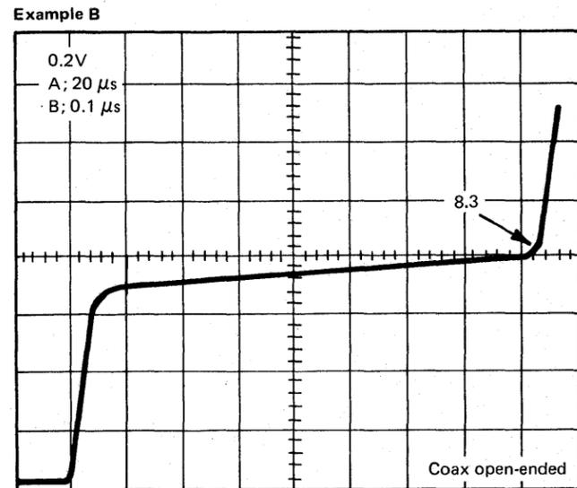
101 m (332 ft) of good coax cable, 8.3 divisions long. (This is an effective method to measure the length of the cable.)
