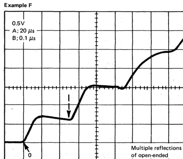
Improper setup of scope.
