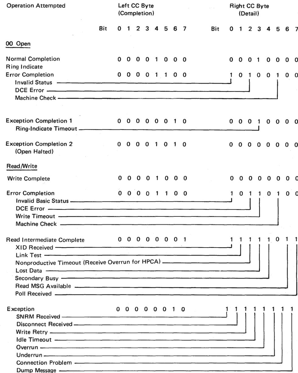
Figure 3-6. CCA/HPCA SDLC Operation Ending Chart (Code CCCC)
