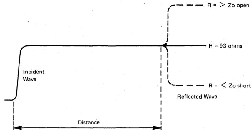
Figure 4-19. Incident and Reflected Waves
