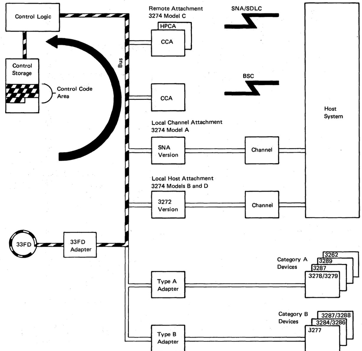
Figure 1-3. Initial Machine Load Data Flow
