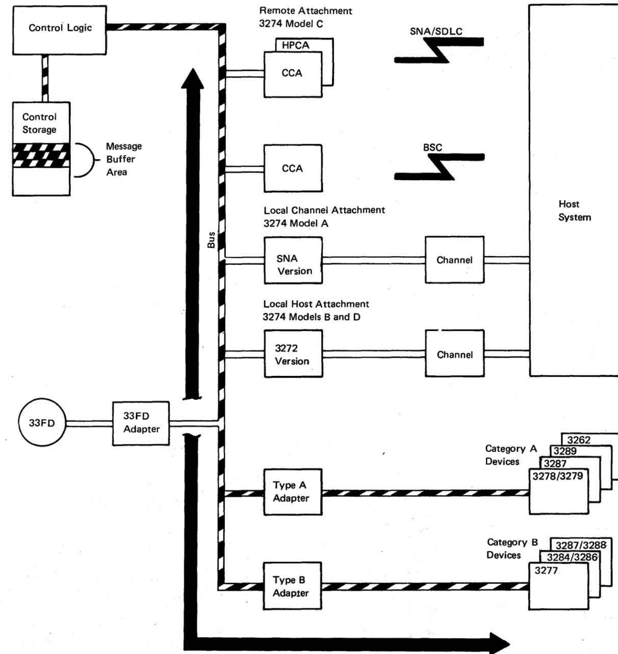
Figure 1-4. Message Data Flow between 3274 Control Unit and Devices
