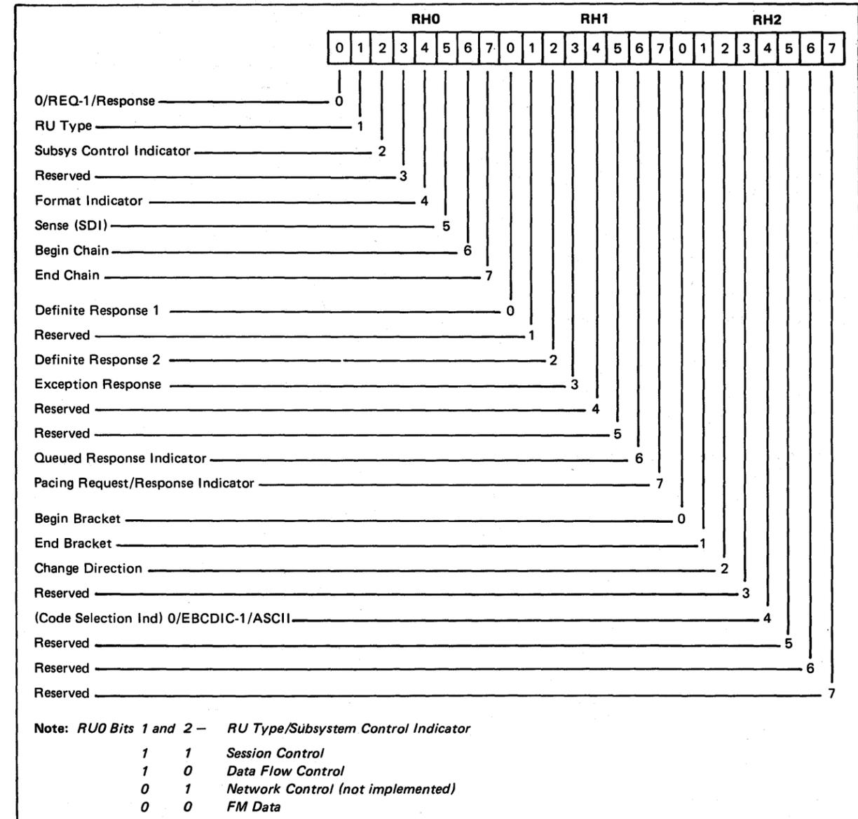
Figure 5-50. Request/Response Header Format
