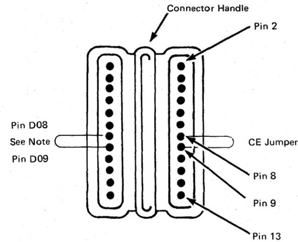
Figure 5-14. 3278 Top-Card Connector CE Jumper (Two Base Cards)
