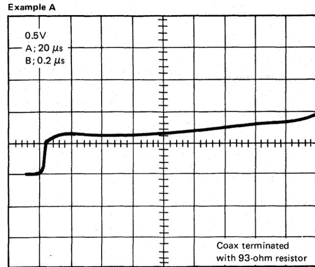
This is an illustration of a good, no-fault coax cable that is 190 m (624 ft.) long. A gradual sloping and overshoot of rise time is normal.
