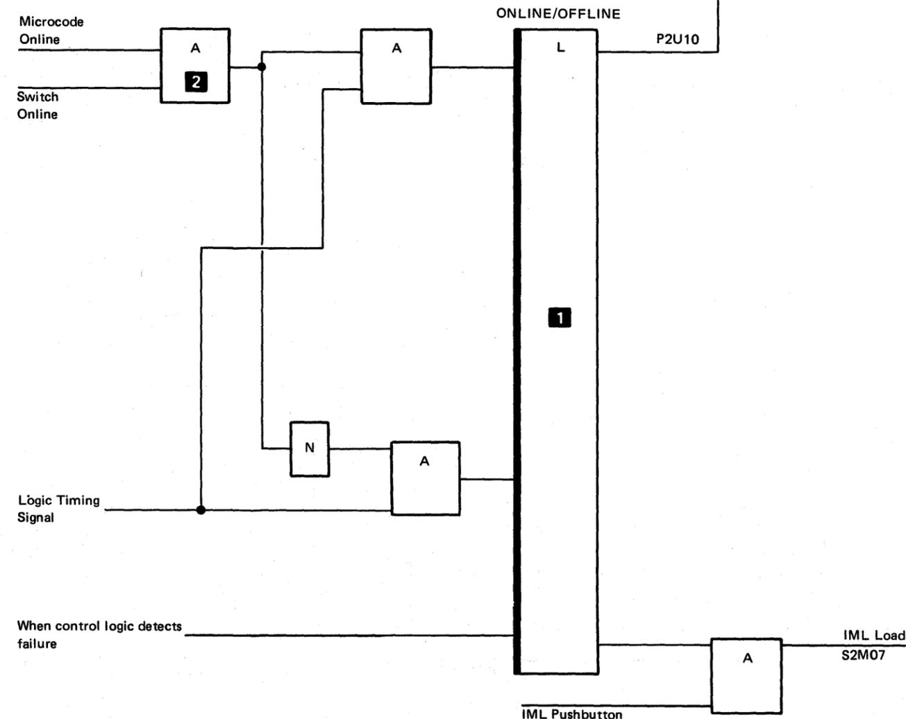
Figure 2-3. ONLINE/OFFLINE Control Logic, Models B and D
