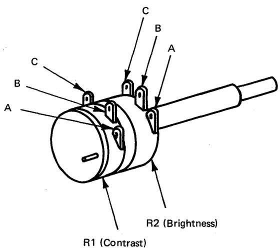
Diagram 7-13. Brightness and Contrast Control Terminals
