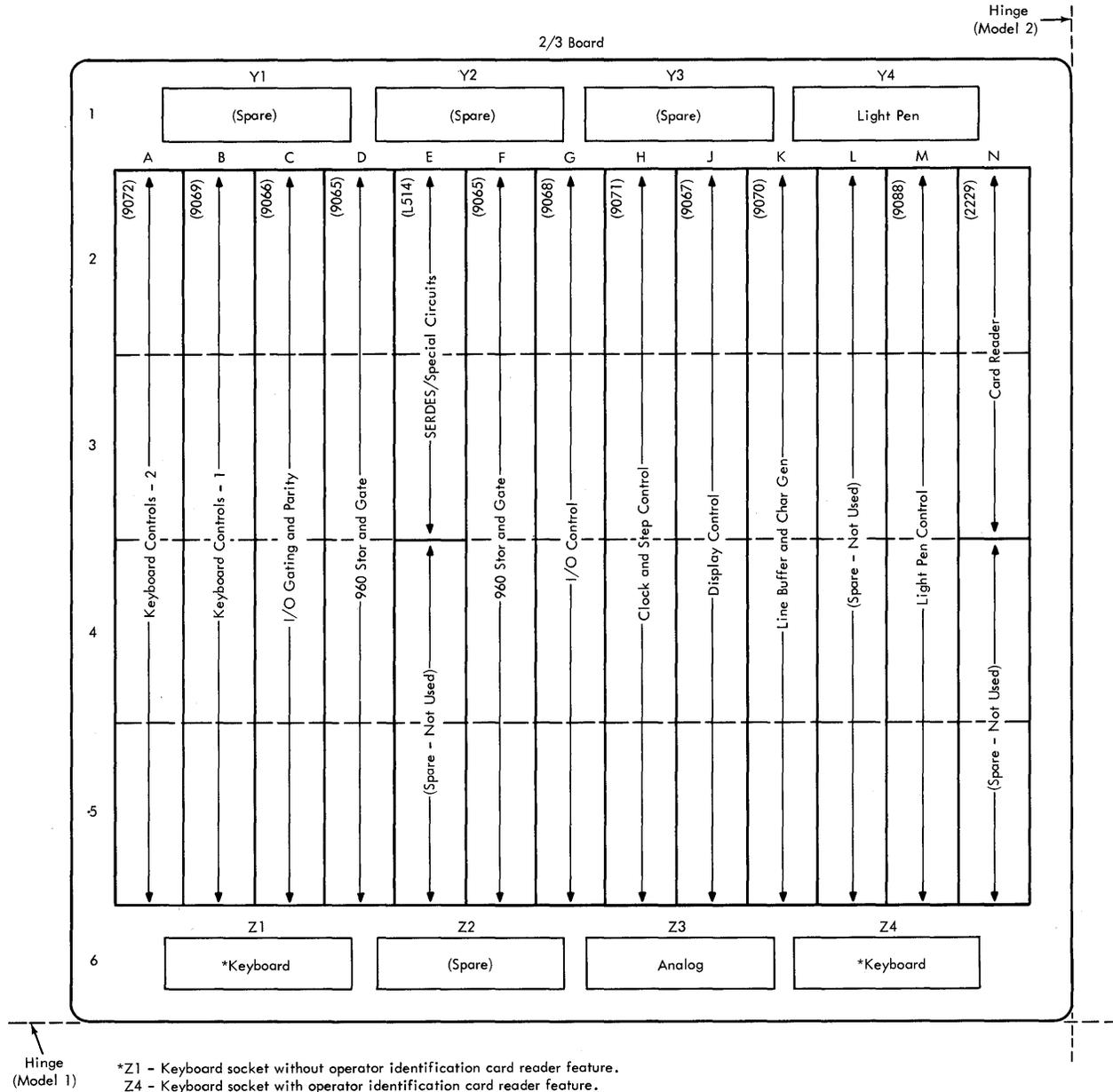
**Diagram 6-13. Board Layout by Card Function - With Features (Card Side View)**
