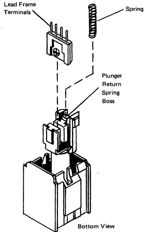
**Diagram 5-4. Switch Plunger Return Spring Positioning**
