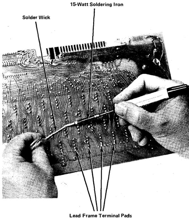
**Diagram 5-2. Unsoldering Lead Frame Terminals**
