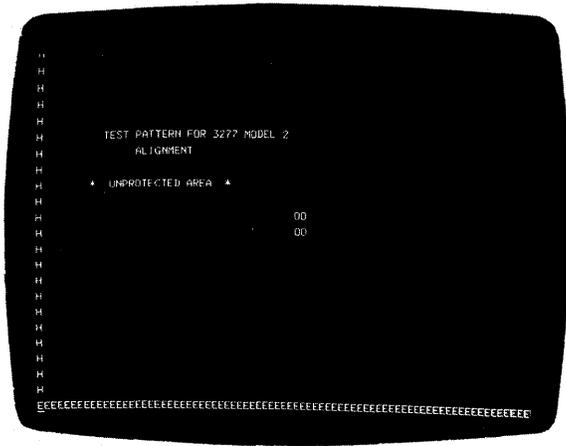
Diagram 3-7. Centering Rings Not Adjusted Properly
