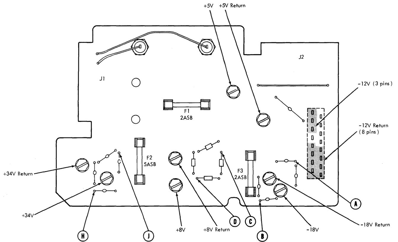
**Diagram 7-9. Low-Voltage Printed Circuit Board**
