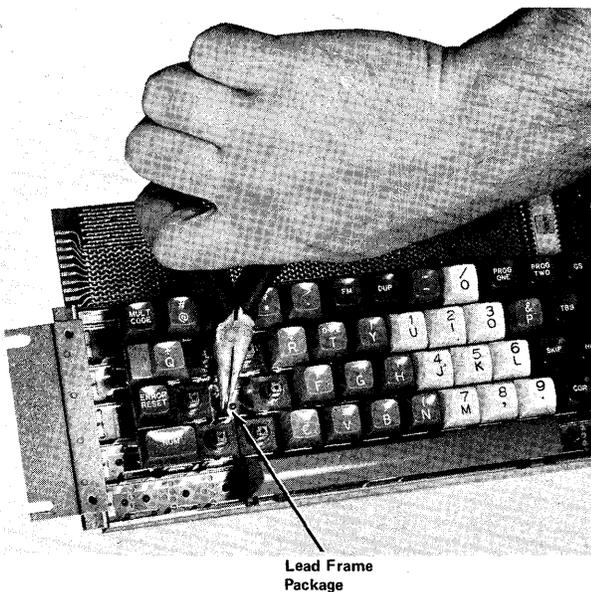
**Diagram 5-3. Lead Frame Removal**
