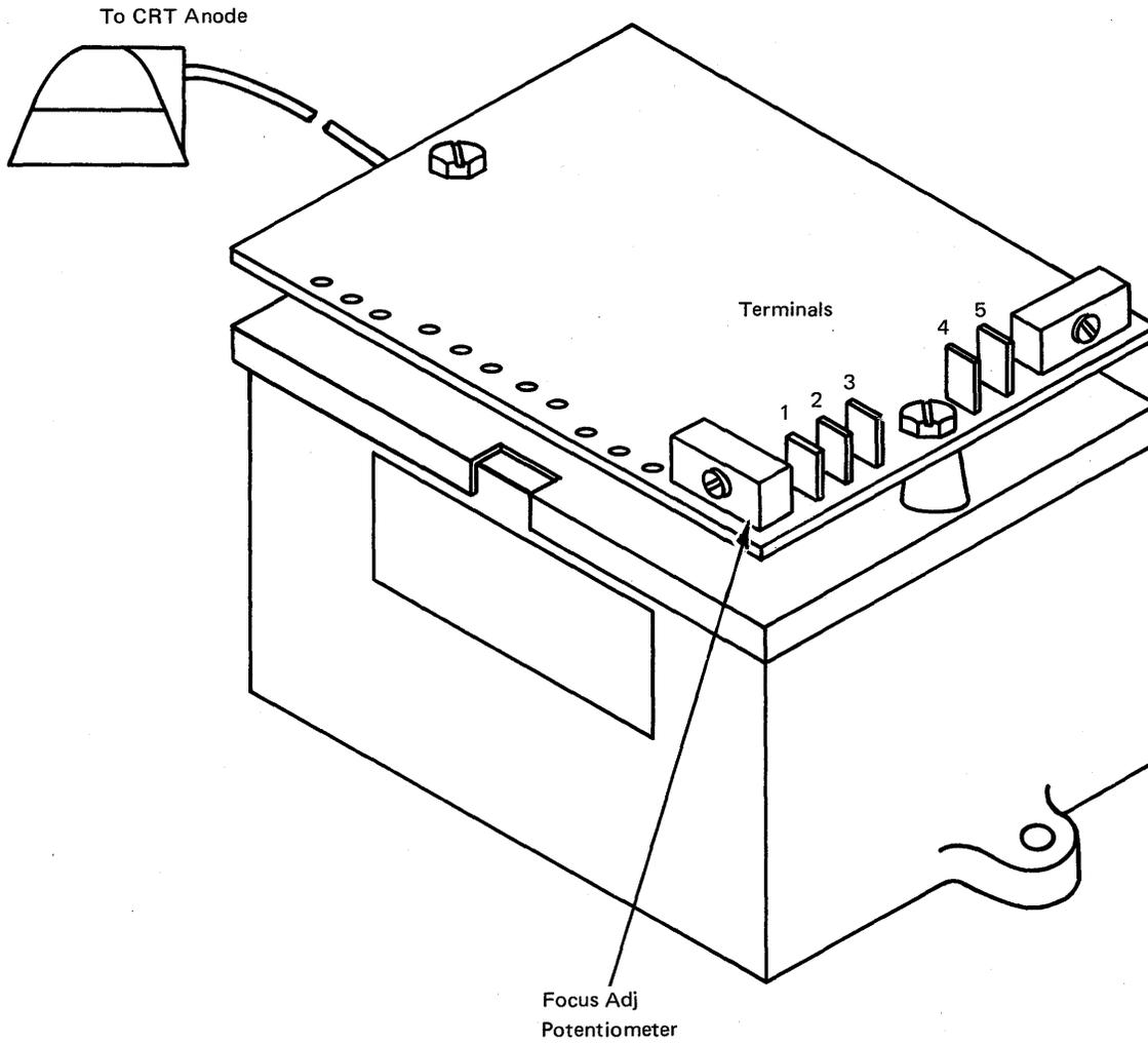
**Diagram 7-14. High-Voltage Power Supply**
