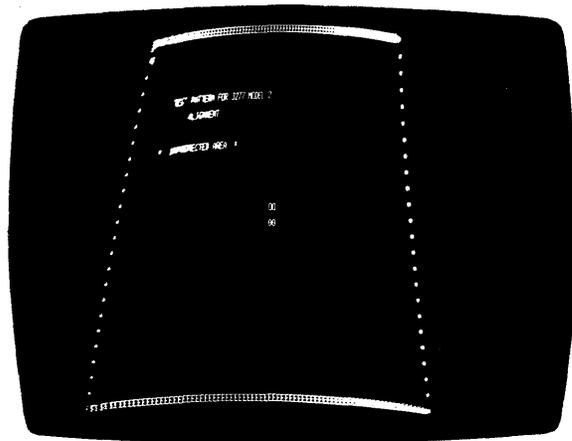
Diagram 3-20. Open in Yoke Horizontal Winding
