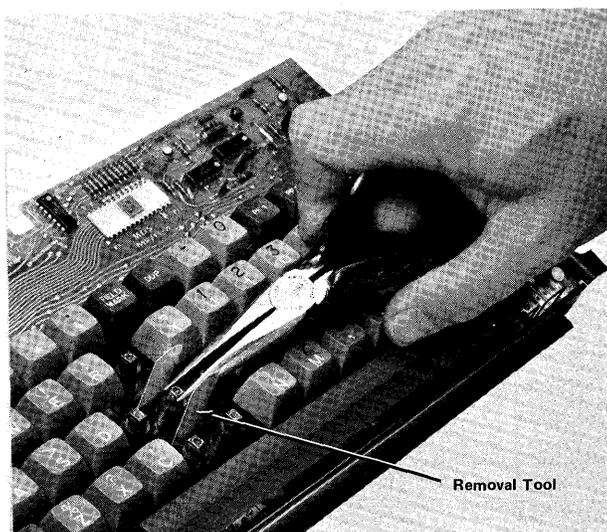
Diagram 5-1. Switch Module Removal
