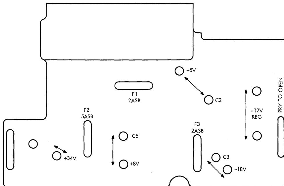
**Diagram 7-10. Low-Voltage Printed Circuit Board Shield**
