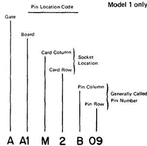
Diagram 6-14. Board Layout Pin Identification Data (Pin Side View)
