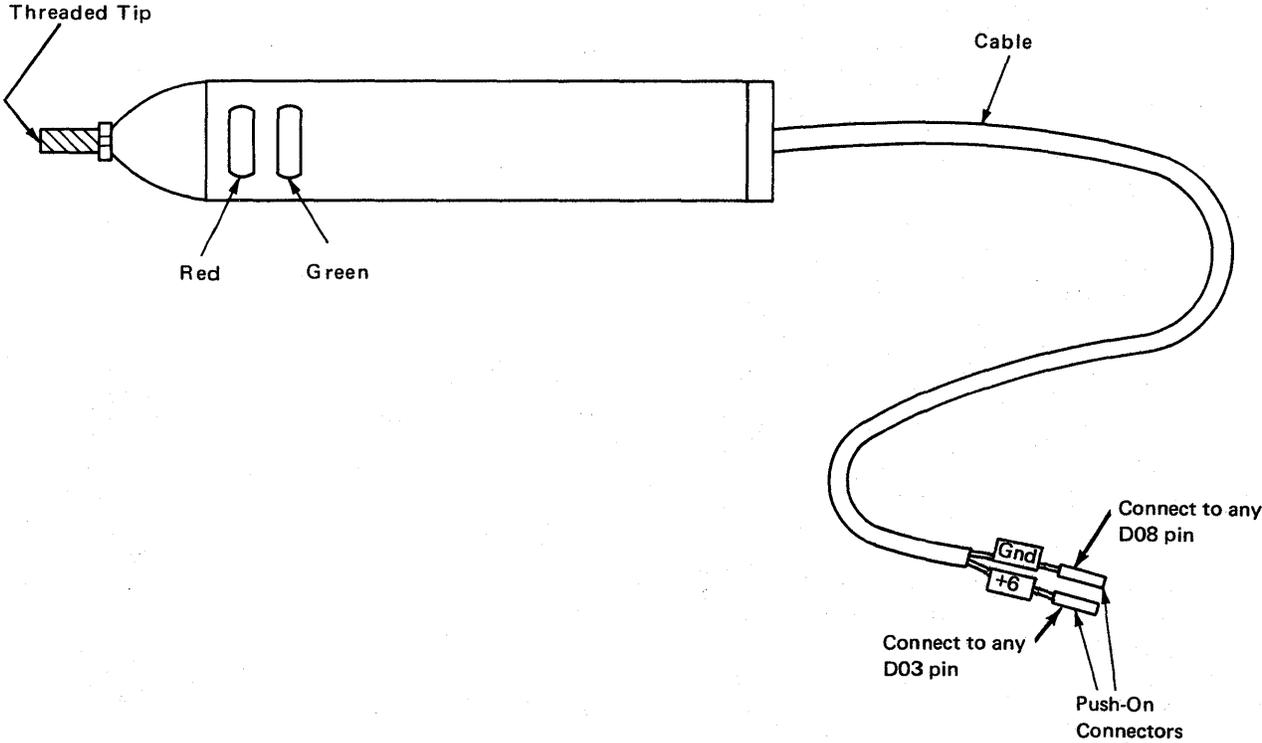
Diagram 2-1. Logic Probe
