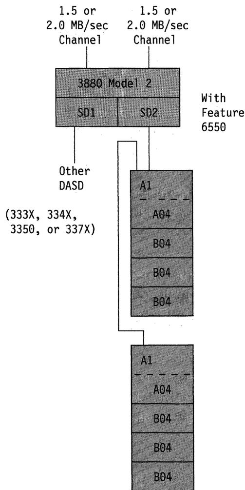
Figure 18. Example of 3380 Model A04 Strings Attached to a 3880 Model 2
