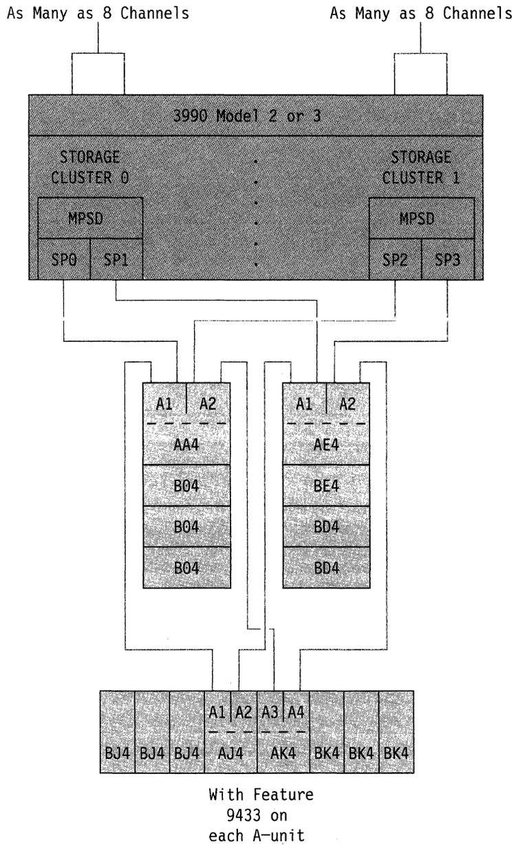
Figure 34. Example of 3380 2-Path and 4-Path Strings Attached to a 3990 Model 2 or 3
