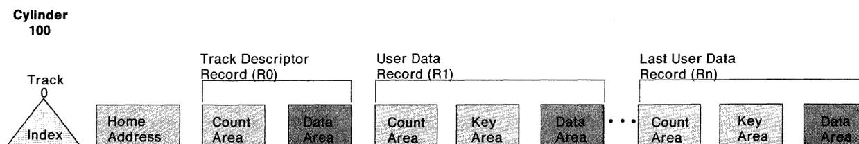
Figure 11. Track and Record Format, Simplified Representation
