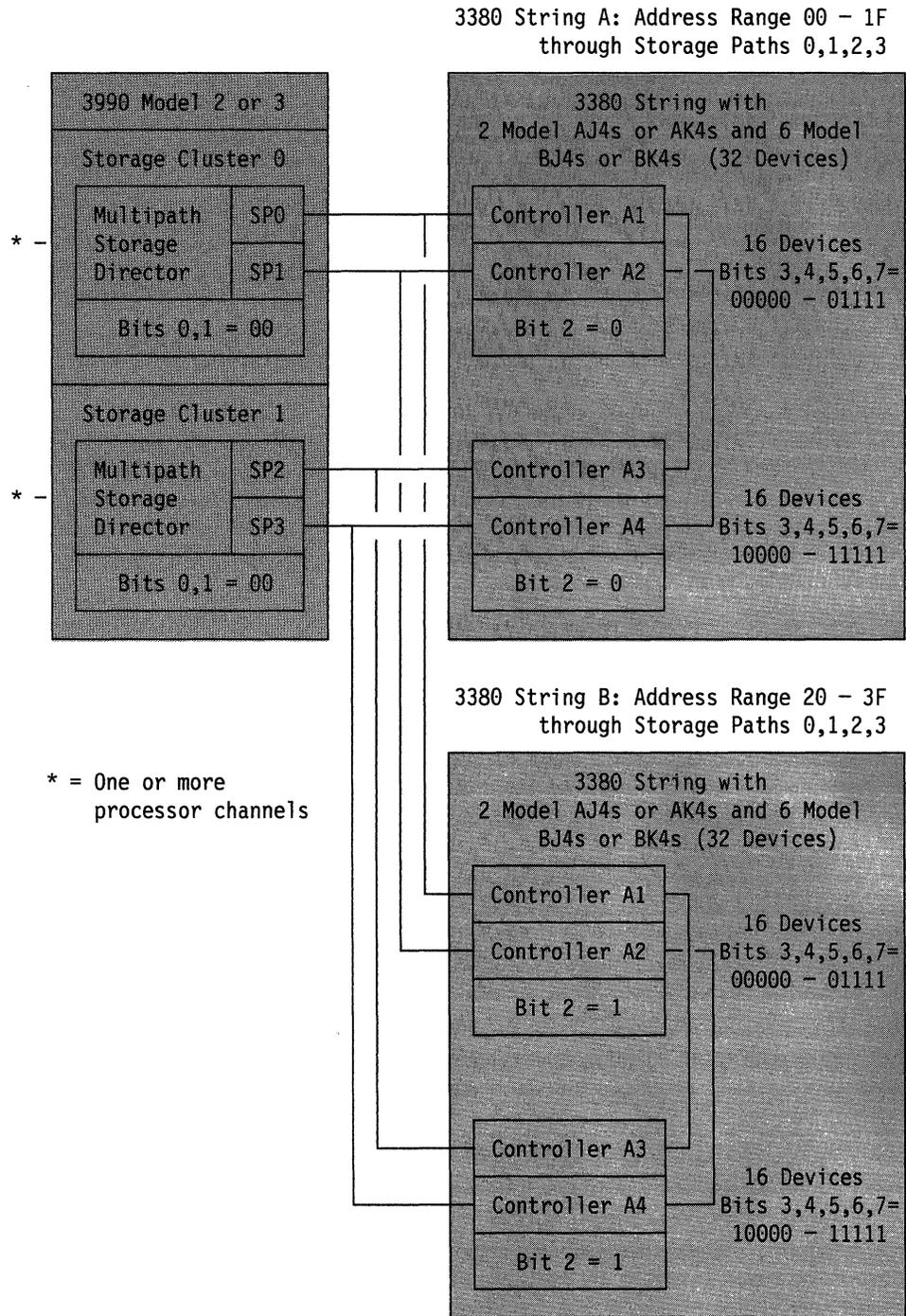
Figure 54. Addressing Example. Two 3380 4-Path Strings (64 Devices) Attached to Two 3880 Storage Directors
