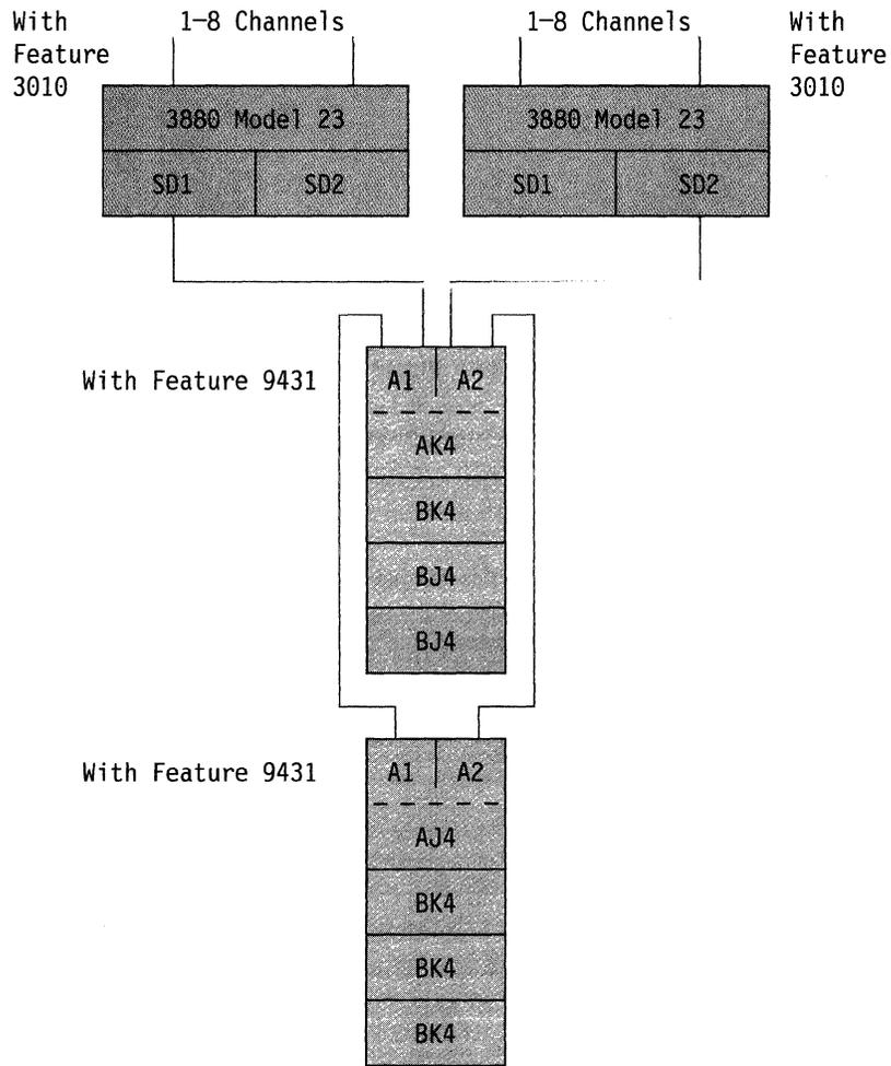
Figure 25. Example of 3380 Model AJ4 and AK4 2-Path Strings Attached to Dual-Framed 3880 Model 23s
