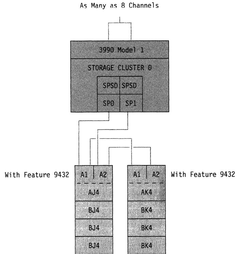
Figure 31. Example of 3380 Model AJ4 and AK4 2-Path Strings Attached to a 3990 Model 1
