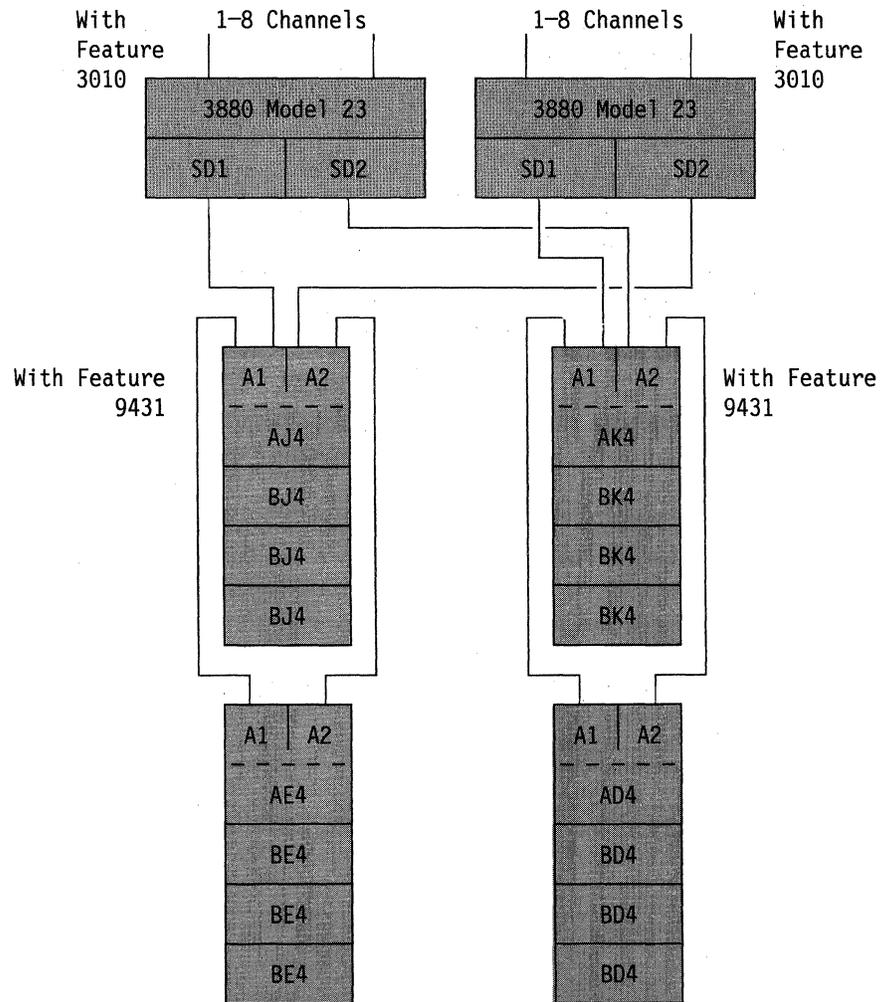
Figure 26. Example of Intermixed AD4, AE4, AJ4, and AK4 Strings Attached to Dual-Framed 3880 Model 23s
