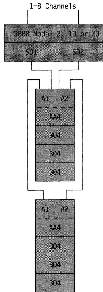
Figure 20. Example of 3380 Model AA4 Strings Attached to a 3880 Model 3, 13, or 23
