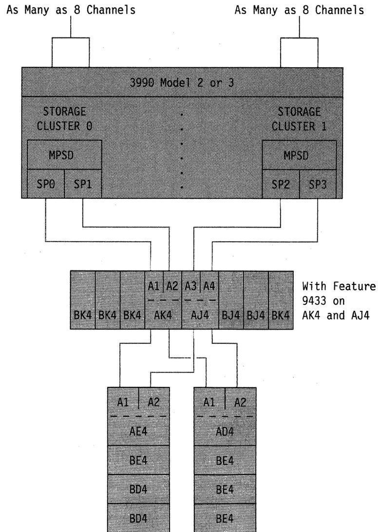
Figure 35. Example of 3380 4-Path and 2-Path Strings Attached to a 3990 Model 2 or 3
