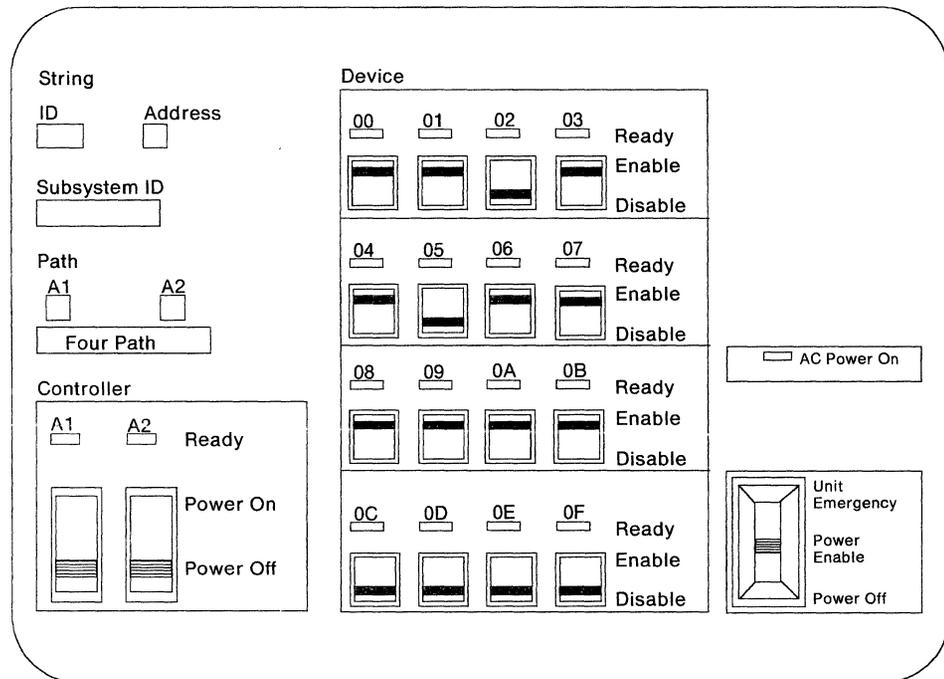
Figure 43. 3380 Model AJ4 or AK4 4-Path Operator Control Panel with Feature 9433. Used for attachment to 3990 Model 2 or 3 Storage Controls. There is a similar panel on the second A-unit that specifies controllers A3 and A4 and devices 10 through 1F.
