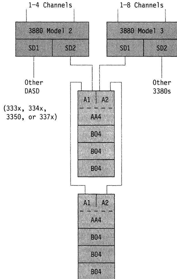
Figure 19. Example of 3380 Model AA4 Strings Attached to 3880 Model 2 and 3 Storage Directors
