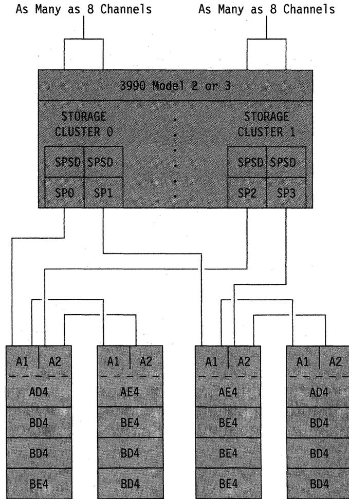
Figure 30. Example of 3380 Model AD4 and AE4 Strings Attached to a 3990 Model 2 or 3
