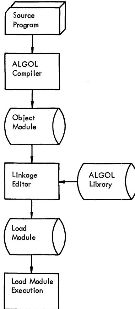
Figure 1. Basic flowchart for handling an ALGOL program.
