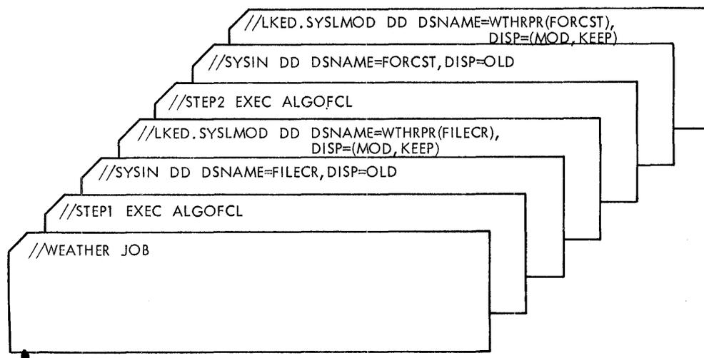
Figure 3. Sample deck for using ALGOFC cataloged procedure with two source programs. These two job steps compile and linkage edit two source programs used in Example 3 of Appendix E. Both source programs have been previously stored on intermediate I/O devices.
