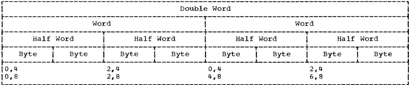
Figure 5-6. CNOP Alignment
