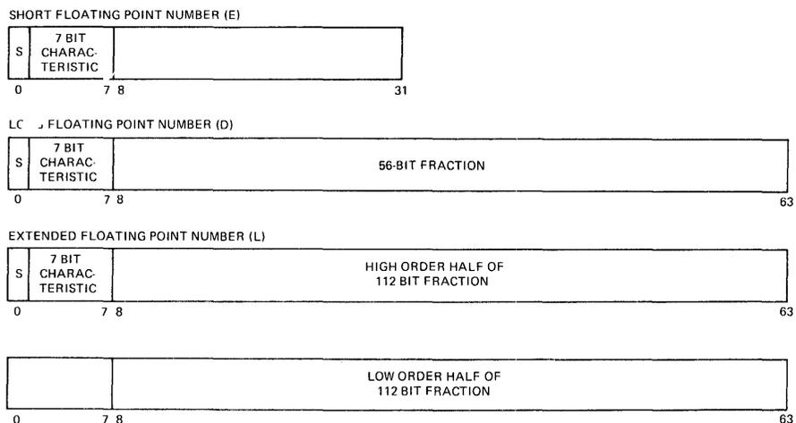
Figure 5-5. Floating-Point External Formats
