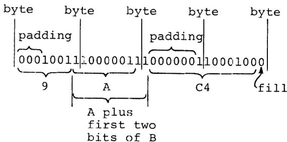
Figure 5-4. Bit-Length Specification (Multiple Operands)
