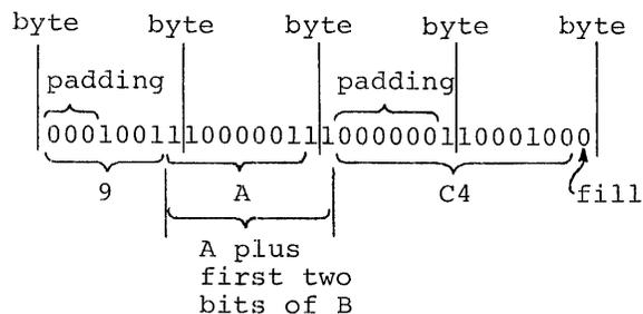
Figure 5-4. Bit-Length Specification (Multiple Operands)
