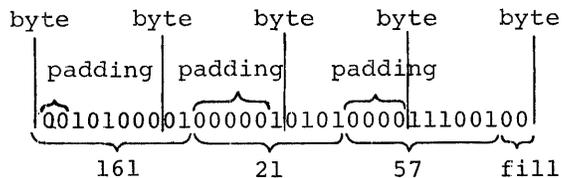
Figure 5-3. Bit-Length Specification (Multiple Constants)
