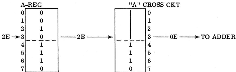
Gate low four bits of the A-register to the low four bits of the adder, block the high four bits.
