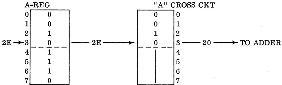
The high four bits of the A-register contents is allowed to pass to the adder, but the low four bits are blocked.
