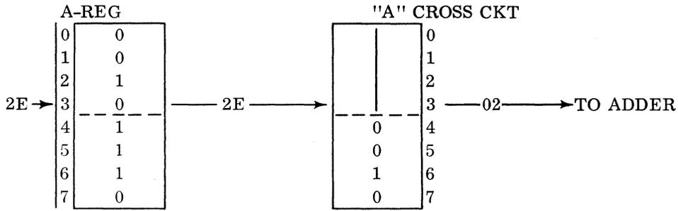
Gate the high four bits of the A-register to the low four bit input to the adder, block the high four bits.
