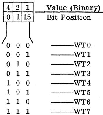
Depending on the bit positions that are active (1), seven different configurations can be represented.
