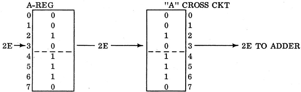
The Adder receives data exactly as it was contained in the A-register.
