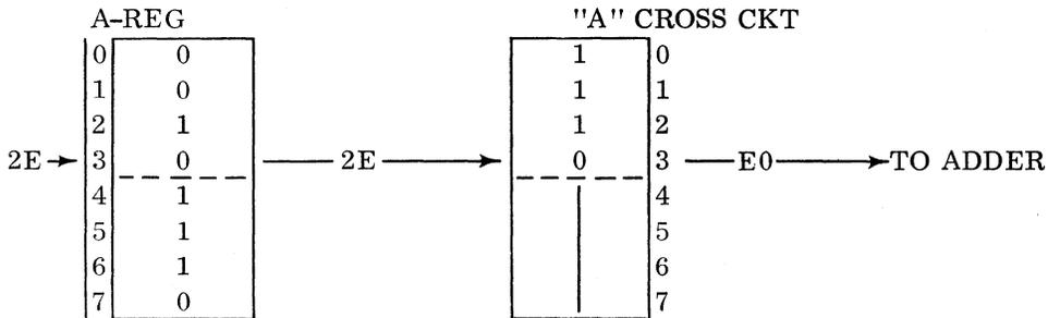
Gate the low four bits of the A-register to the high four bits of the adder, block the low four bits.
