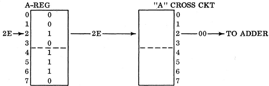
Block the A-register input to the adder.
