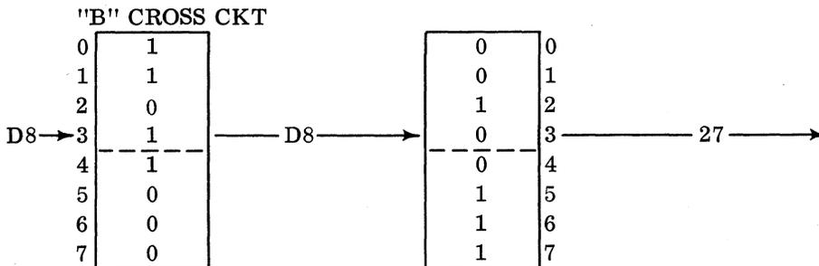
Contents of the B-register are inverted and gated to the adder.
