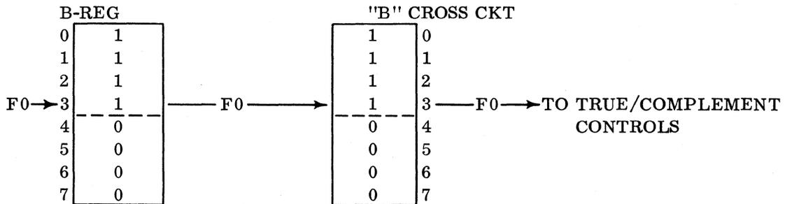
Gate bits 0-7 of the B-register to bits 0-7 of the true/complement controls.
