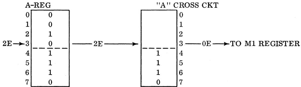
The low four bits of the A-register are gated to the M1-register for "Branch on Mask" control word operations. (Word Type 5)
