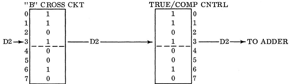
Gate B-register contents undisturbed to the adder.
