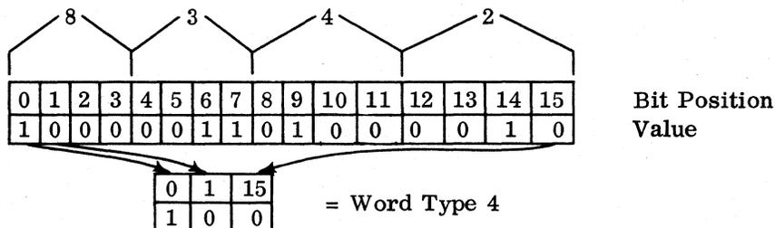
Depending on the control word read into the control register; to determine the word type, the system simply looks at three bit positions.
