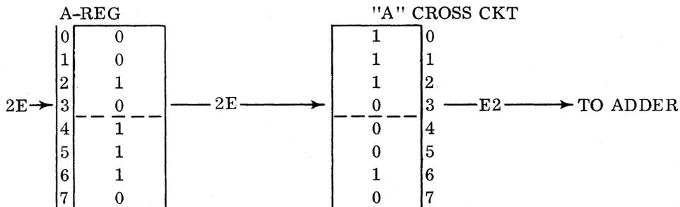
Gate the low four bits of the A-register to the high four bits of the adder, gate the high four bits of the A-register to the low four bits of the adder.
