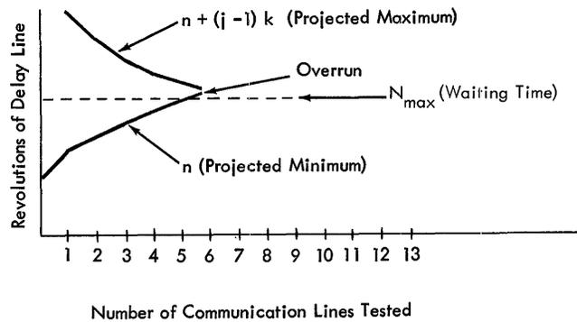
Figure 7. Projection of Delay Line Revolution
