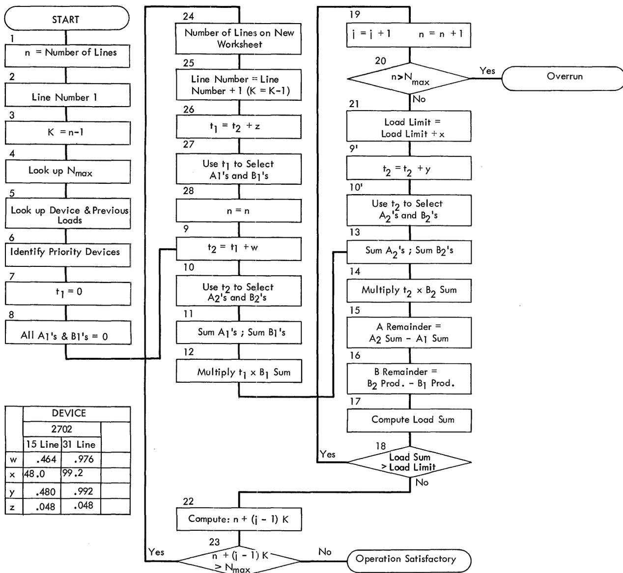
Figure 9. Flowchart for IBM 2702 Performance Analysis Worksheet
