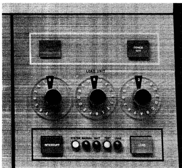
●Figure 12. Operator Controls (Areas B, F, and G)
