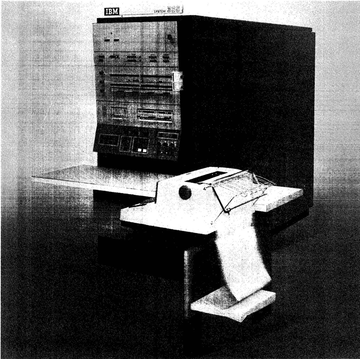
• Figure 1. Processing Unit and Console Printer-Key-board
