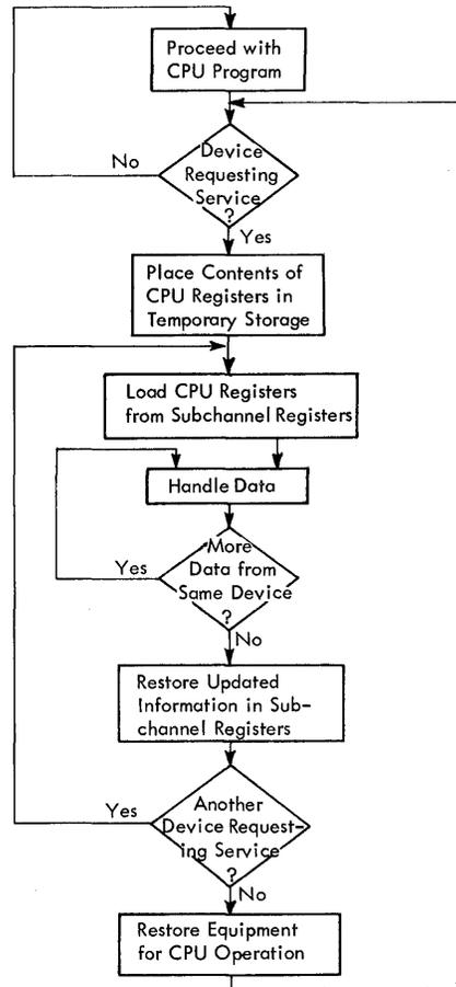
Figure 4. Equipment Sharing by Model 40 CPU and Multiplexer Channel
