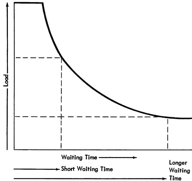
Figure 5. Priority Load Curve
