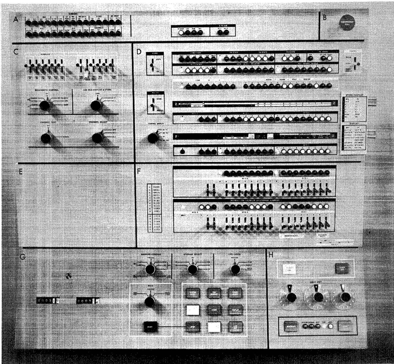
Figure 3. Model 40 System Control Panel
