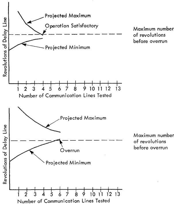
● Figure 7. Projection of Delay Line Revolution Requirements
