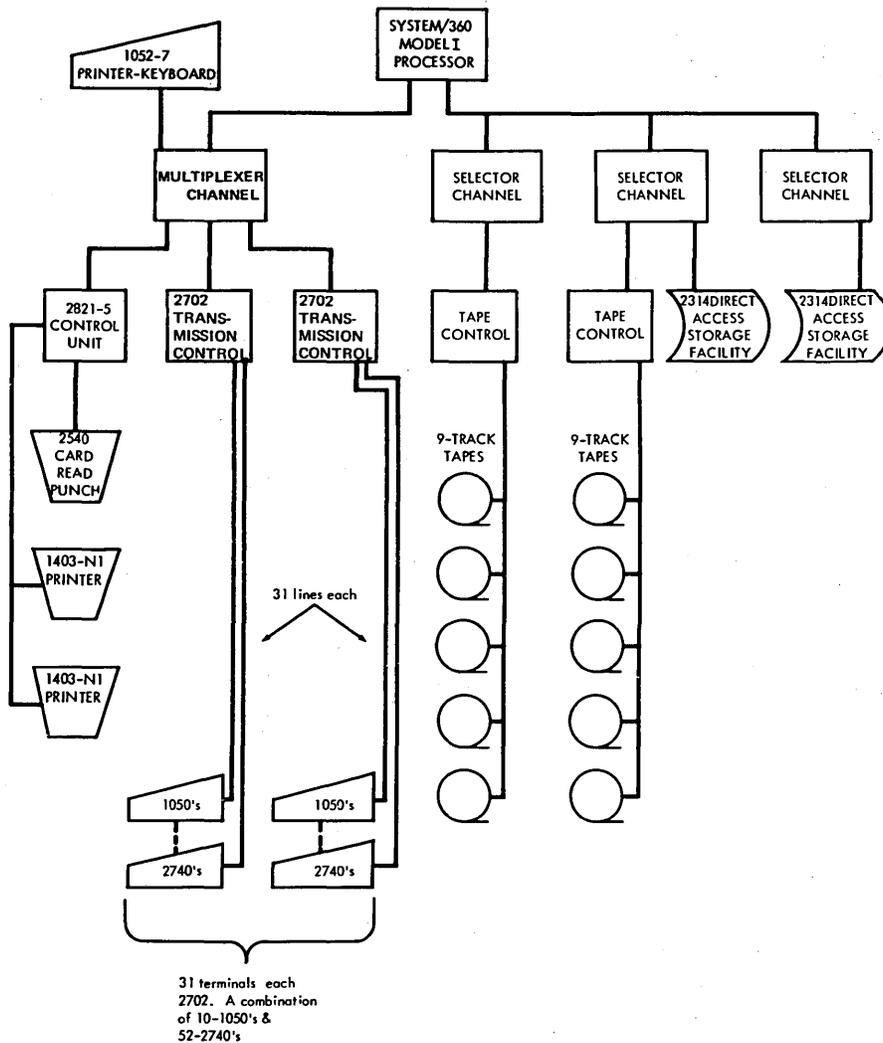
•Figure 16. Typical configuration - IMS/360 System
