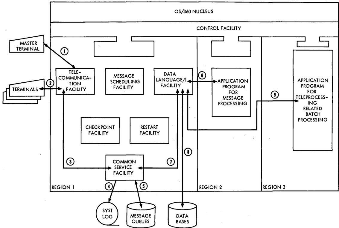
Figure 11. Teleprocessing and related batch IMS/360 system flow
