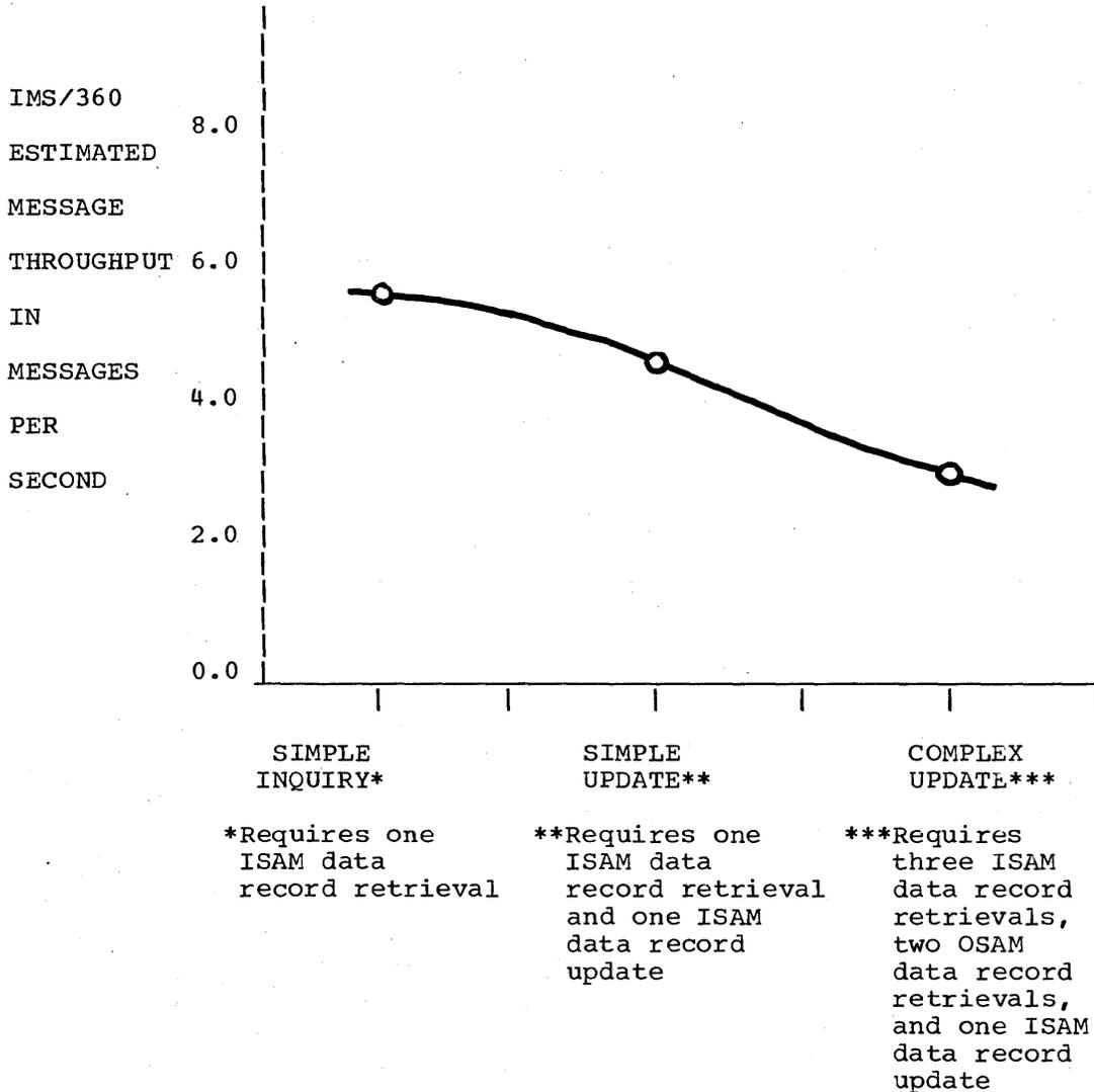
Figure 13. Large Information Management System/360 example - message throughput graph
