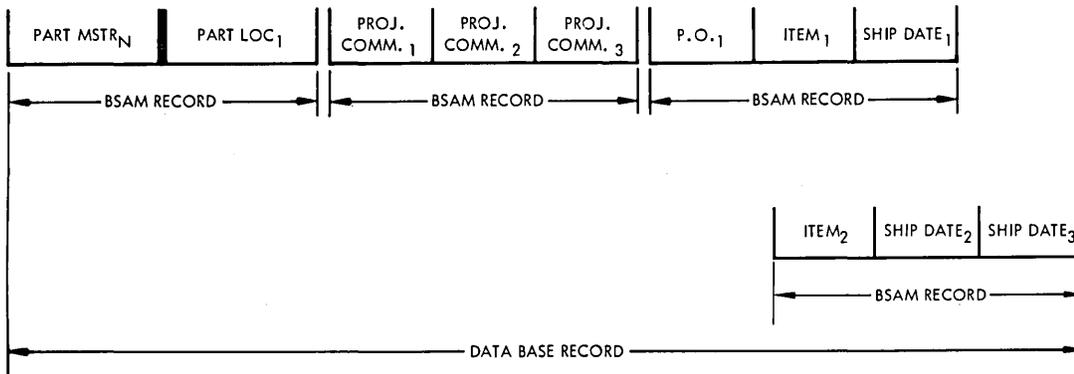
Figure 5. The Nth data base record stored in the hierarchical sequential organization
