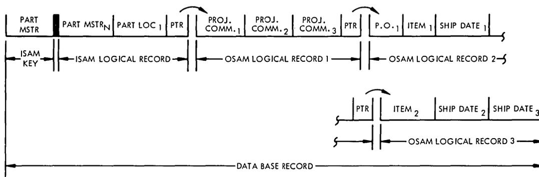
Figure 6. The Nth data base record in hierarchical indexed sequential organization
