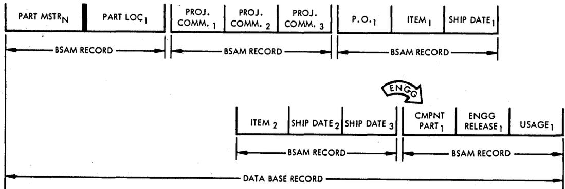
Figure 9. The Nth data base record in the hierarchical sequential organization - engineering data added
