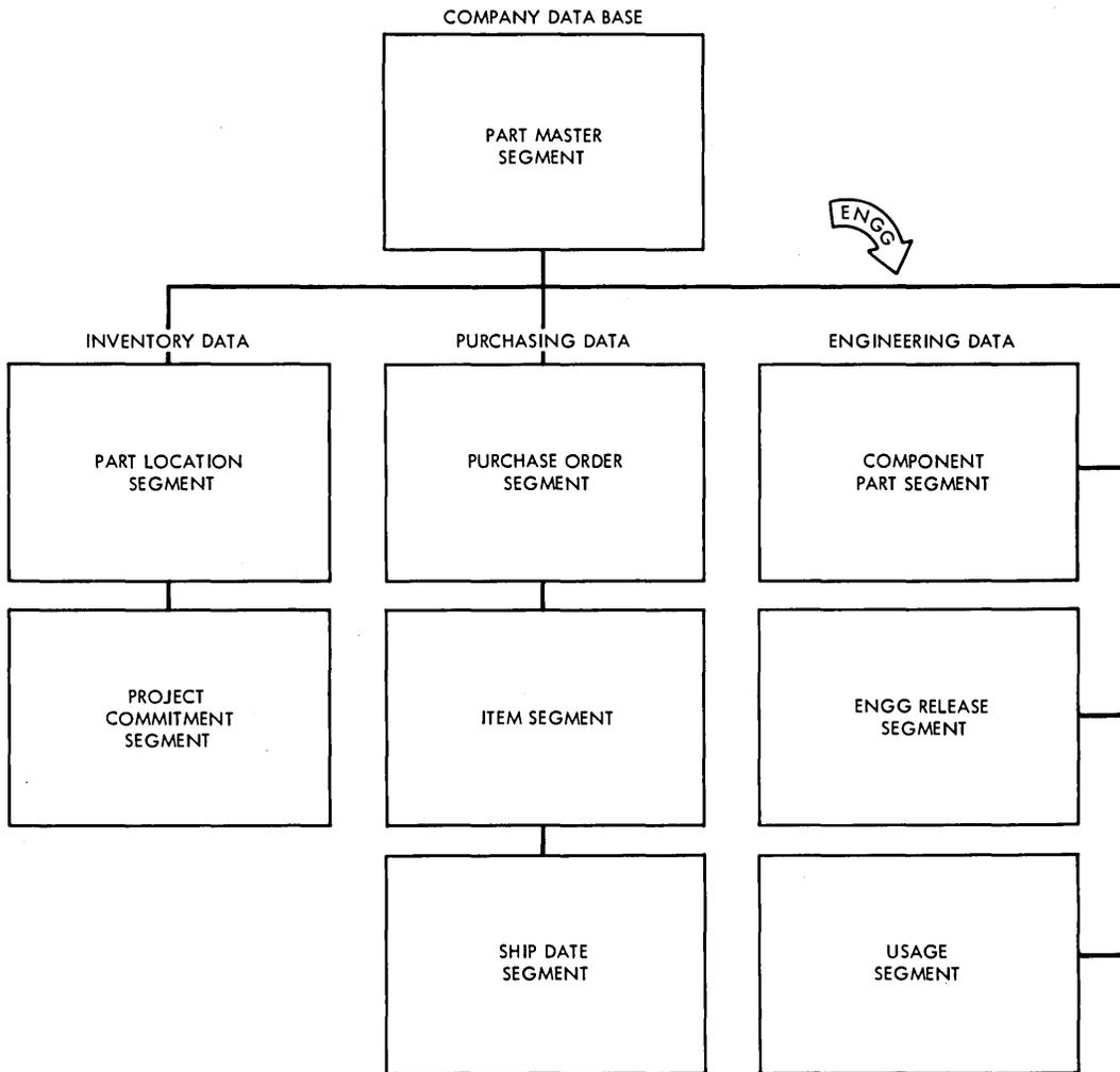
Figure 7. Company data base segment logical hierarchical relationship - inventory and purchasing data - engineering data added
