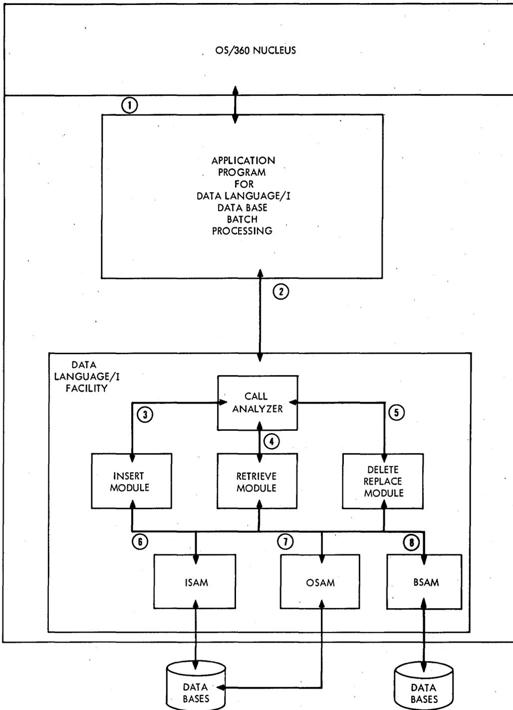
Figure 12. Data Language/I data base batch system flow
