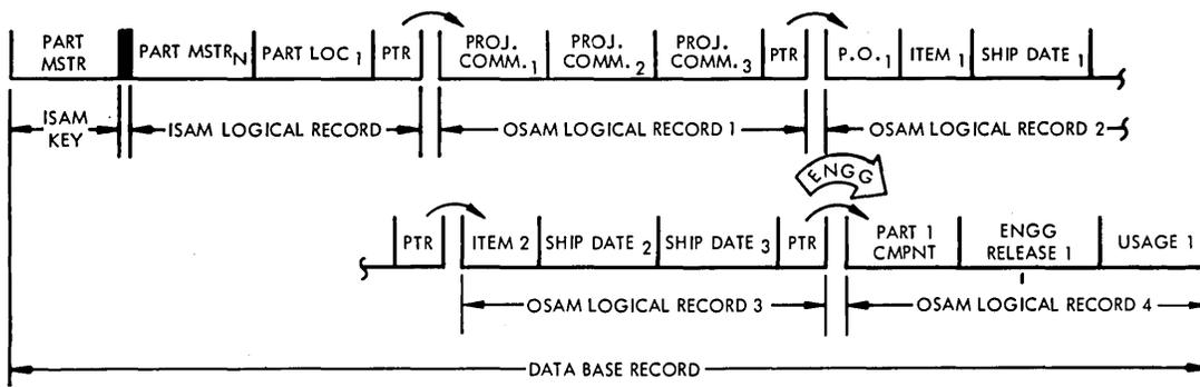
Figure 10. The Nth data base record in hierarchical indexed sequential organization - engineering data added
