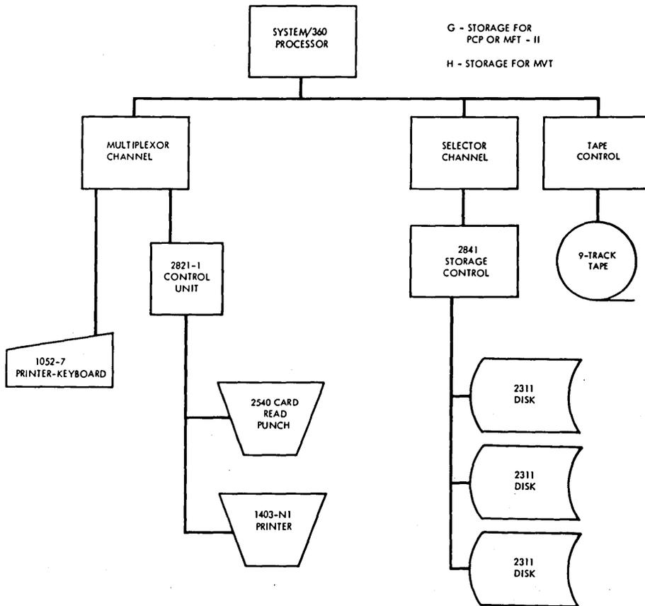
Figure 15. Minimum configuration - IMS/360 batch-only
