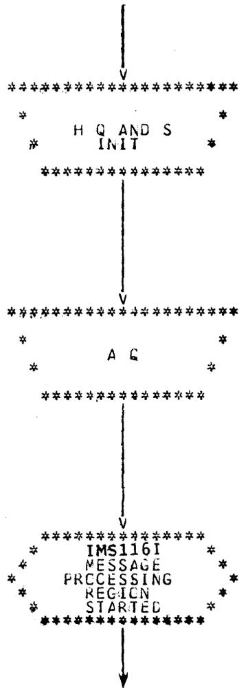
At the same time that the reply goes to the MT saying that the start message region command is in progress, two messages are received at the System/360 console.
