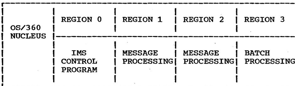
Figure 2. Operating System/360-IMS/360 multiprogramming environment
