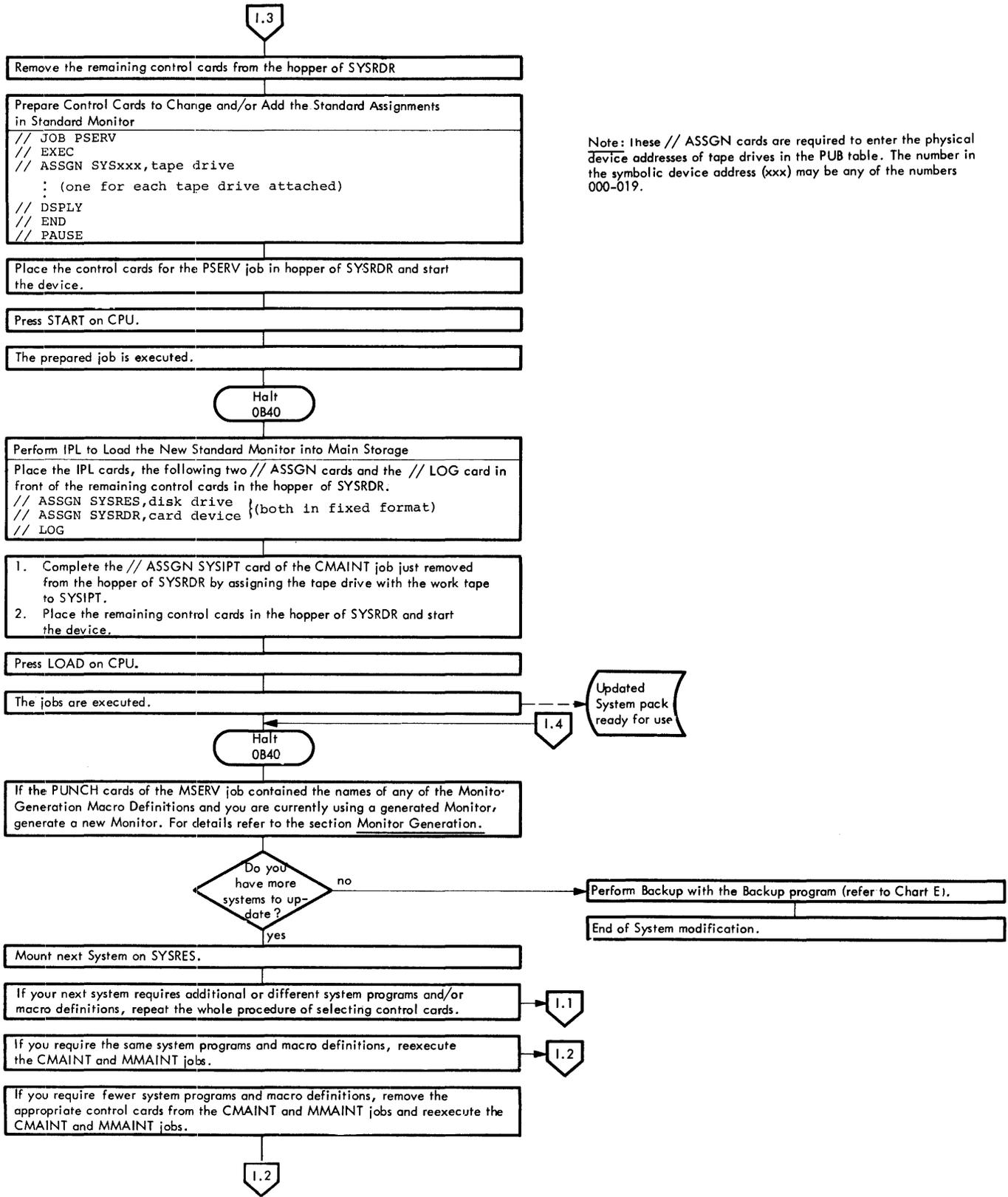
Note: These // ASSGN cards are required to enter the physical device addresses of tape drives in the PUB table. The number in the symbolic device address (xxx) may be any of the numbers 000-019.
