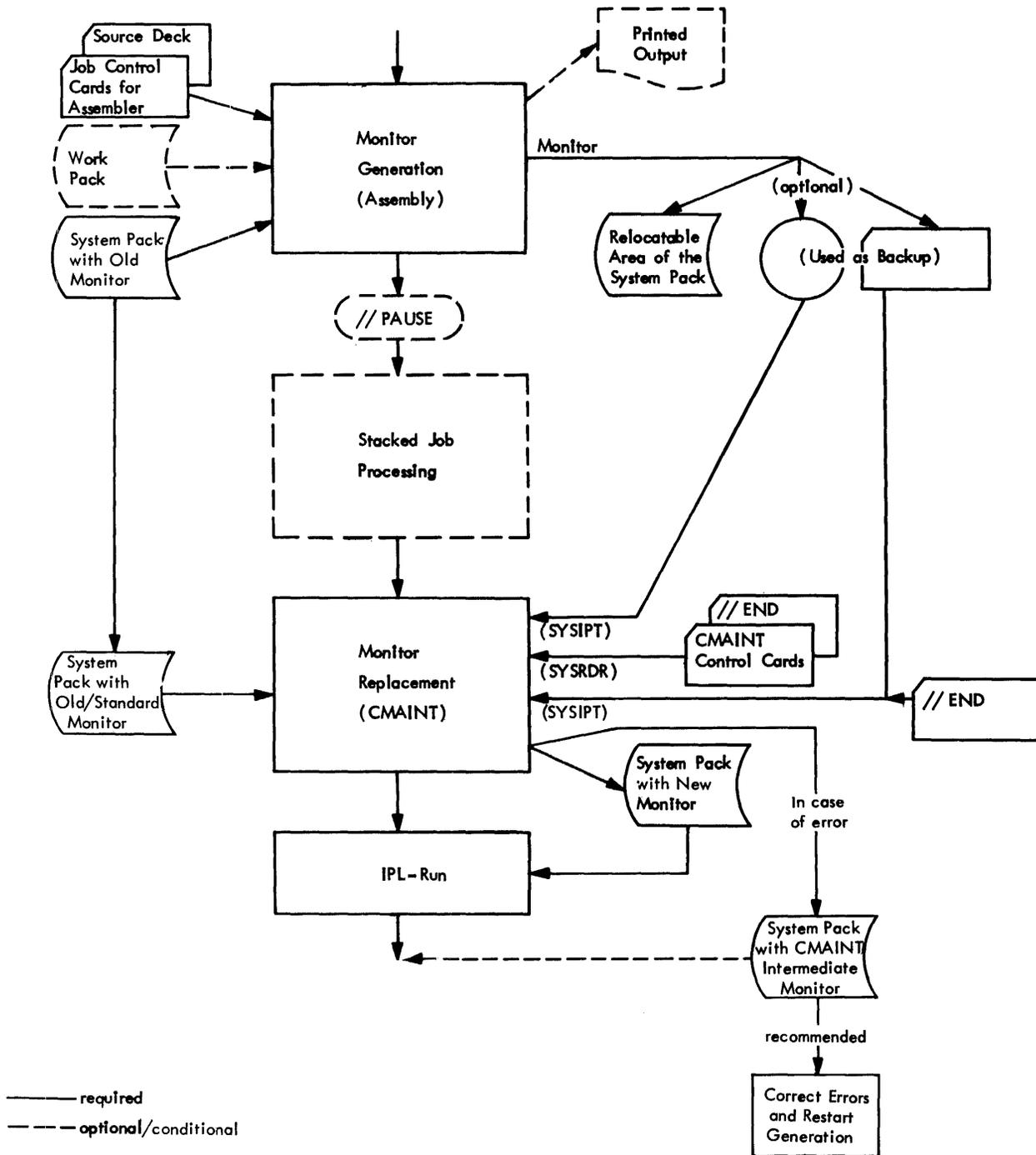
Figure 11. Generating a Disk-Resident Monitor and Including It on the System Pack
