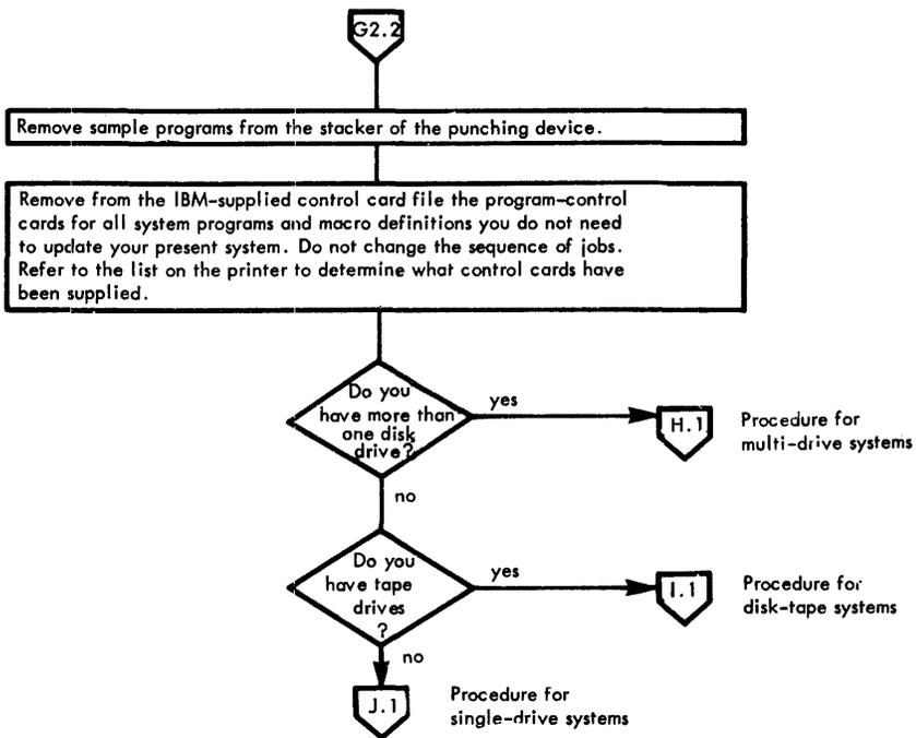
Chart G2. Punch Out IBM-Supplied Control-Card File and, if Desired, New or Changed Sample Programs, Part 2 of 2
