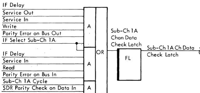
Figure 3B-74. Channel Data Check Latch
