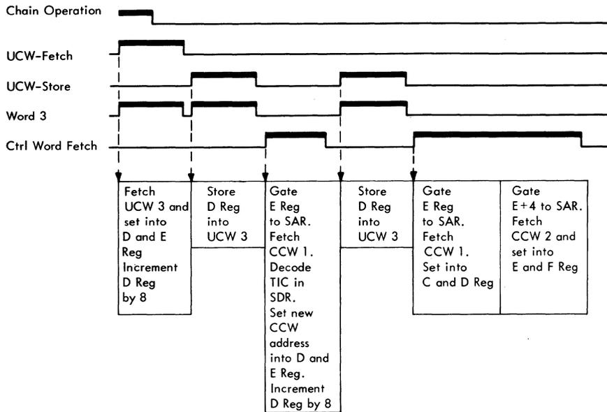
Figure 3B-28. Transfer-in-Channel Sequence
