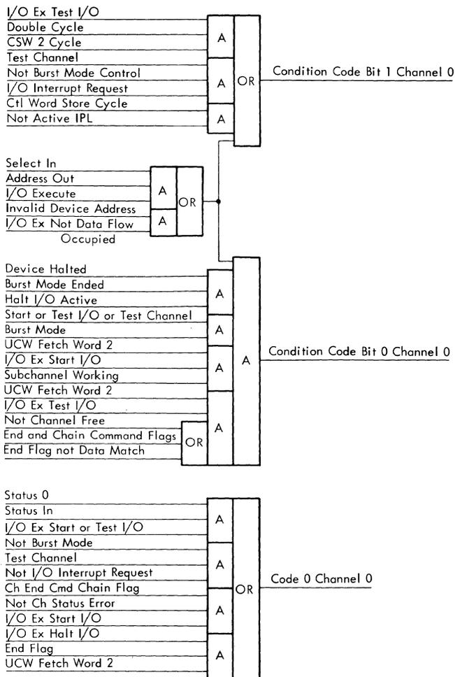
Figure 3B-32. Channel 0 Condition Code Generation
