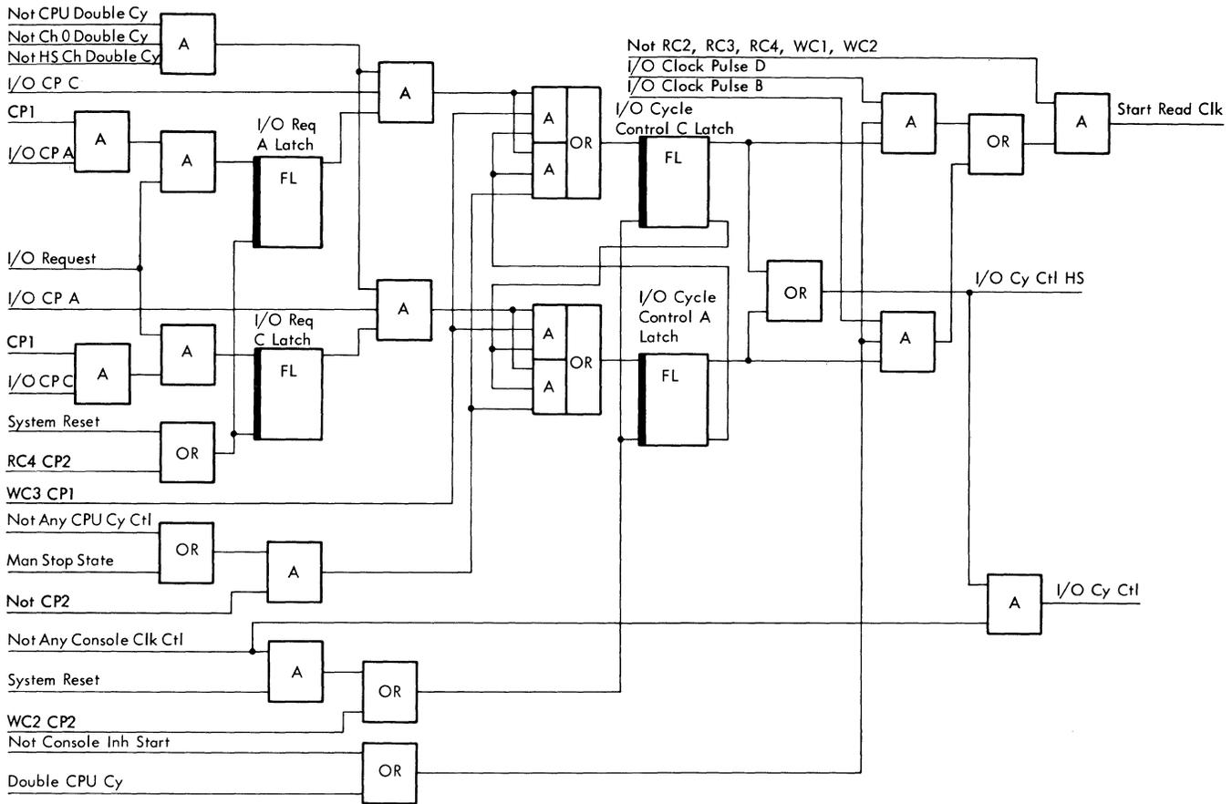
Figure 3B-8. I/O Cycle Request Latches
