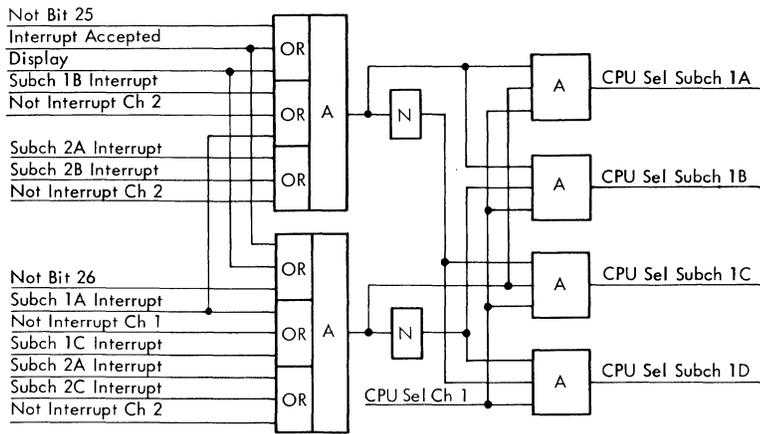
Figure 3B-40. CPU Subchannel Select and Interrupt Priority
