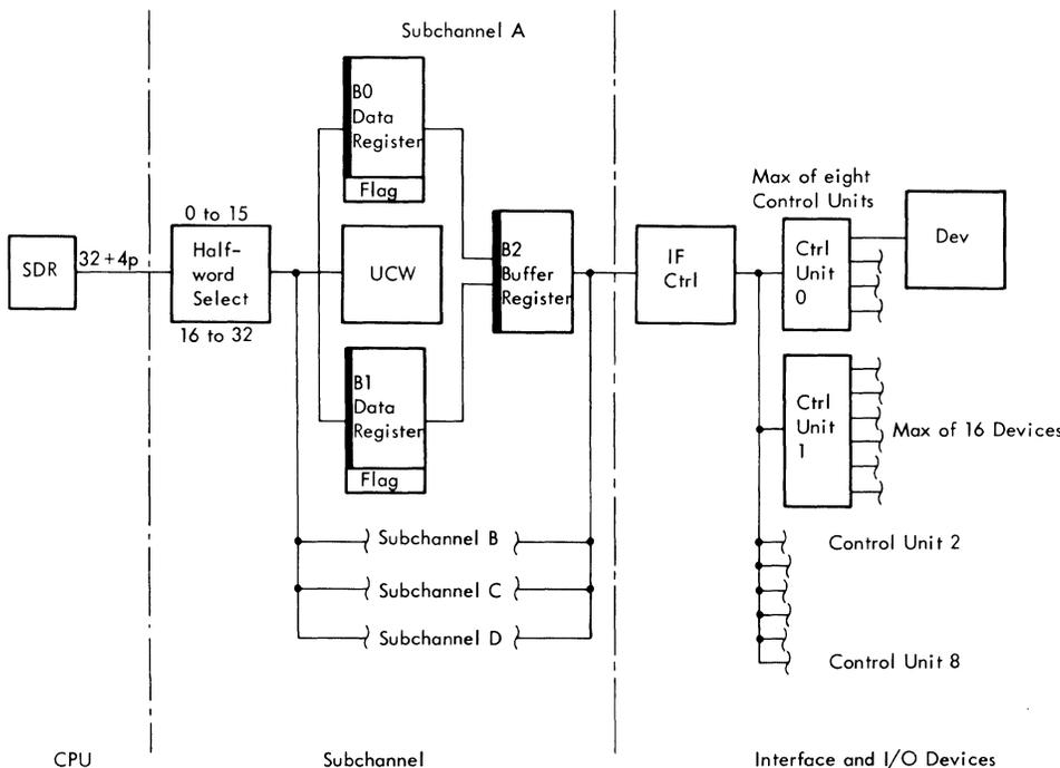
Figure 3B-35. HSMPX Simplified Channel Data Flow
