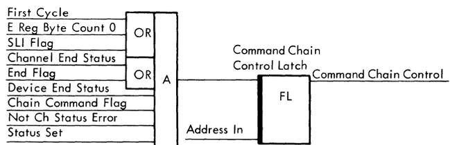
Figure 3B-26. Command Chain Control Latch
