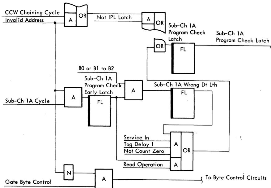
Figure 3B-76. Program Check set by Invalid Address
