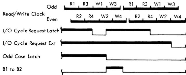
Figure 3B-59. Data Fetch for Write (Odd Address)
