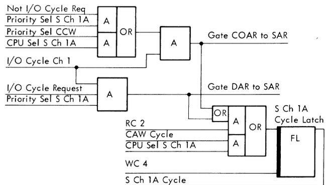
Figure 3B-12. Subchannel Cycle Latch
