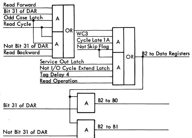
Figure 3B-54. Gating of B2 Buffer Register to Data Register
