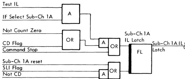
Figure 3B-73. Incorrect Length Latch
