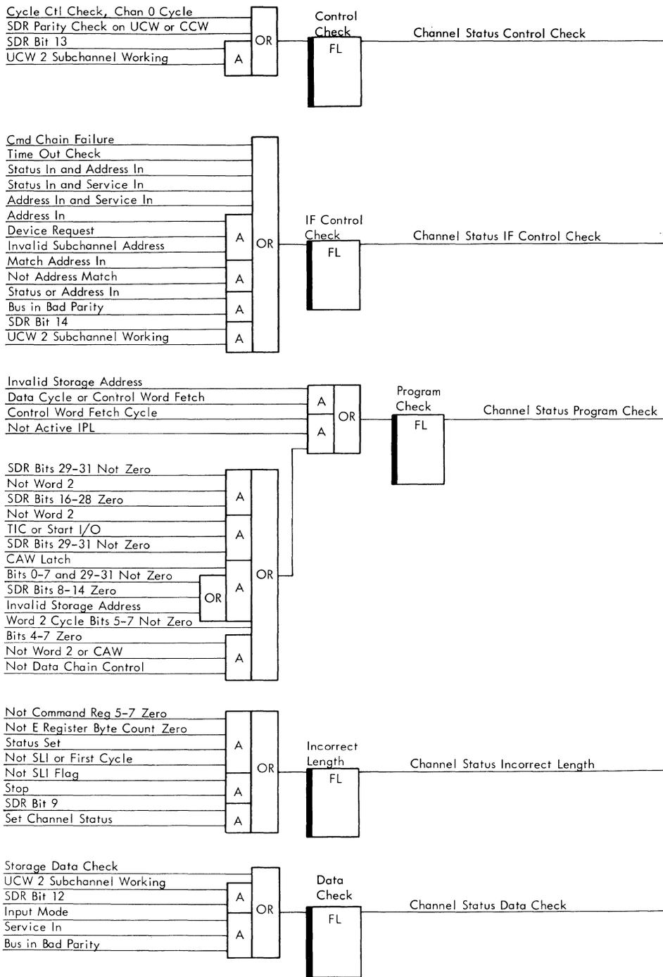
Figure 3B-34. Channel 0 Check Latches
