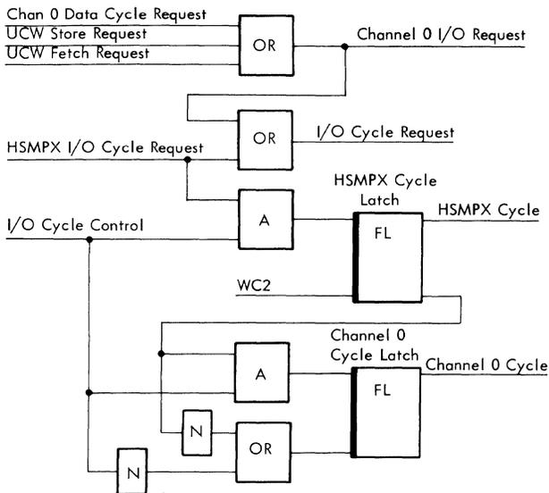
Figure 3B-6. Channel 0 I/O Cycle Request and Channel Cycle Latches
