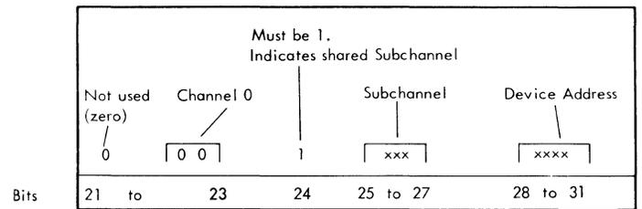
Figure 3B-19. Shared Subchannel Address Format
