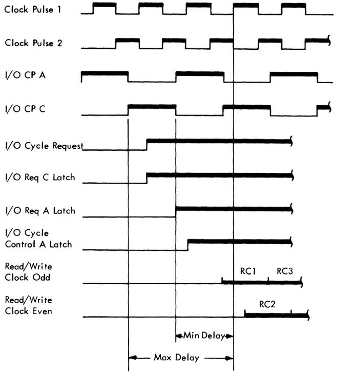
Figure 3B-9. I/O Cycle Request with no Read/Write Cycle
