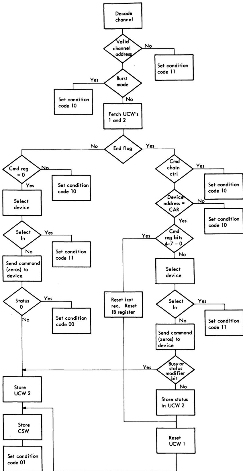
Figure 3B-30. Test I/O
