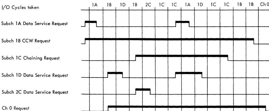
Figure 3B-5. Example of I/O Cycles taken for the Different Channels
