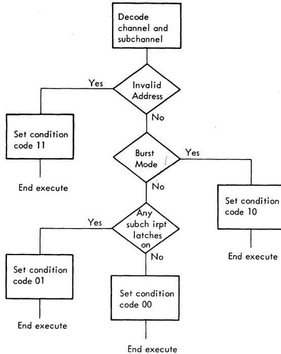
Figure 3B-69. Test Channel
