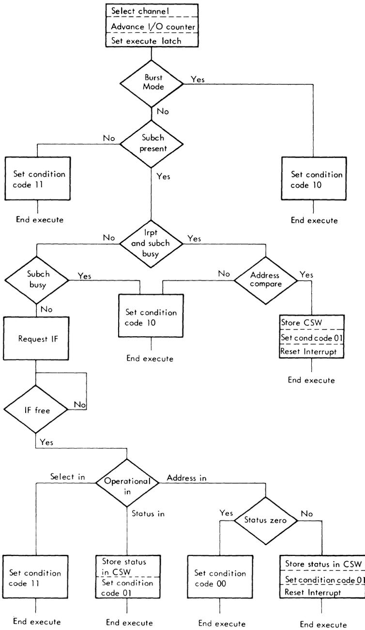
Figure 3B-66. Test I/O (HSMPX Channel)
