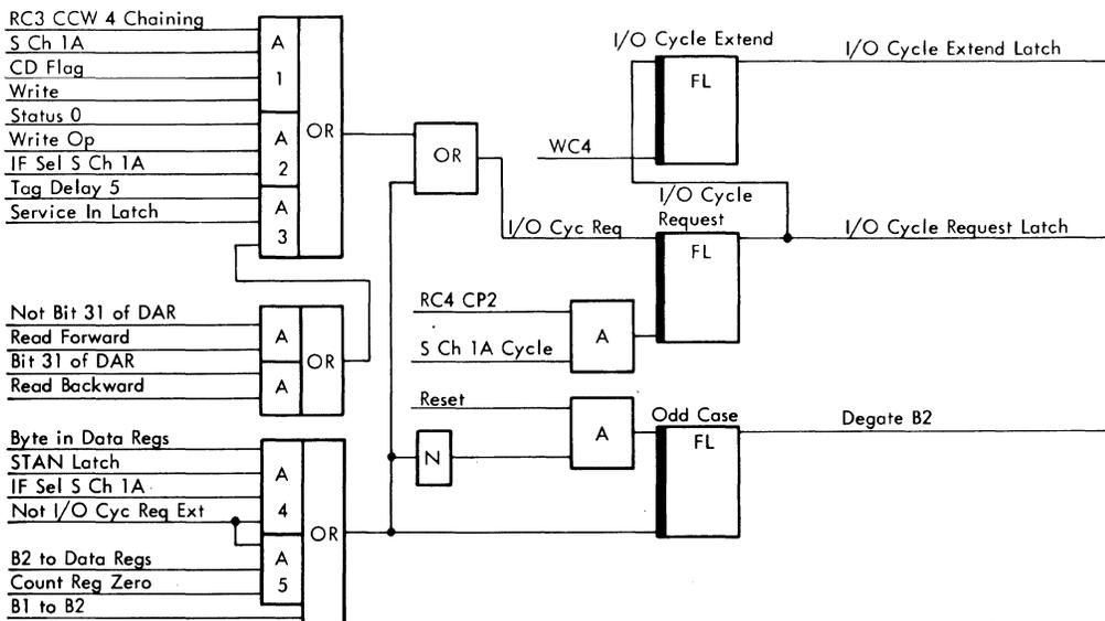
Figure 3B-55. I/O Cycle Request and Extend Latches
