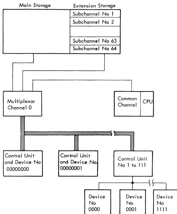
Figure 3B-13. MPX Channel 0 Data Flow Block Diagram
