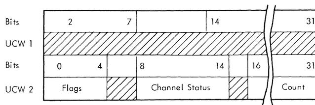
Figure 3B-25. UCW 1 and 2 Contents after Device End
