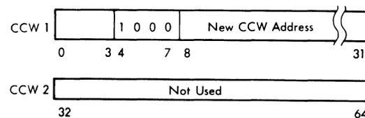
Figure 3B-27. Transfer-in-Channel, CCW Format
