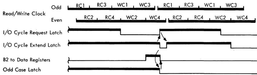
Figure 3B-57. End Read (Three Bytes of Data in Subchannel)
