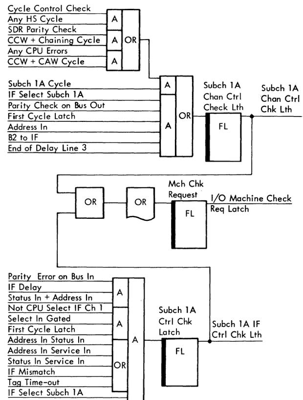
Figure 3B-77. Channel Control Check and IF Control Check Latches
