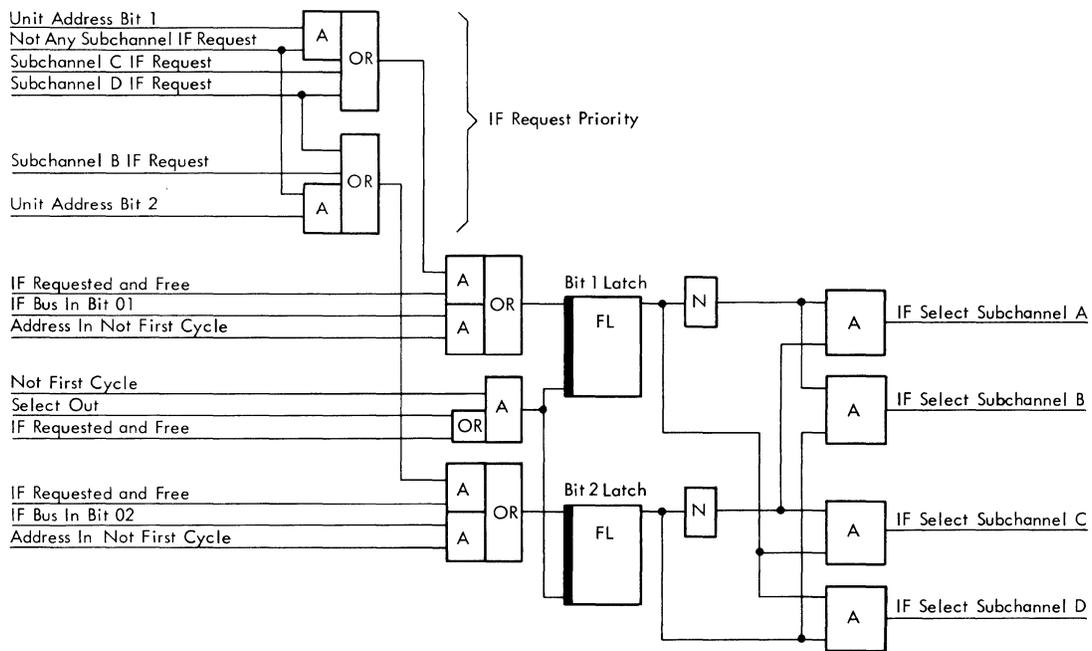
Figure 3B-41. IF Subchannel Select Register, Select Decode and Request Priority
