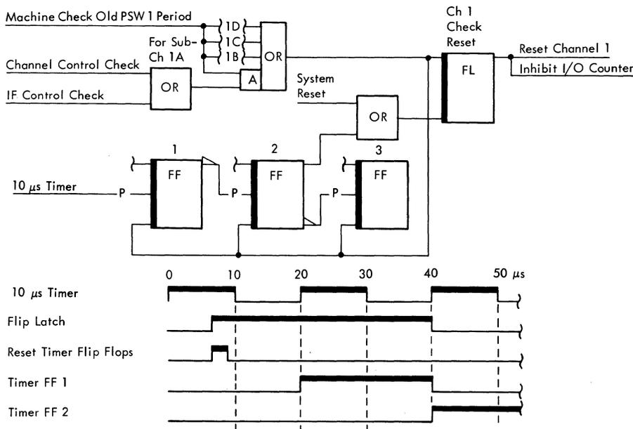
Figure 3B-78. Channel Reset by Machine Check
