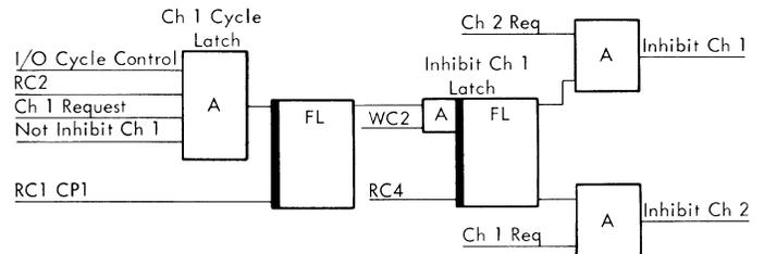
Figure 3B-11. HSMPX Channels 1 and 2 Priority
