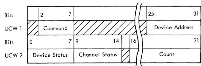
Figure 3B-24. UCW 1 and 2 Contents after Channel End
