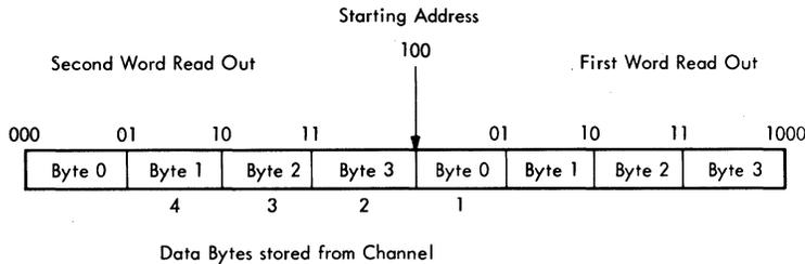
Figure 3B-56. Example of Even Starting Address (Read Backward)
