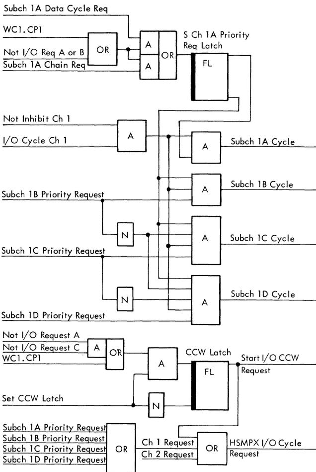
Figure 3B-7. HSMPX Channel I/O Cycle Request
