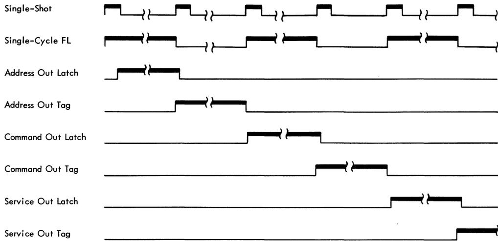
Figure 3B-46. Single-Cycle Timing for Initial Selection (Service-In)
