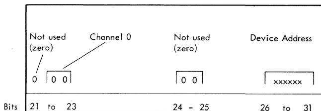
Figure 3B-18. Single Subchannel Address Format
