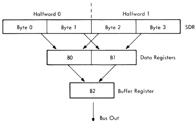
Figure 3B-58. Data Flow (Write)
