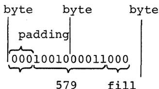
Figure 5-2. Bit-Length Specification (Single Constant)
