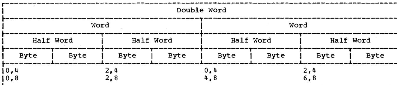
Figure 5-6. CNOP Alignment
