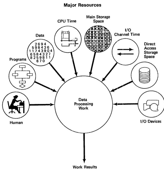
Figure 3. Resources Required to Process Data Automatically
