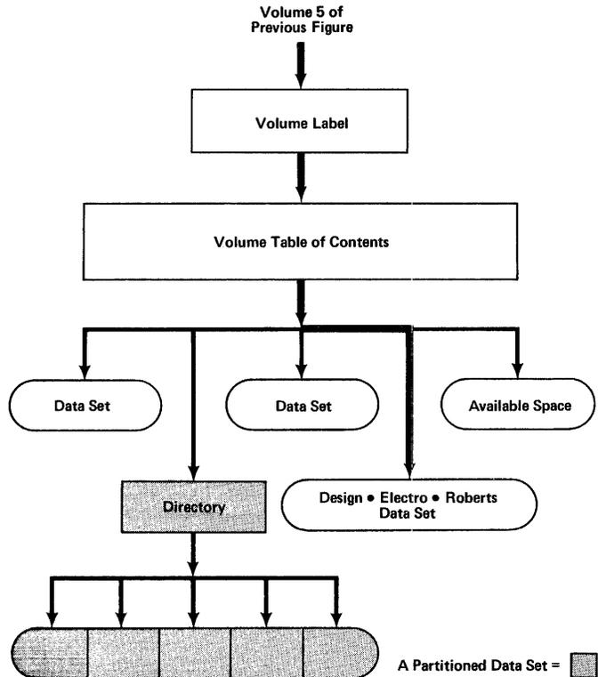
Figure 54. Simplified Diagram of Catalog System For Locating Data Sets Within a Direct Access Volume
