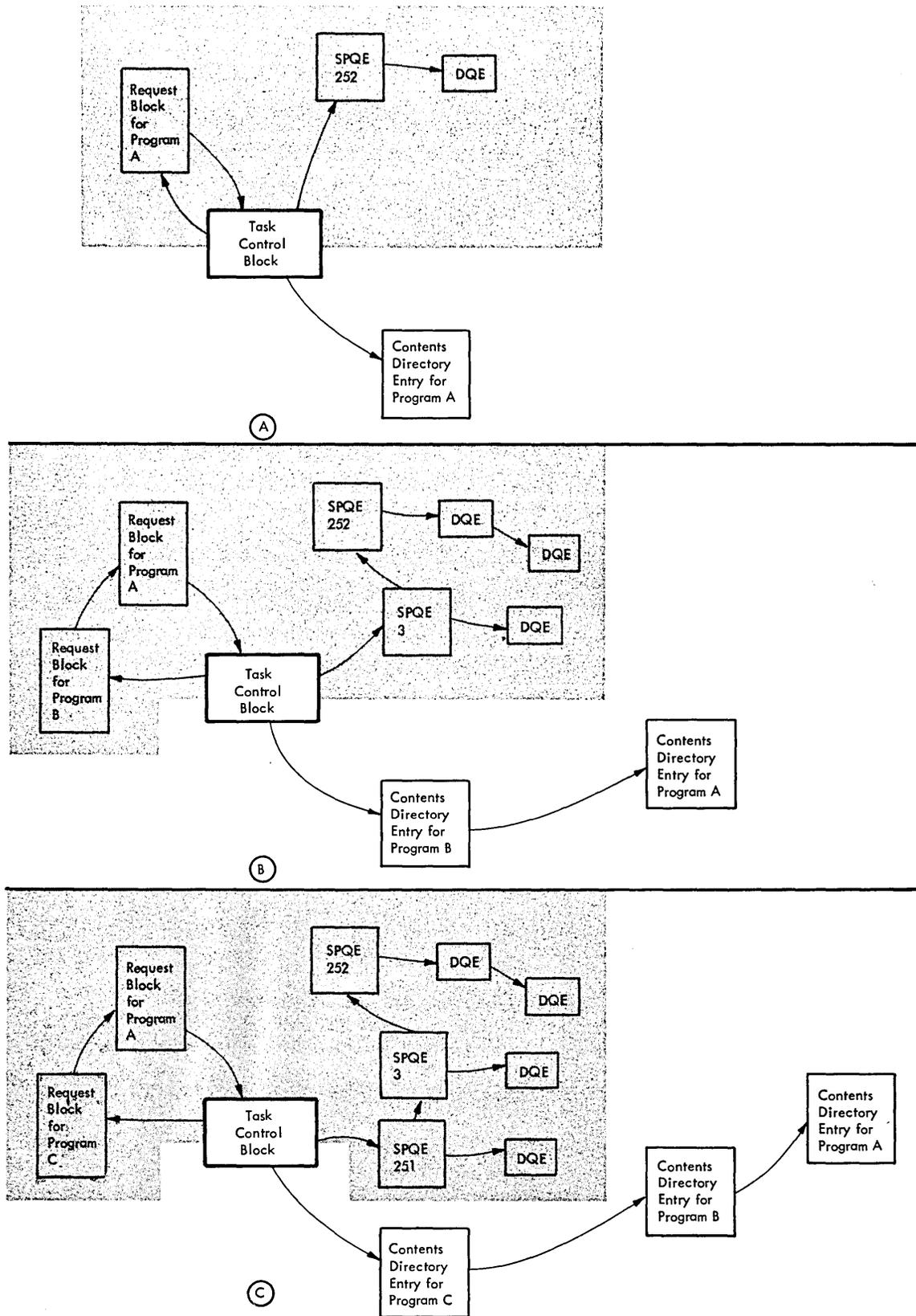
Figure 25. Example of the Modification of Contents Directory During a Task
