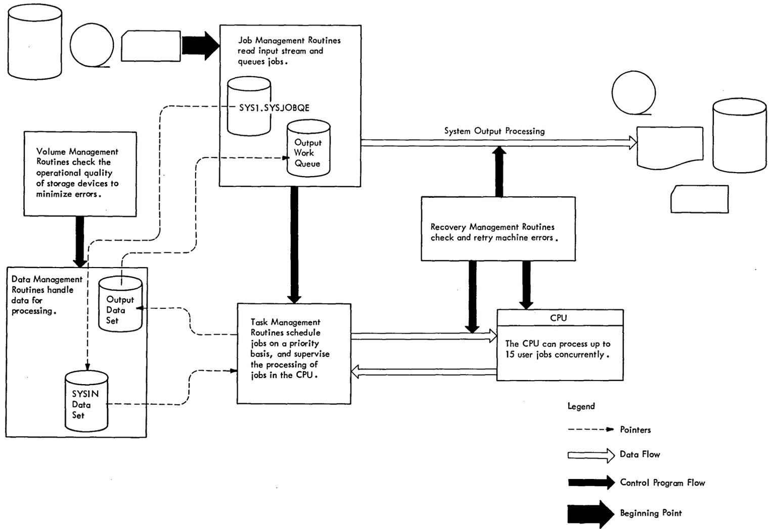
Figure 6: MVT Control Program Routines
