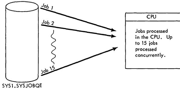
Figure 3. Jobs are Stored on SYS1.SYSJOBQE and then Processed
