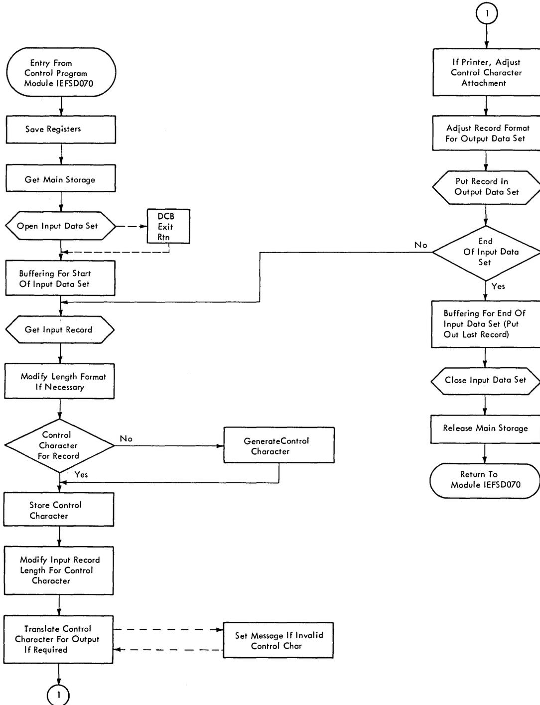
Figure 10. General Logic of Standard Output Writer
