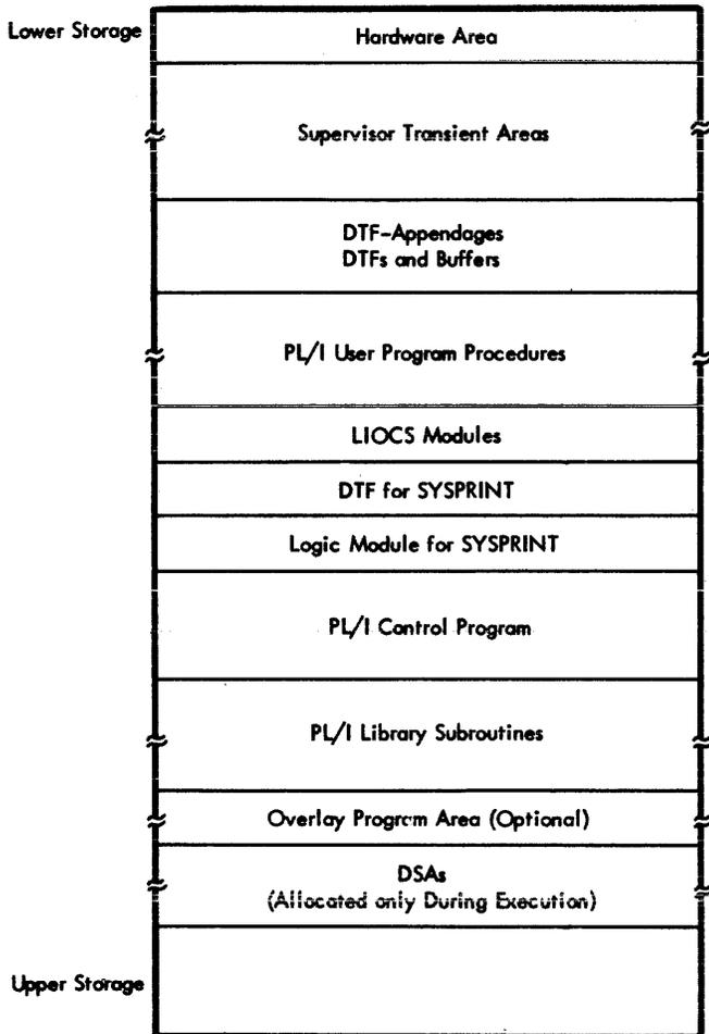
Figure 3. Object-Time Storage Layout
