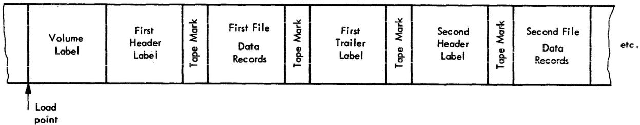
Figure 22. Format of Labeled Tape File
