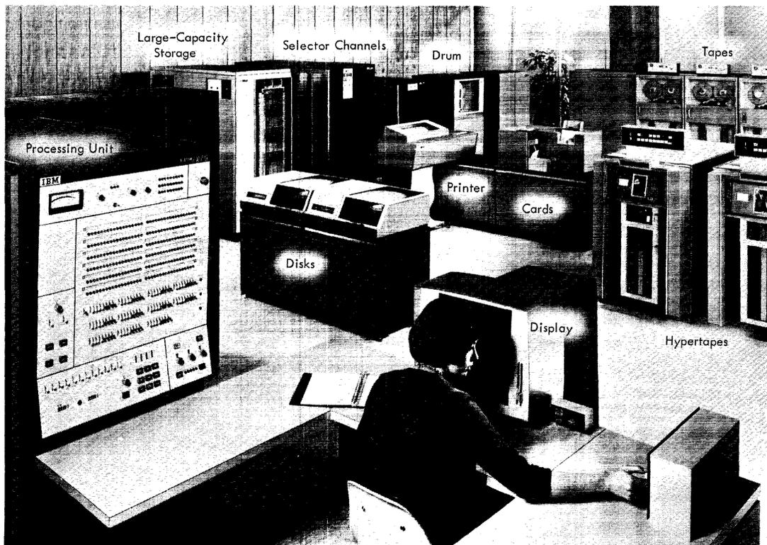
Figure 5. IBM System/360 Model 60
