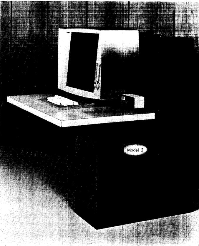
Figure 8. IBM 2250 Display Unit
