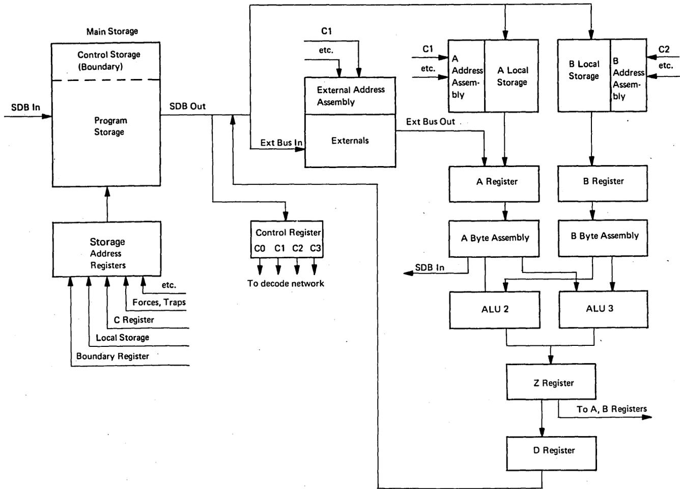
Figure 2. Simplified System/370 Model 145 CPU data flow
