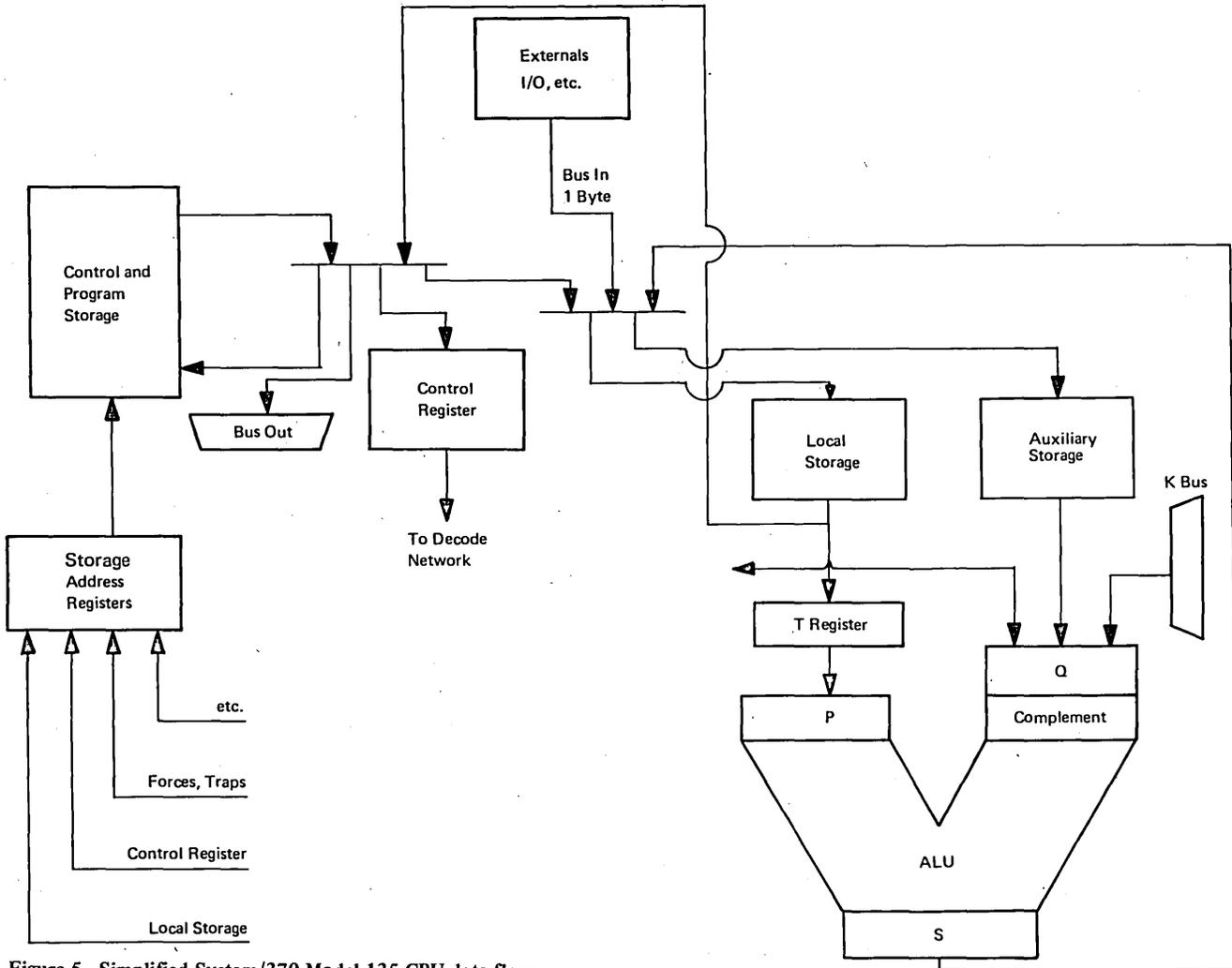
Figure 5. Simplified System/370 Model 135 CPU data flow
