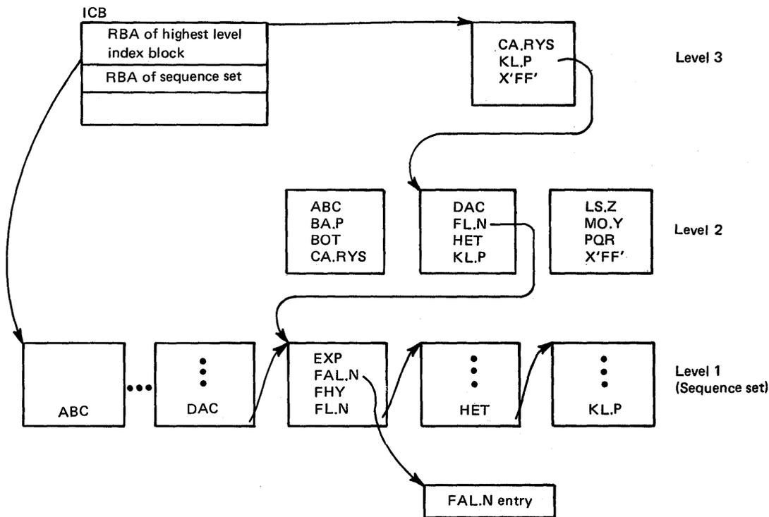
Figure 8-2. Example of a RACF Index
