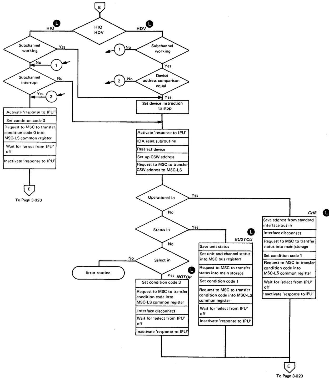
This routine is the continuation from the basic loop after analyzing the instruction identifier, the result being an interrupt.
