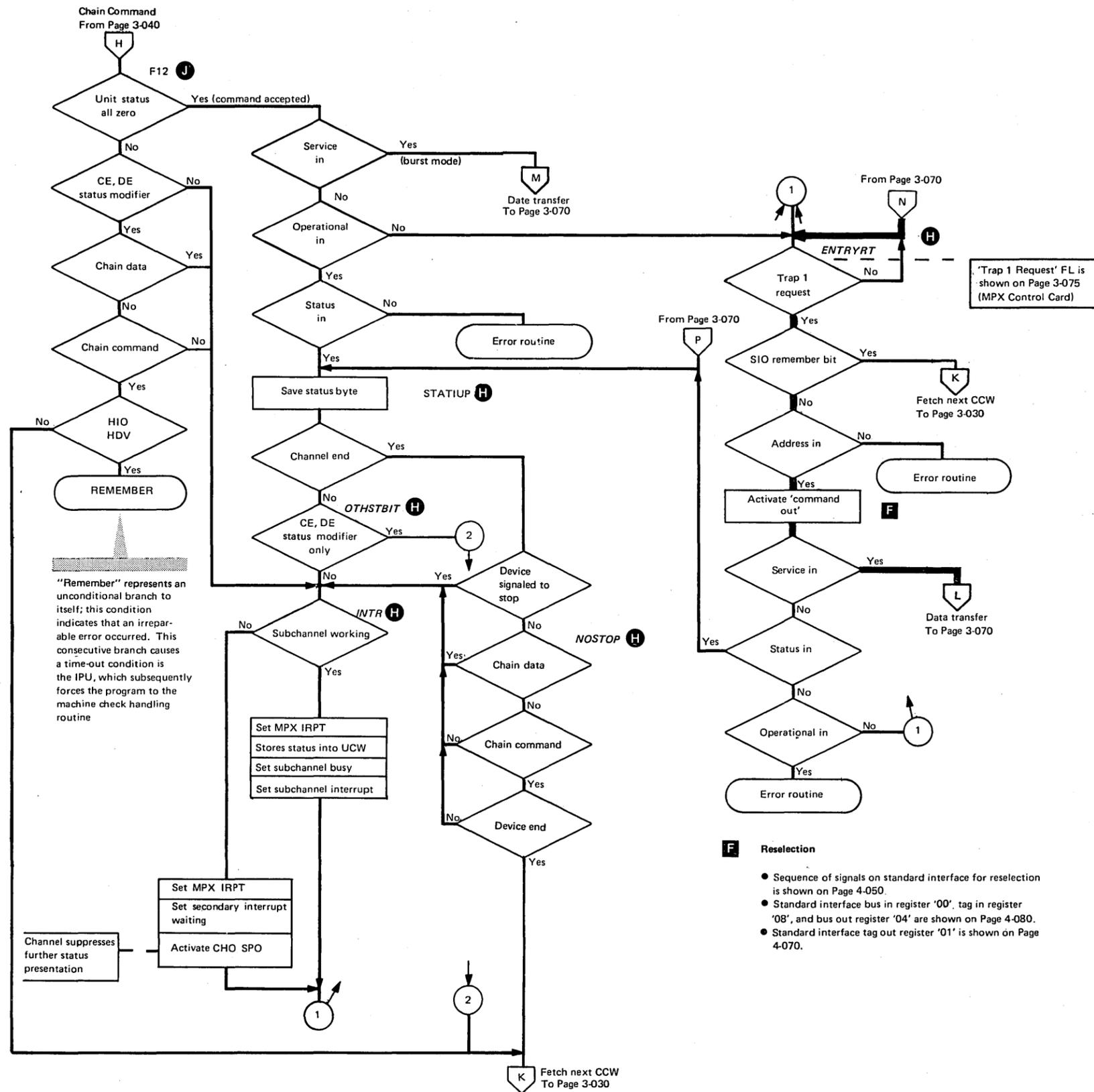
"Remember" represents an unconditional branch to itself; this condition indicates that an irreparable error occurred. This consecutive branch causes a time-out condition is the IPU, which subsequently forces the program to the machine check handling routine
