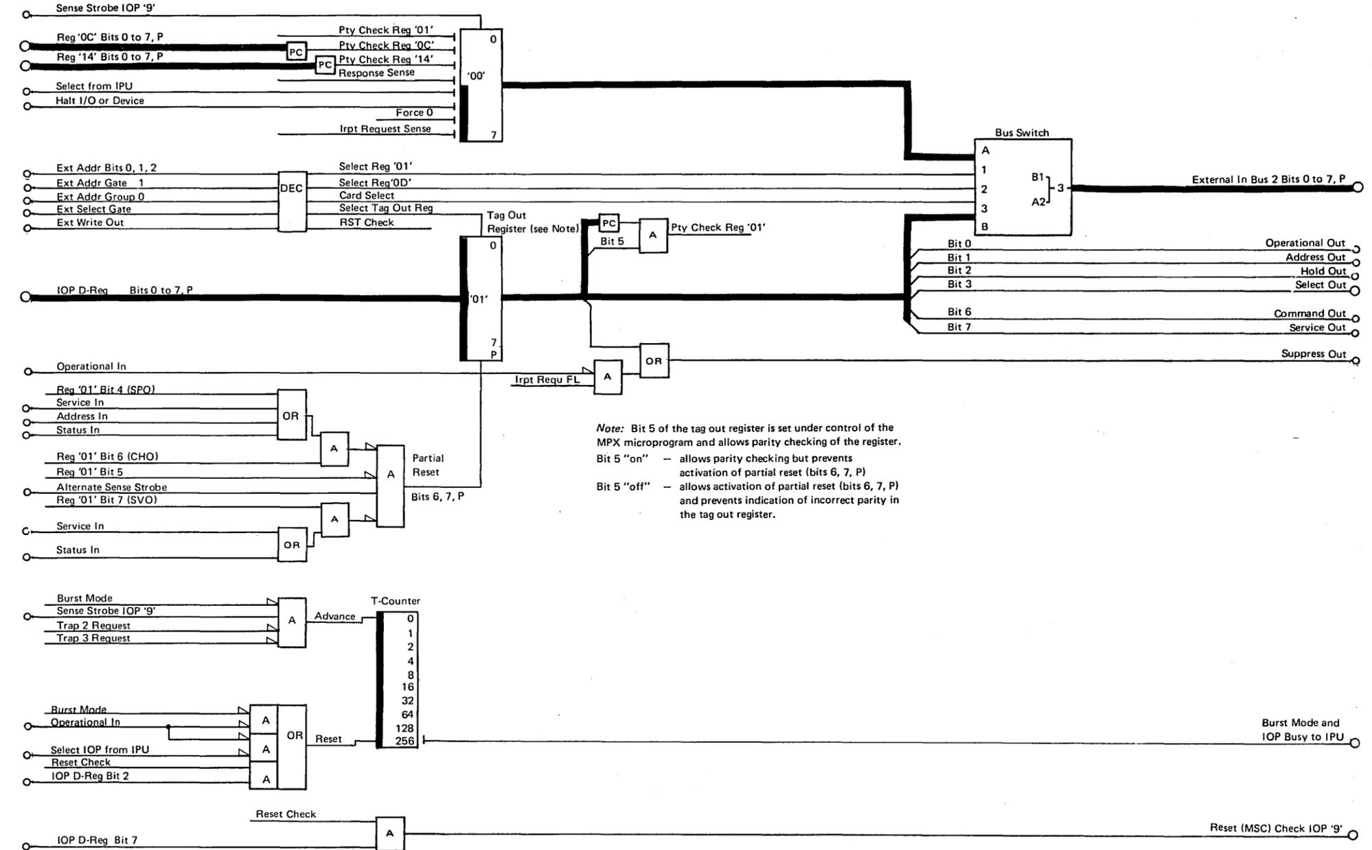
Note: Bit 5 of the tag out register is set under control of the MPX microprogram and allows parity checking of the register.
