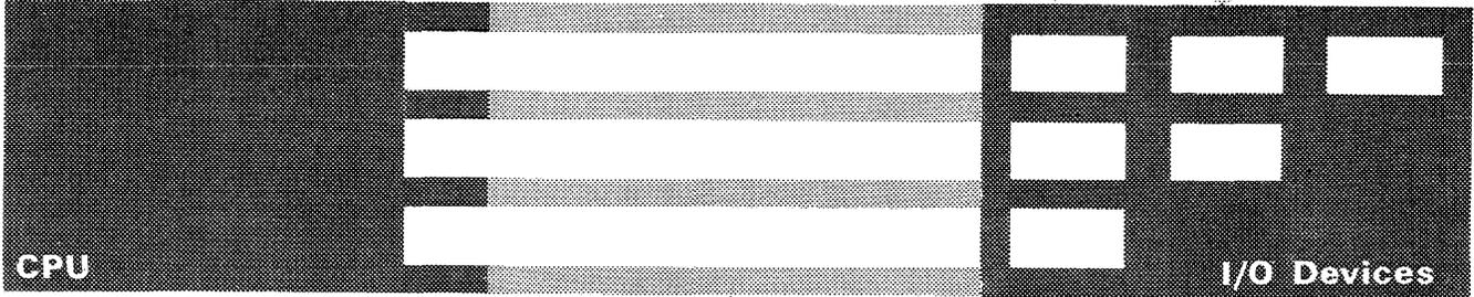
Specialized integrated adapters, integrated attachments, a direct disk attachment, and a standardized channel are used for attaching I/O devices. The integrated adapters, attachments, and the channel work like System/360 channels. For programming purposes, the I/O attachment facilities are considered to consist of three channels.
