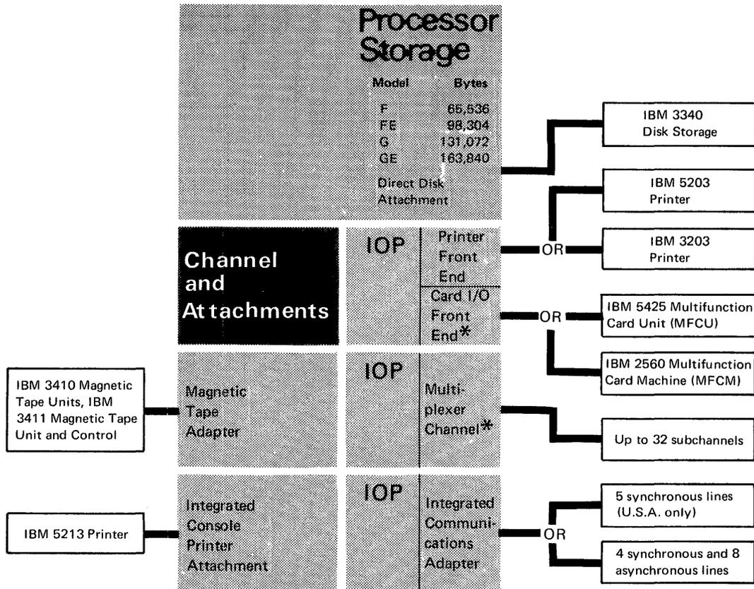
\*Either the integrated card I/O attachment or the multiplexer channel, but not both, can be attached to the Model 115.
