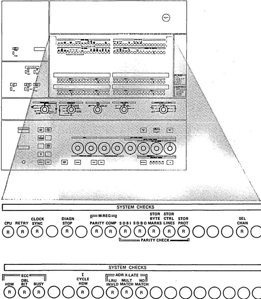
If a system check indicator is on, refer to the system check error recovery procedure.
