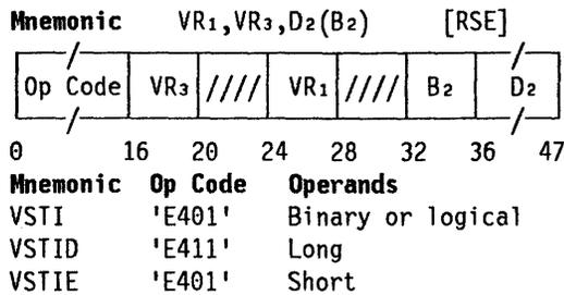
Element by element, the third operand is used to select element locations of the second operand in storage, at which elements of the first-operand vector are placed. The element positions of the first operand correspond to those of the third operand.
