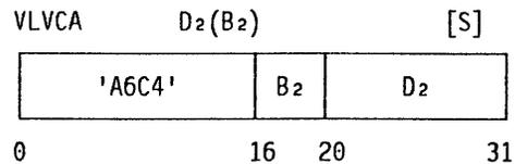
If the second-operand-address value is greater than zero, the vector count (VCT) is replaced by the lesser of the section size and the address value. If the second-operand-address value is zero or less than zero, the vector count is set to zero.
