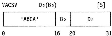
The current value of the vector-activity count (VAC) is stored at the doubleword designated by the second-operand address. Execution of this instruction does not increment the vector-activity count and leaves its value unchanged.
