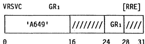
If the vector change bit associated with a specified pair of vector registers is one, the contents of those vector registers are placed in consecutive doublewords of a storage area called the save area of the vector-register pair, and the vector change bit is then set to zero. If the vector change bit is already zero, the vector registers are not stored. In either case, the address of the save area is incremented to the location of the save area of the next pair of vector registers.
