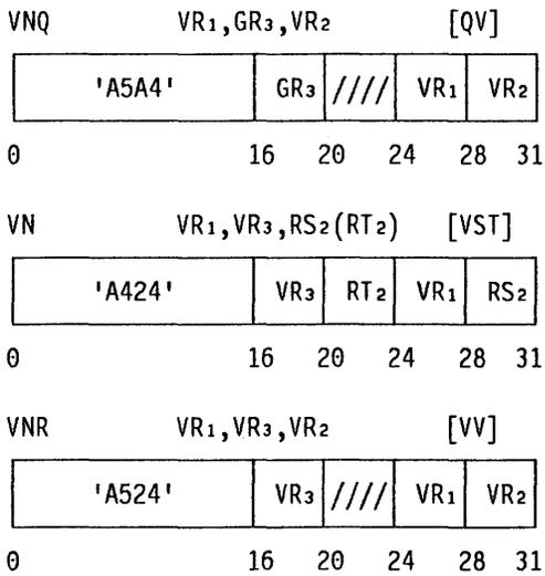
Element by element, the AND of the second and third operands is placed in the first-operand location.
