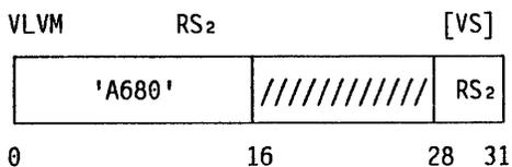
The second-operand bit vector replaces the active bits of the vector-mask register (VMR). Bits beyond the active bits are set to zeros.
