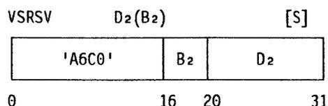
The contents of the vector-status register (VSR) are placed in storage at the doubleword location designated by the second-operand address, except that, when the CPU is in the problem state, the value of the vector change bits stored by the instruction is undefined.
