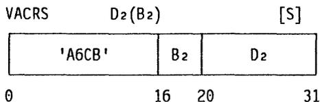
Bits 8-63 of the vector-activity count (*VAC*) are replaced by bits 8-63 of the doubleword designated by the second-operand address; bits 0-7 of the *VAC* are set to zeros. Execution of this instruction does not increment the vector-activity count and leaves the loaded value unchanged.
