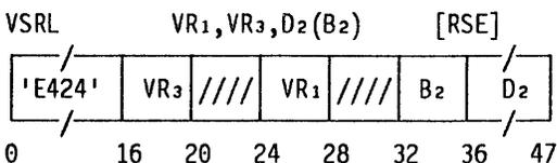
One by one, the elements in the third-operand vector are shifted left (VSLL) or right (VSRL) by the number of bits specified by the second-operand address, and the result is placed in the first-operand location.
