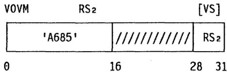
The *OR* of the second-operand bit vector and of the active bits of the vector-mask register (*VMR*) is placed in the vector-mask register. Bits beyond the active bits are set to zeros.
