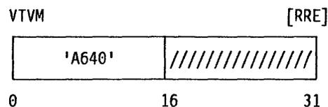
The active bits of the vector-mask register are tested, and condition code 0, 1, or 3 is set according to whether those bits are all zeros, mixed zeros and ones, or all ones.
