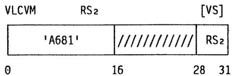
The complement of the bits from the second-operand bit vector replaces the active bits of the vector-mask register (VMR). Bits beyond the active bits are set to zeros.
