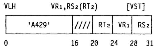
Element by element, the second operand is extended from a vector of 16-bit signed binary integers to a vector of 32-bit signed binary integers, and the result is placed in consecutive first-operand locations.
