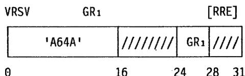
If the vector in-use bit associated with a specified pair of vector registers is one, the contents of those vector registers are placed in consecutive doublewords of a storage area called the save area of the vector-register pair. If the vector in-use bit is zero, the vector registers are not stored. In either case, the address of the save area is incremented to the location of the save area of the next pair of vector registers.
