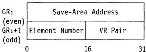
Depending on the address size, the rightmost 31 or 24 bits of the contents of the even general register are used as the save-area address. When the general register is updated to the address of the next location, the leftmost one or eight bit positions, respectively, of the general register are set to zeros.
