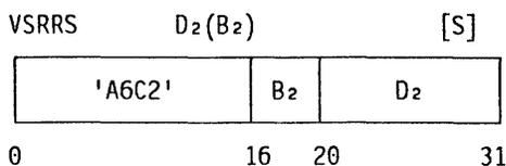
The contents of the vector-status register (VSR) are replaced by the doubleword designated by the second-operand address, and vector registers may be cleared depending on the vector in-use bits.
