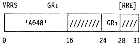
If the vector in-use bit associated with a specified pair of vector registers is one, the contents of those vector registers are replaced by consecutive doublewords from a storage area called the save area of the vector-register pair. If the vector in-use bit is zero, the vector registers remain unchanged. In either case, the address of the save area is incremented to the location of the save area of the next pair of vector registers.
