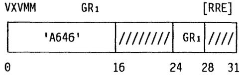
Bits 16-31 of the general register designated by GR<sub>1</sub> are set to the value of bits 0-15 of the vector-status register. Thus, bit 31 of the general register indicates the current setting of the vector-mask mode. Bits 0-15 of the general register are set to zeros.
