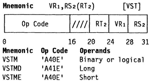
Element by element, elements of the first-operand vector corresponding to ones in the active bits of the vector-mask register are placed unchanged in storage at the corresponding element locations of the second operand. Elements of the first operand corresponding to zeros in the active bits of the vector-mask register are not stored, and the corresponding second-operand locations in storage remain unchanged.
