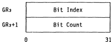
Both are treated as 32-bit signed binary integers. The bit index identifies the first bit of the second operand to be processed. The bit count gives the number of bits to be processed. If the bit count is zero or less than zero, no bits are processed. Upon completion or interruption of the instruction, the bit index identifies the next bit to be processed, and the bit count, if greater than zero, gives the number of bits remaining.
