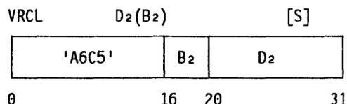
The specified pairs of vector registers are cleared, the associated vector in-use bits and vector change bits are set to zeros, and the vector interruption index is set to zero.
