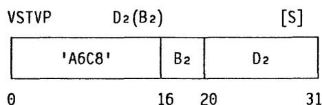
The 16-bit section size and the 16-bit partial-sum number are placed in storage in the left and right half, respectively, of the word at the location designated by the second-operand address.
