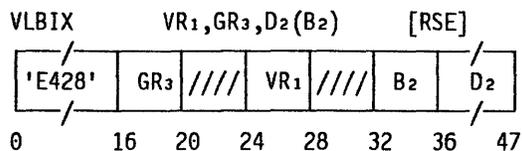
Bit by bit, the second operand is converted from a bit vector to a vector of element numbers, the result vector is placed in the first-operand location, and the number of elements in the result vector is placed in the vector count.
