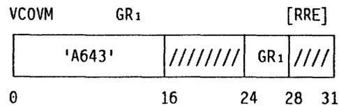
Selected bits among the active bits of the vector-mask register (VMR) are counted, and the count is added to the contents of the general register designated by GR<sub>1</sub>. For the COUNT LEFT ZEROS IN VMR instruction, the selected bits are the zero bits to the left of the leftmost one bit. For the COUNT ONES IN VMR instruction, the selected bits are the one bits.
