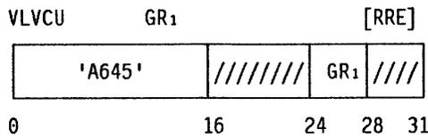
If the operand in the general register designated by the GR<sub>1</sub> field is greater than zero, the vector count (VCT) is replaced by the lesser of the section size and the operand. If the operand is zero or less than zero, the vector count is set to zero. The general register is then updated by subtracting the new vector count from the register contents.
