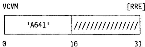
The active bits of the vector-mask register (VMR) are complemented. Bits beyond the active bits of the vector-mask register are set to zeros.
