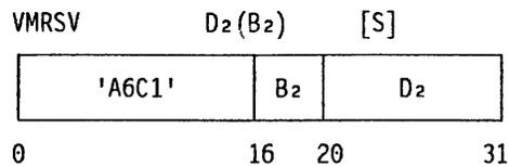
The contents of the entire vector-mask register (VMR) are placed unchanged in storage at the second-operand location.
