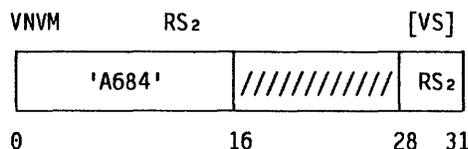
The *AND* of the second-operand bit vector and of the active bits of the vector-mask register (VMR) is placed in the vector-mask register. Bits beyond the active bits are set to zeros.
