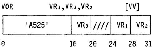
Element by element, the *OR* of the second and third operands is placed in the first-operand location.
