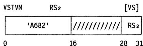
The contents of the active-bit positions of the vector-mask register are stored as a bit vector at the second-operand location.
