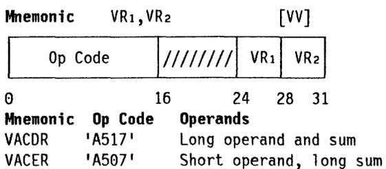
Partial sums of the elements of the second-operand vector are accumulated by adding the second-operand elements to the contents of element positions 0 to  $p-1$  of the first operand. The partial-sum number  $p$  depends on the model.
