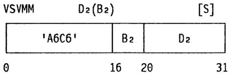
The vector-mask mode is set on or off, depending on whether the rightmost bit, bit 31, of the second-operand address is one or zero, respectively. The second-operand address is not used to address data, and all address bits other than bit 31 are ignored.
