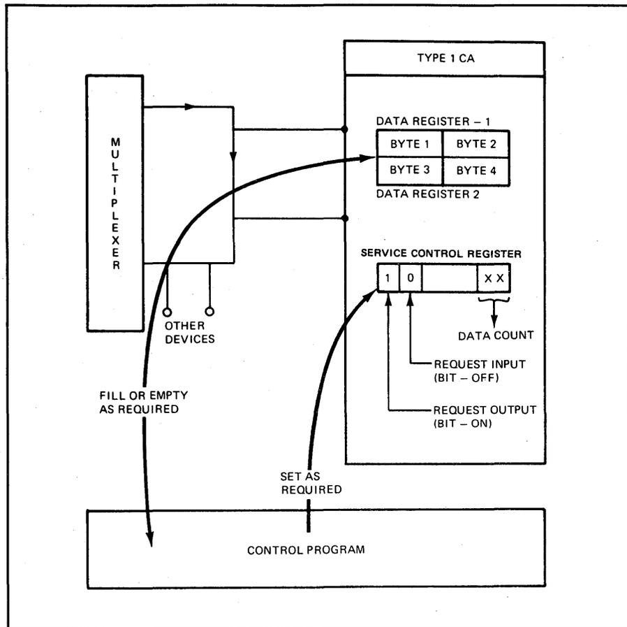
Figure E.2 Type 1 Channel Adapter Data Transfer
