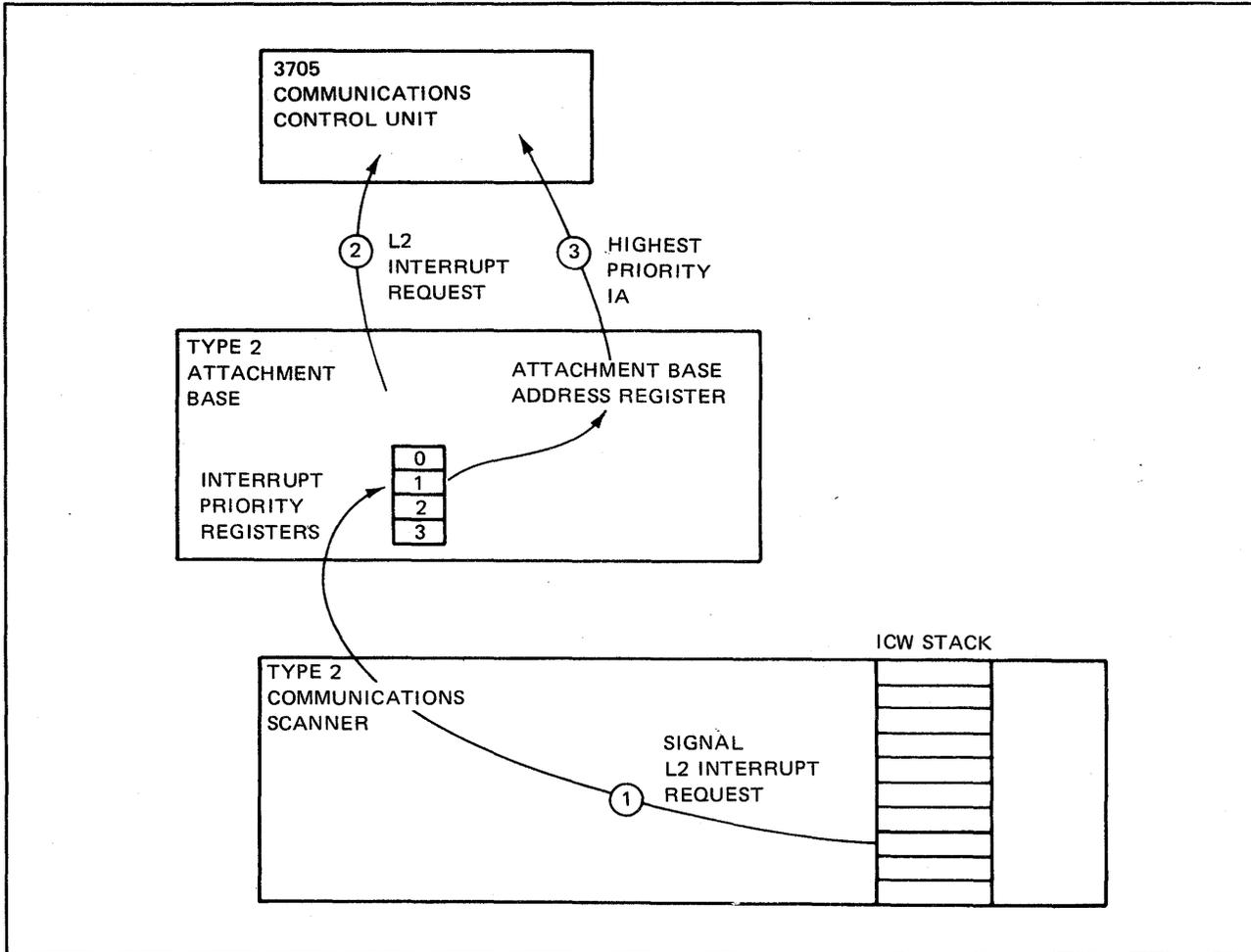
Figure J.8 Level 2 Interrupt Request.
