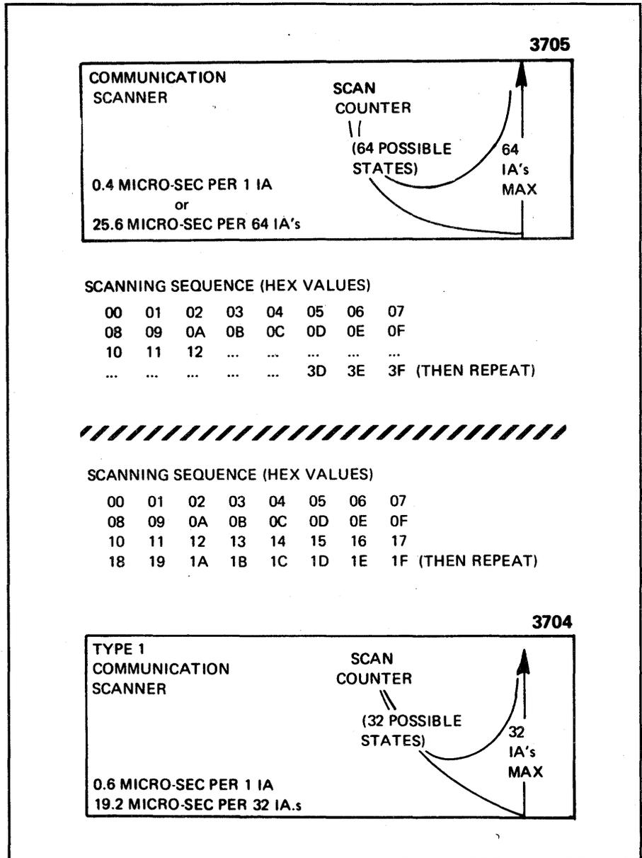
Figure I.3 Scanning Sequence for a Type 1 CS
