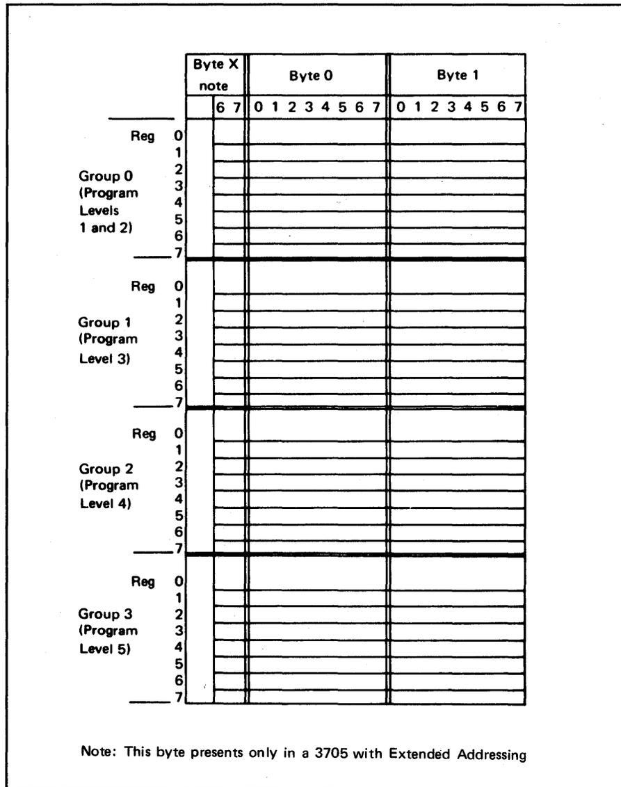
Figure B.1 Function of the Program Levels in the Network Control Program
