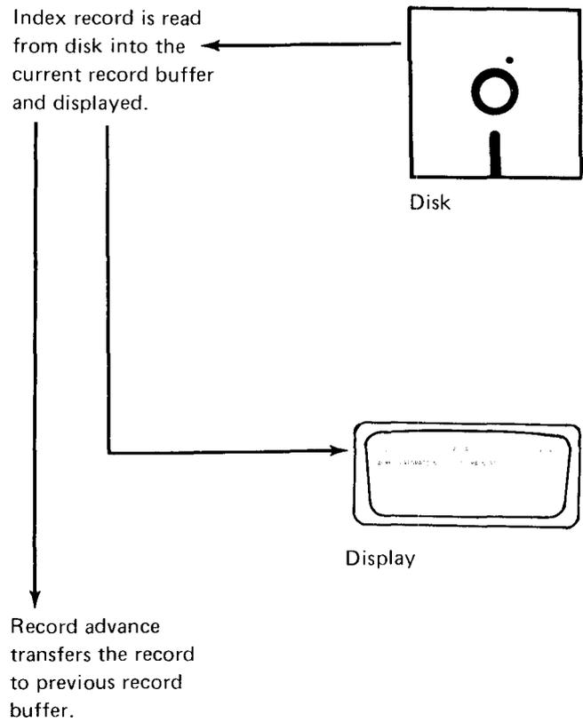
Figure 6. Data Flow for Read Index Mode
