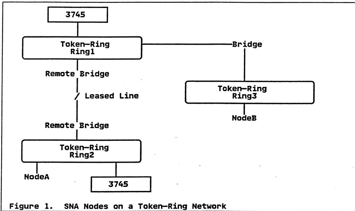
Figure 1. SNA Nodes on a Token-Ring Network
