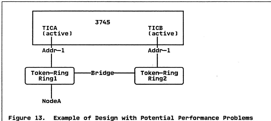
**Figure 13. Example of Design with Potential Performance Problems**
