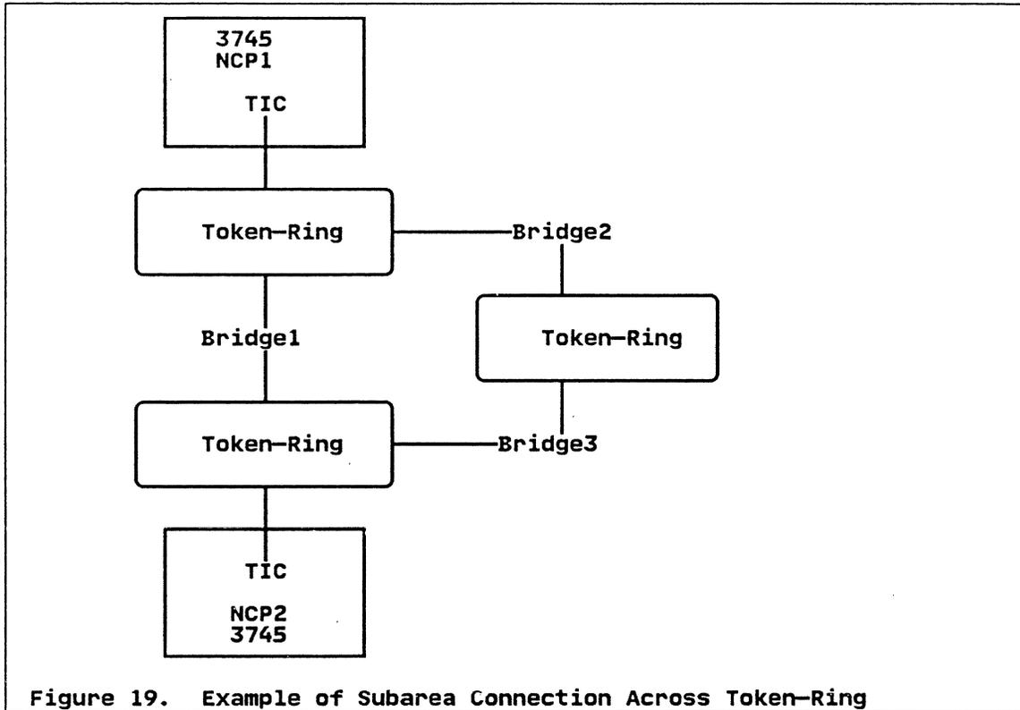
**Figure 19. Example of Subarea Connection Across Token-Ring**
