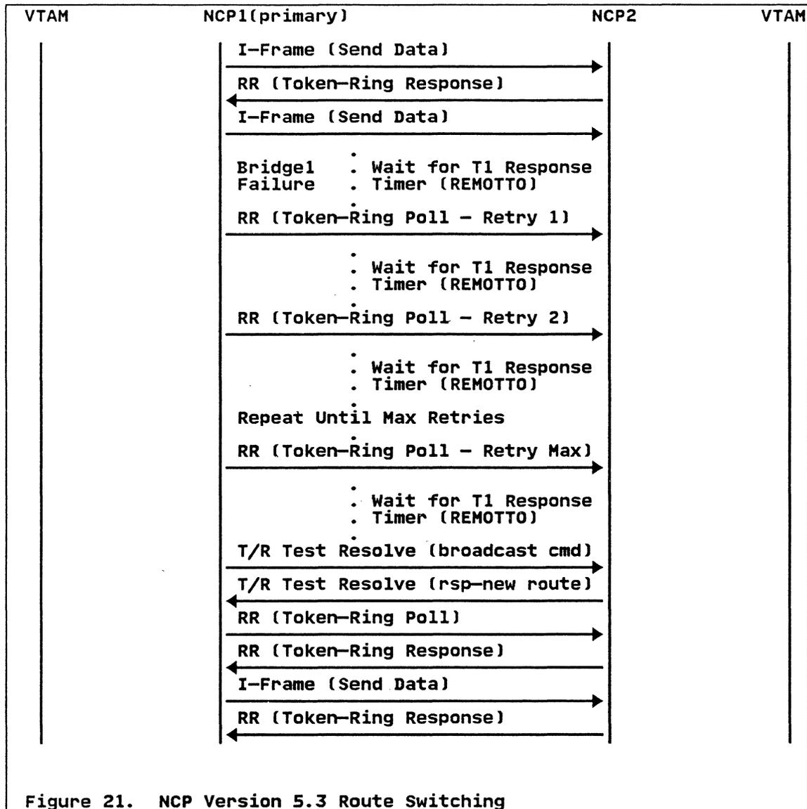
In the diagram above, NCP1 holds up its sessions while it tries to find a new Token-Ring route by resending the Test Resolve Token-Ring Frame. When it gets a response to the Test-Resolve, NCP1 updates its tables and polls the remote NCP. After receiving a positive response, NCP1 continues sending data.
