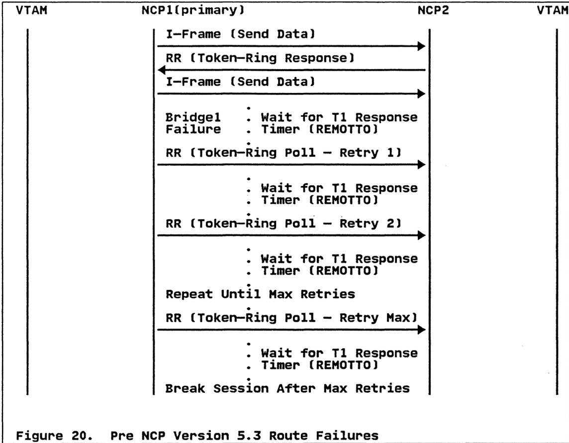
Each frame across the Token-Ring is acknowledged within the timer specified in the NCP generation (REMOTTO or LOCALTO). If a frame is not acknowledged in time, then NCP polls the remote NCP. After the maximum number of retries is attempted, then NCP breaks the INN session.
