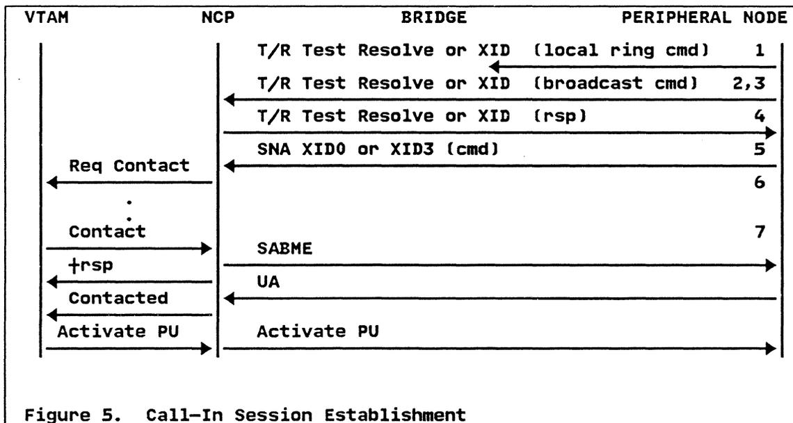
(Note: The description above is not intended to describe the detailed flows between VTAM, NCP and the Node. It provides a basic understanding of the command flows which occur to make the Token-Ring node known to the VTAM host. The numbers under the peripheral node correspond to the text above the figure).
