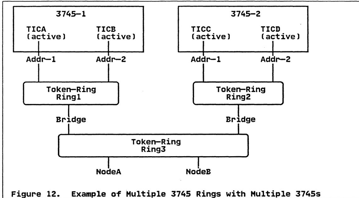
In the figure above, both 3745s have two concurrently active TICs. Both TICA and TICC are active at Token-Ring address Addr-1; TICB and TICC at Token-Ring address Addr-2. Therefore, TICA and TICC concurrently support traffic from SNA nodes accessing the host at gateway address Addr-1; TICB and TICC at address Addr-2.
