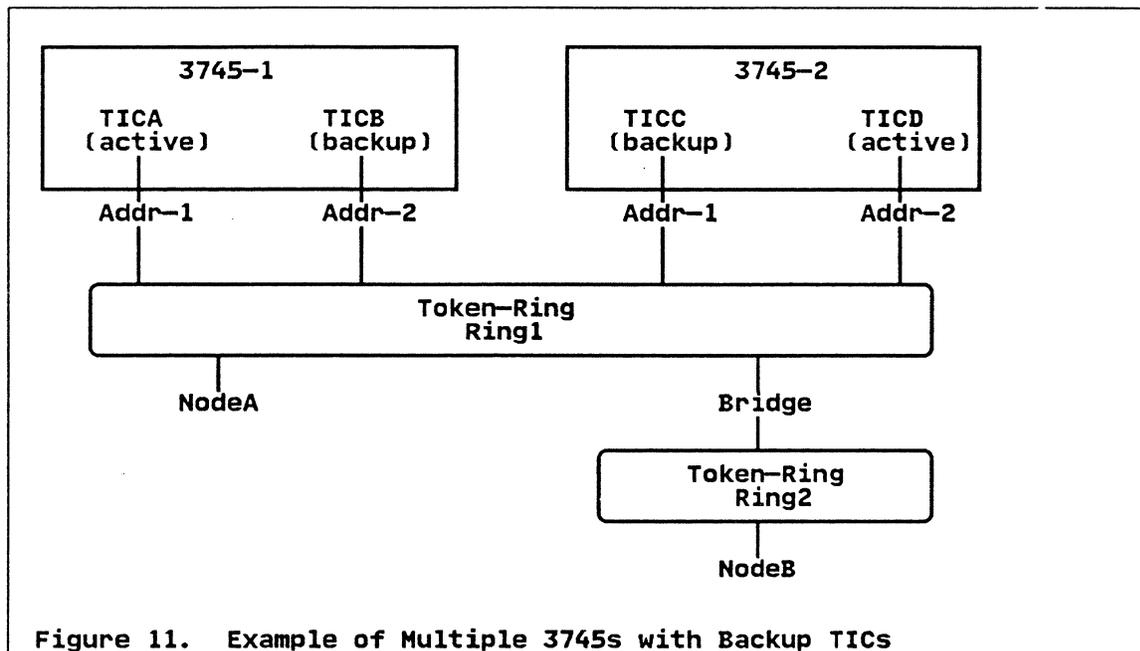
Figure 11. Example of Multiple 3745s with Backup TICs
