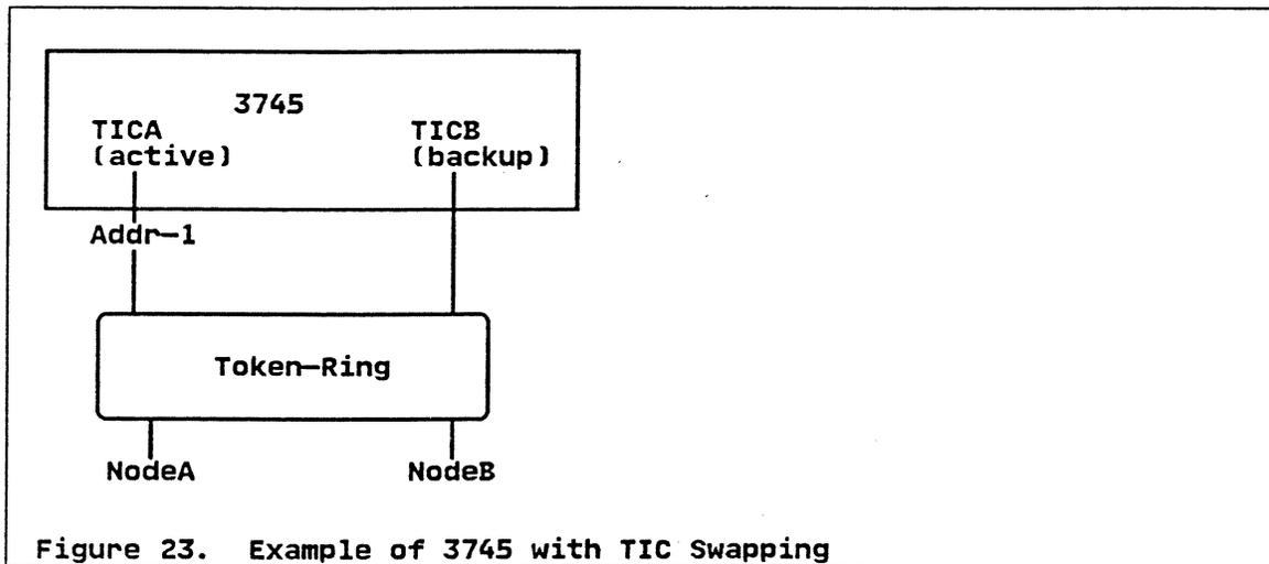
In the above figure, the 3745 is configured with two TICs - TICA and TICB. TICA is defined at address - Addr-1. TICB is not defined to the NCP. NodeA and NodeB are both customized to access the host gateway at Addr-1. Since TICB is an inactive backup, an operator may use TIC swapping to backup any of the TICs in the same NCP. Thus, TIC swapping provides 1 to many backup for TICs.
