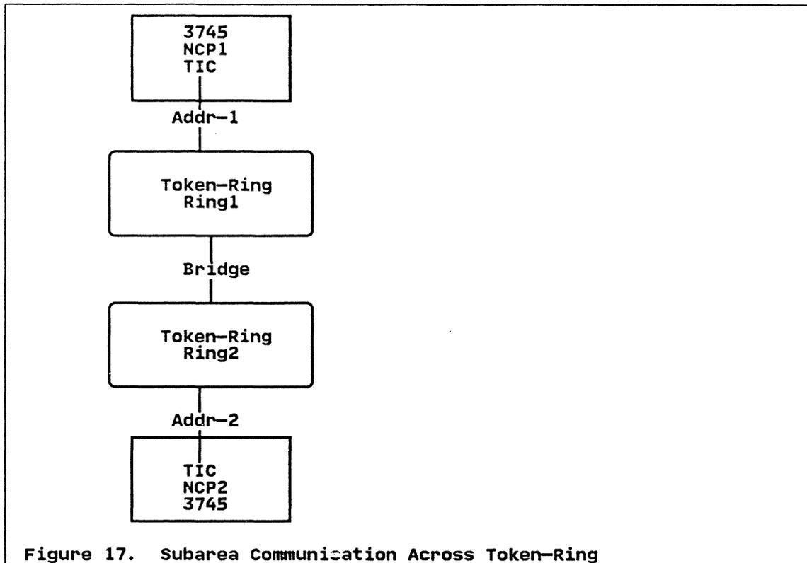
In the figure above, NCP1 connects into Ring1 at address Addr-1, and NCP2 connects into Ring2 at address Addr-2. Ring1 and Ring2 are bridged together and appear as one logical Token-Ring Network. (NOTE: The 3745s could be on the same ring, or the rings could be bridged with remote bridges).
