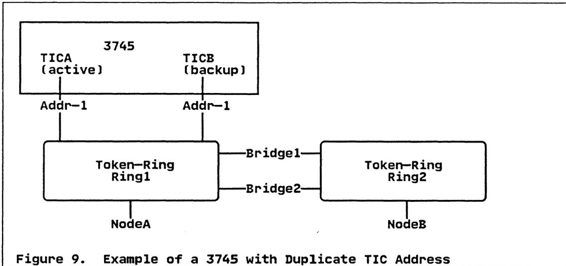
In the above figure, the 3745 is configured with two TICs - TICA and TICB. Both TICA and TICB are defined at the same address - Addr-1 (duplicate TIC addressing requires NCP V5.3, V5.2.1 w/PTF, or V4.3.1 w/PTF). TICA is the active TIC, and TICB is the inactive backup TIC. NodeA and NodeB are peripheral nodes which are customized to access the host gateway at address Addr-1.
