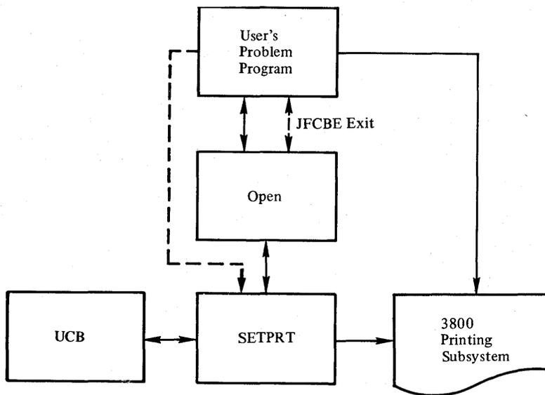
Figure 3. An Overview of Direct Processing to the 3800
