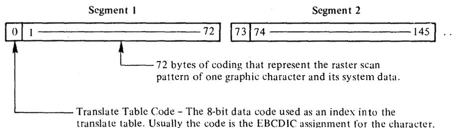
When a graphic character is to be modified, the 3800 uses the translate table code to index into the translate table. The contents found at that location (a 1-byte WCGM code) determine the WCGM location into which the 72 bytes of scan pattern and system data are to be placed.
