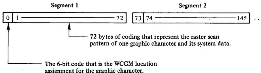
A library character set is loaded directly into a WCGM. SETPRT uses the 6-bit code, contained in the first byte of each 73-byte segment, as the address of the WCGM location into which the remaining 72 bytes are loaded.
