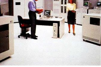
Rack-mounted ES/9000 models contain a compact processor and channel design. This compactness provides new reliability and serviceability and eases your upgrade from IBM ES/9370 processors. A two-sided circuit board used in the rack-mounted design reduces the number of cables needed by integrating the hardware.
