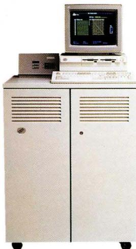
Fibre-optic technology, the physical medium used in this advanced method of channel connectivity, allows data to be transmitted much faster than today's 4.5 MB/sec. data rate – up to a maximum of 10 MB/sec. In addition, you can locate remote functions and disaster-backup equipment far more flexibly than before. ESCON connections also enable you to dynamically add or remove I/O resources while your system remains available to users.
