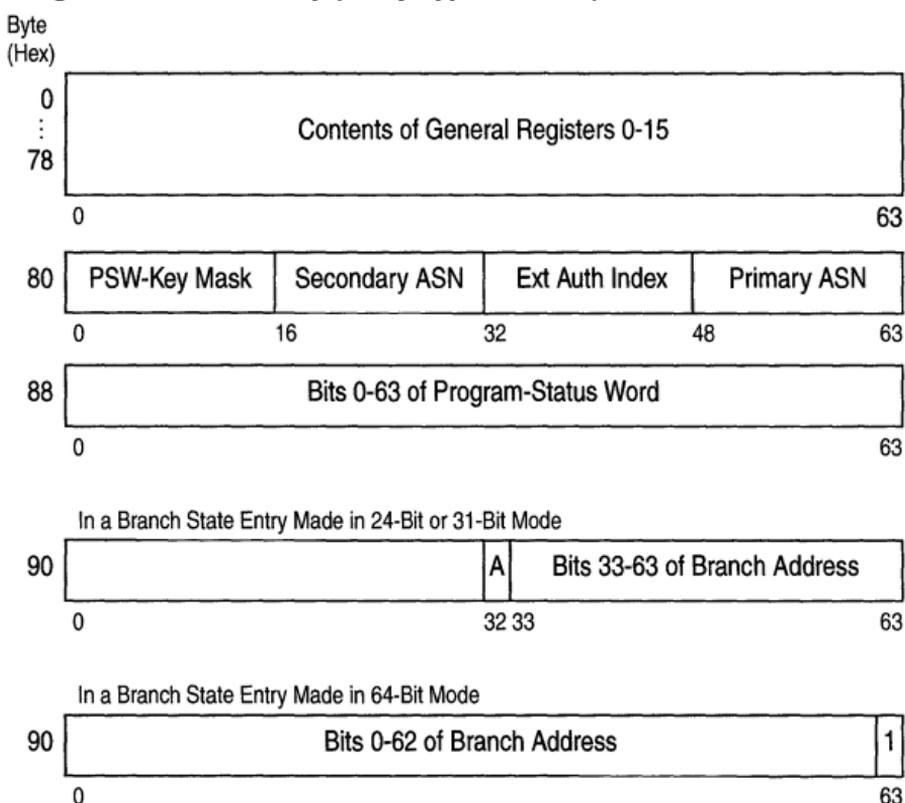
In a Program-Call State Entry Made on a Call to 24-Bit or 31-Bit Mode
