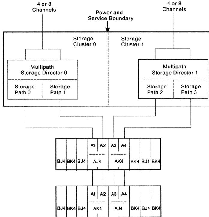
**Note:** The figure shows a maximum configuration of four A-units and 12 B-units. A minimum configuration consists of two A-units in the same string.
