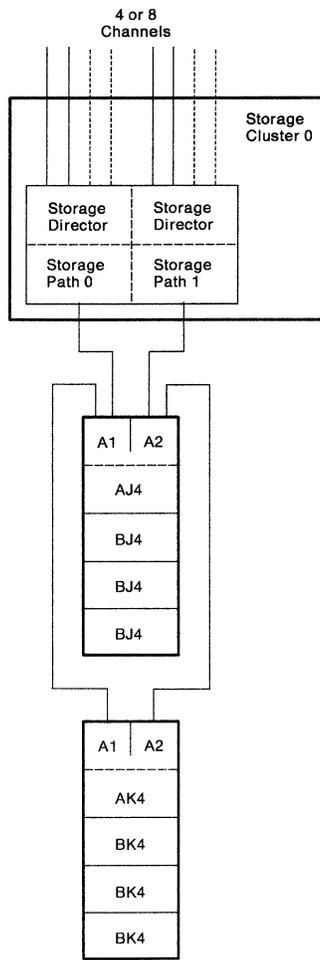
Figure 15. 3990 Model 1 in DLS Mode Attached to 2-Path DASD Strings
