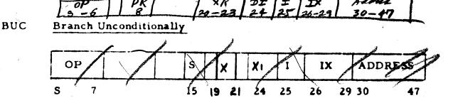
Branching is performed unconditionally, but the S modifier of the instructions, if set to "one," indicates that the Program register is not set from the Program Counter. The index register specified in the X modifier is set from the Program Counter (specifying index register "zero" nullifies this action).
