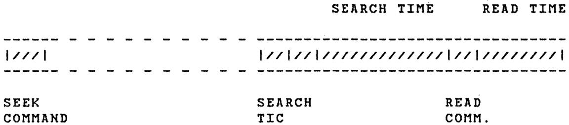
3. BLOCK MULTIPLEXING MODE (less supervisor time than (2))
