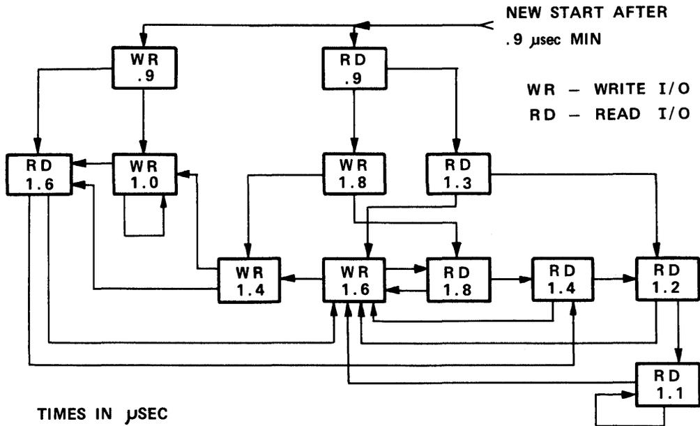
Figure 2.2:: IC Bus Timings, PU Trap level  $\leq 4$
