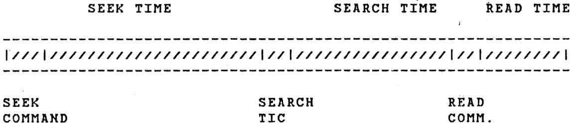
2. SELECTOR CHANNEL WITH SEEK SEPARATION (more supervisor time needed for additional SIO/construction)
