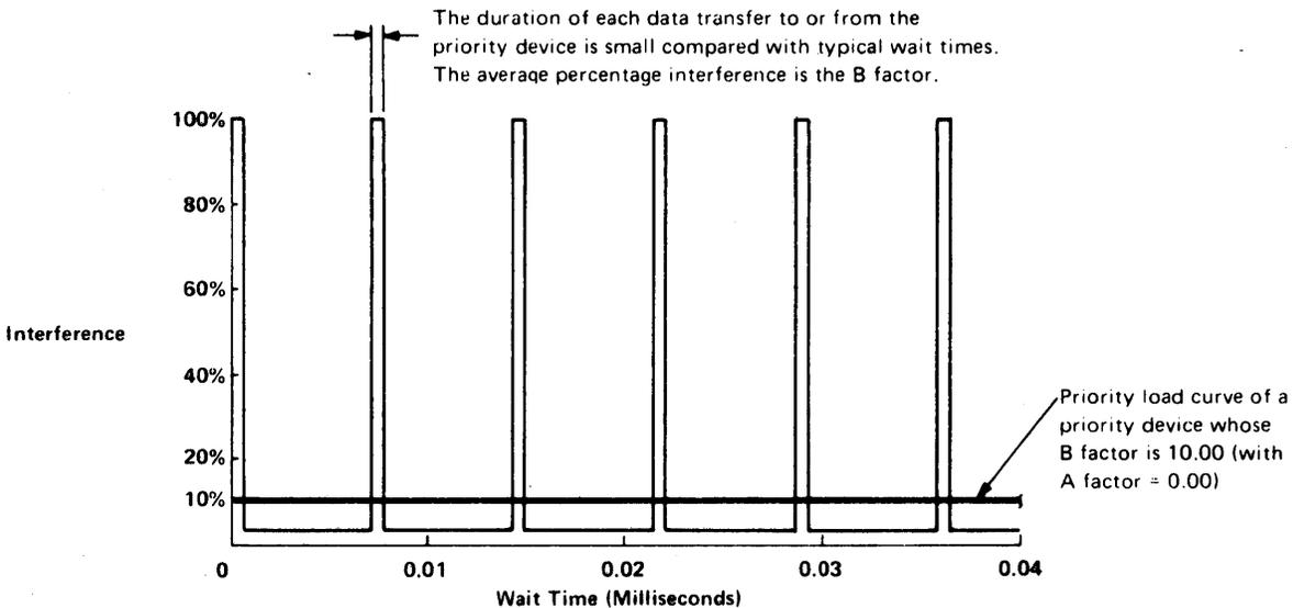
Figure 2.9: Example of Priority Load Curve of a Priority Device Causing Interference by Transferring Data (B-factor Interference)
