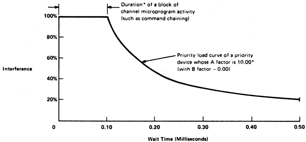
\* The A factor given in the channel evaluation factor tables (in the appendixes) is the duration of interference in milliseconds multiplied by 100. If the duration of interference is 0.10 millisecond (as shown in the illustration), the A factor is  $0.10 \times 100 = 10.00$ . Thus, for a waiting device having a wait time of 0.2 millisecond, the interference is obtained directly as a percentage thus:
