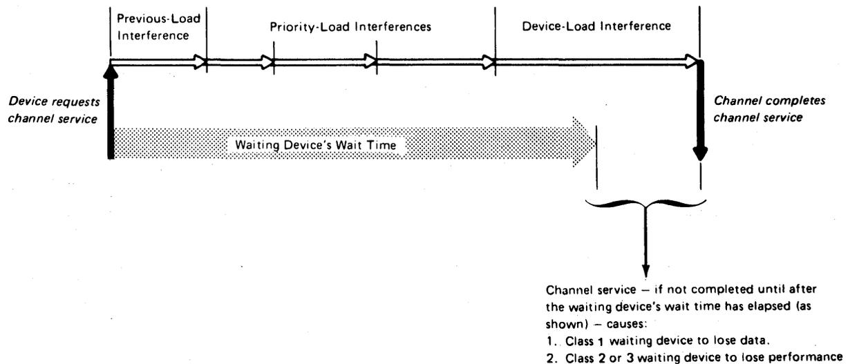
Figure 2.7 Three Kinds of Interference Can Cause Channel Service to be Delayed Beyond a Waiting Device's Wait Time
