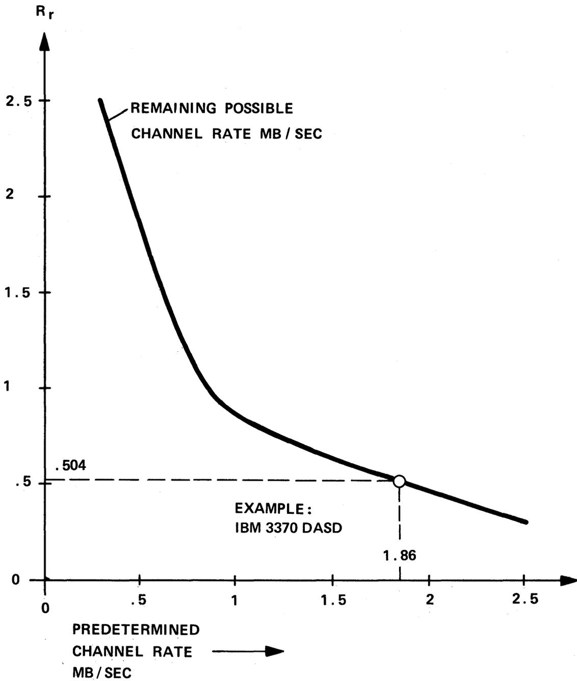
Figure 2.5: Remaining Possible Channel Rates Versus Given, Predetermined Rates
