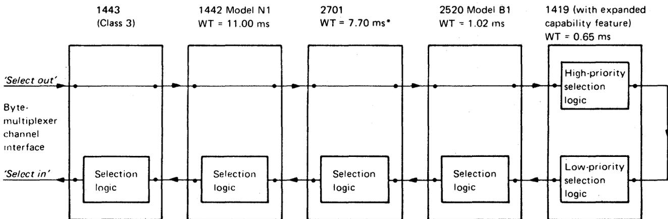
**Figure 2.6: Example Priority Sequence of Devices on the Byte Multiplexer Channel, and 'Select In' and 'Select Out' Line Connections**
