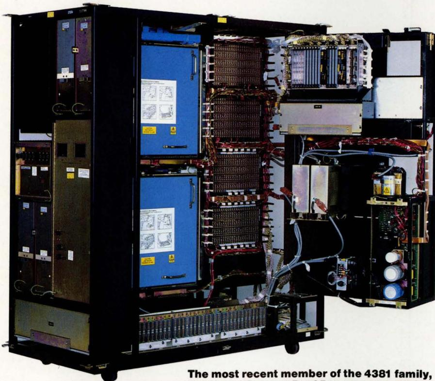
**The most recent member of the 4381 family, the Model Group 3 Dual Processor, contains two processor boards. Each of the two integrated central processors has its own channels and high speed buffer. The engineering/scientific performance of the 4381 Dual Processor is up to 90% greater than the 4381 Model Group 2 Uniprocessor.**
