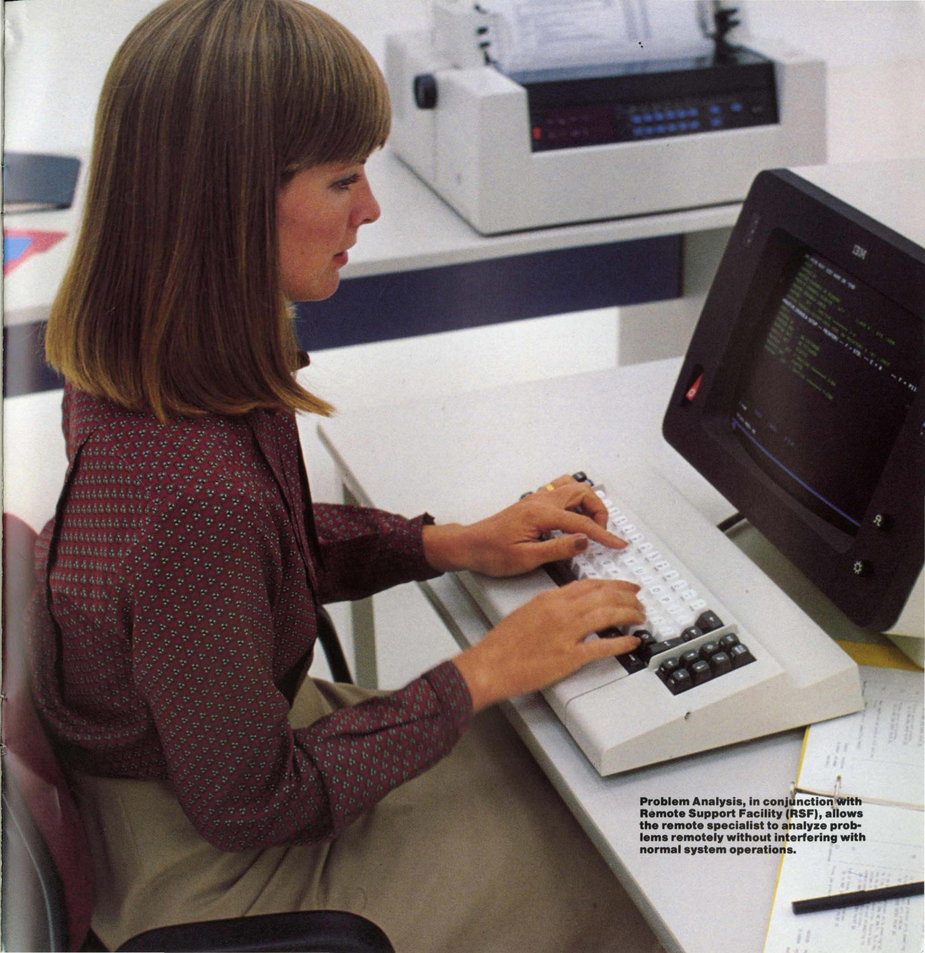
**Problem Analysis, in conjunction with Remote Support Facility (RSF), allows the remote specialist to analyze problems remotely without interfering with normal system operations.**
