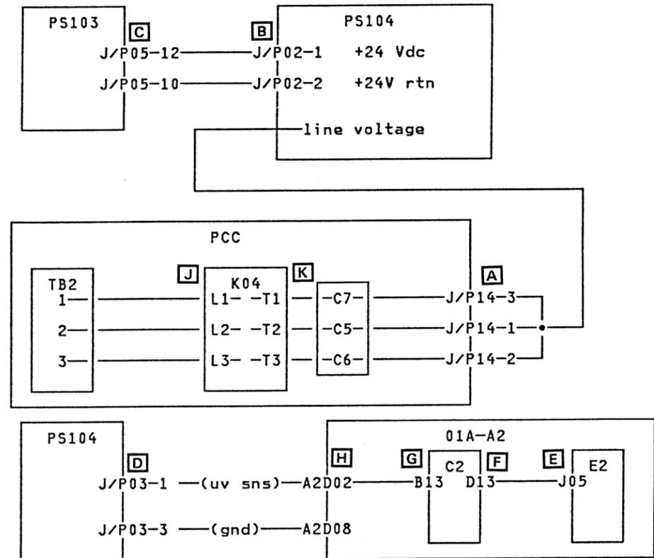
**Note:** UV sense is ground with PU power off; 1.5V with PU power on.
