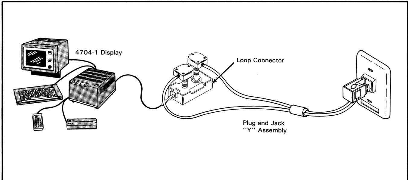
**Figure 2-2. Example of Attaching a Device to a Cabling System Receptacle**
