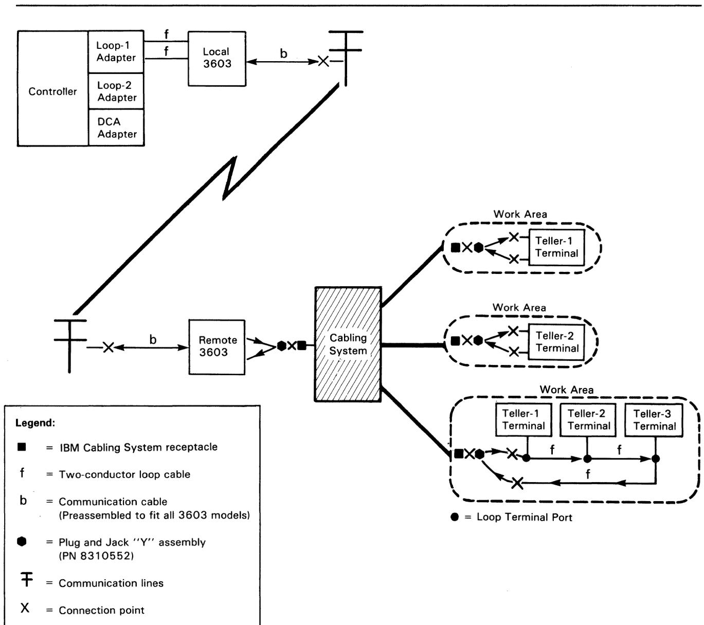
Figure 2-4. Attaching a Remote Loop to the Cabling System
