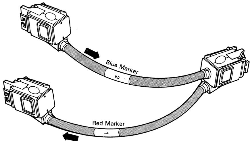
**Note:** Remember, the cabling system "Y" assembly is color-coded. Pay close attention to how you connect these assemblies.
