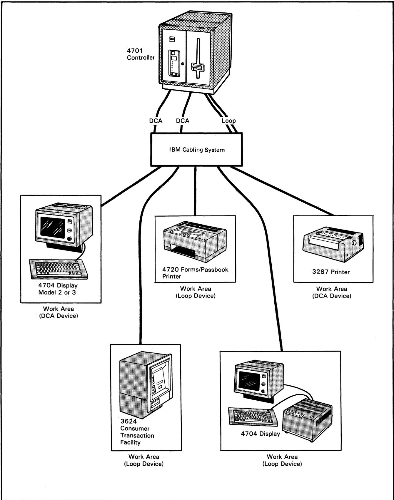
Figure 1-1. A 4700 or 3600 System Configuration with the Cabling System
