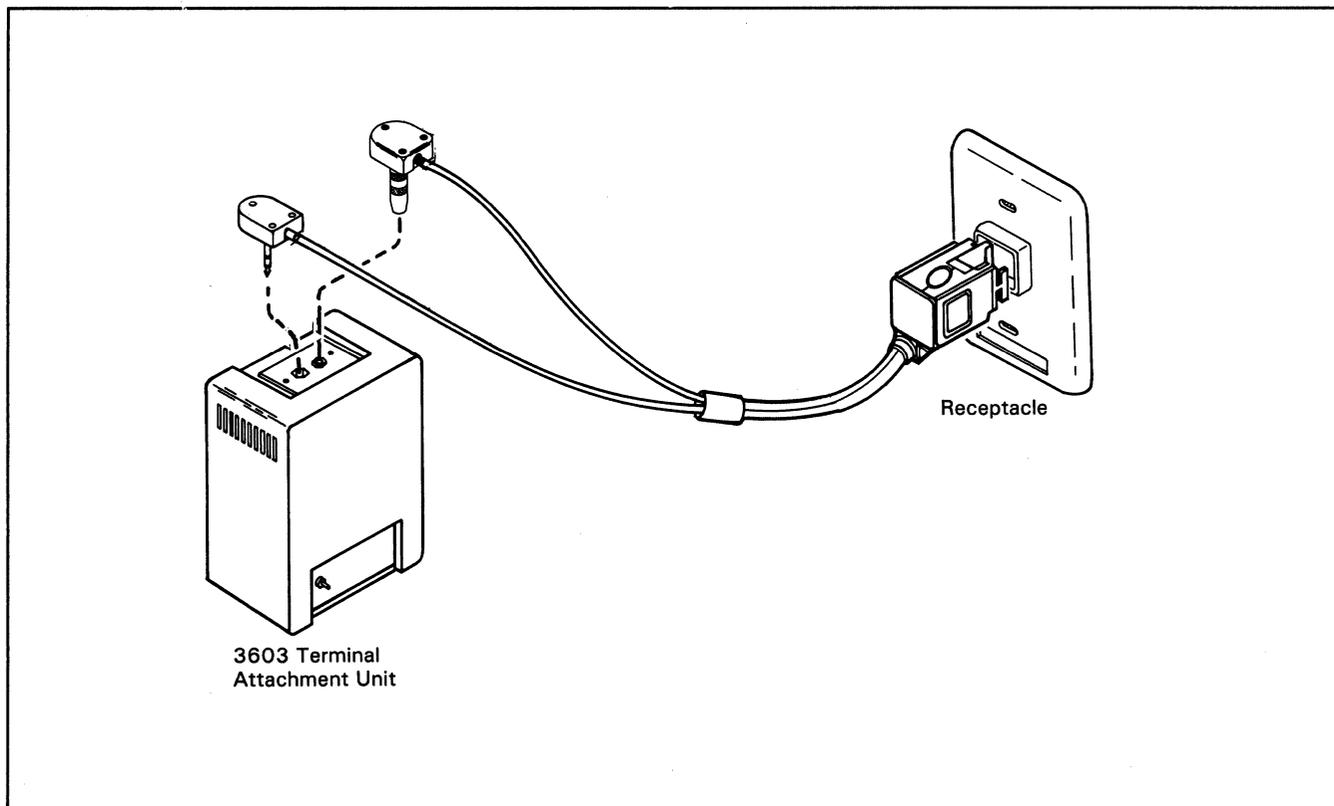
**Figure 2-5. Example of Attaching a 3603 to a Cabling System Receptacle**
