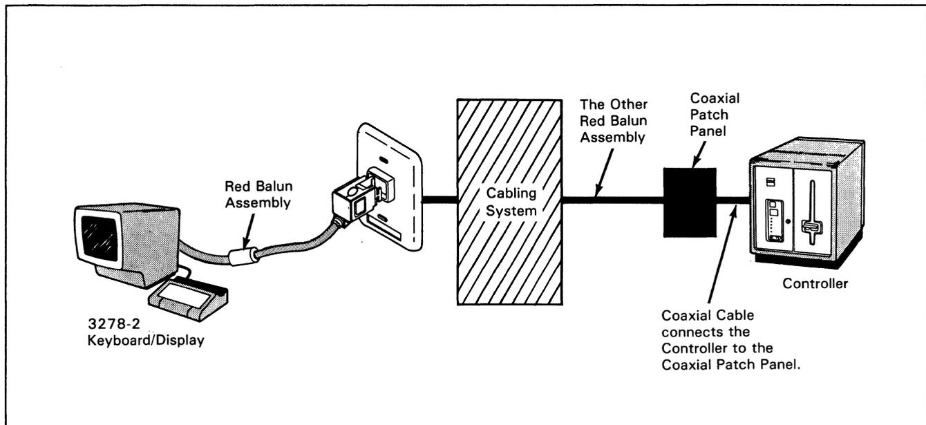
Figure 3-1. Connecting a DCA Device Using Cabling System (Method 1)
