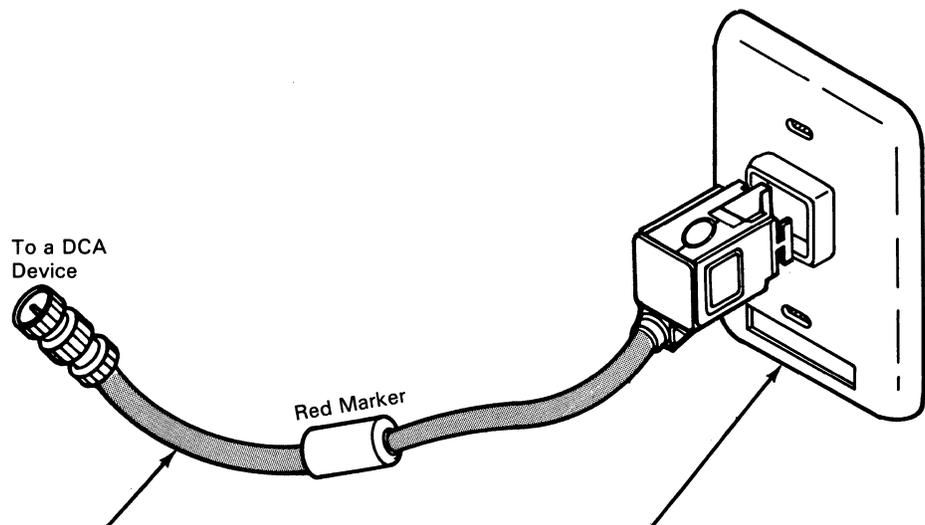
The Red Balun assembly connects DCA devices to cabling system receptacles.
