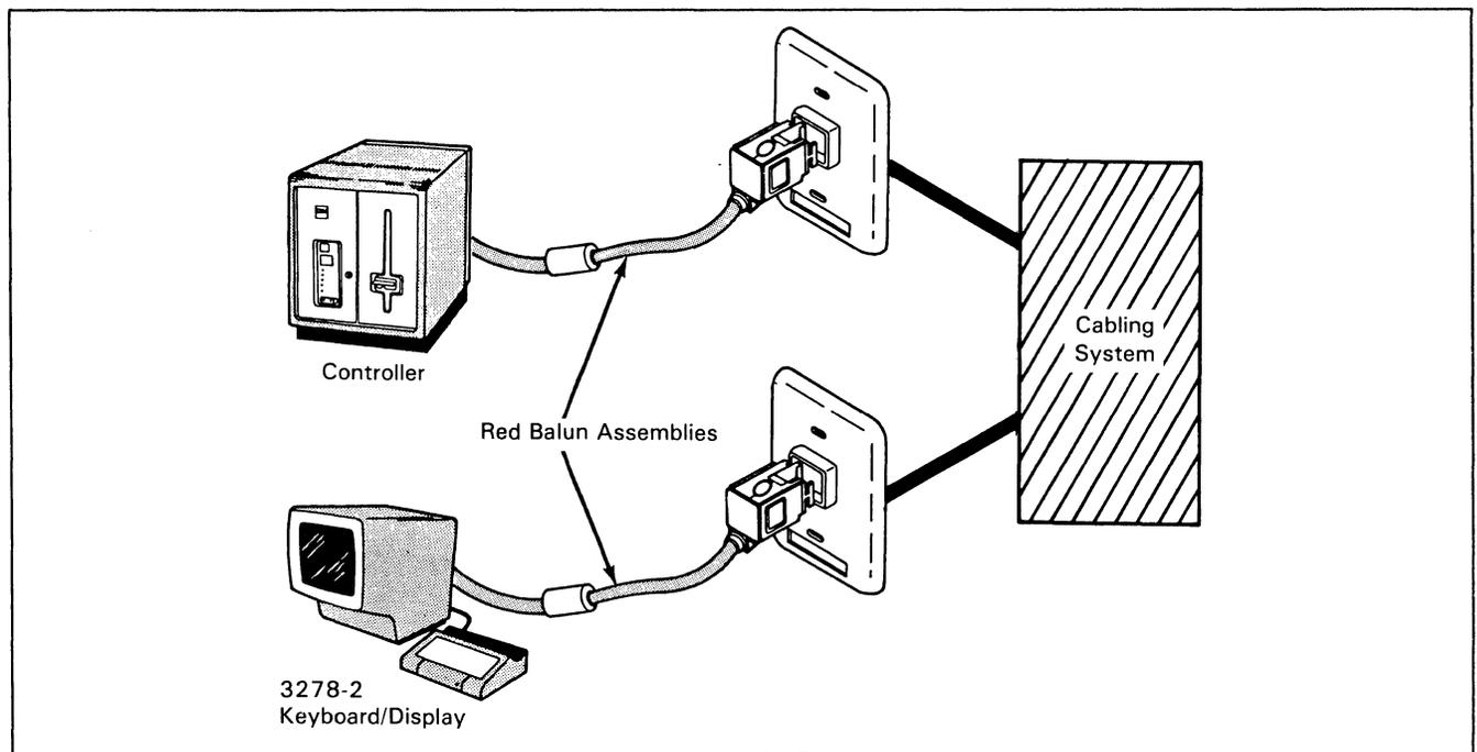
Figure 3-2. Connecting DCA Using Cabling System (Method 2)
