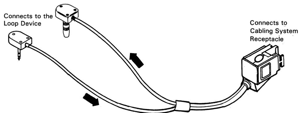
This assembly connects loop devices to the cabling system receptacle. This assembly has the same plug and jack receptacles as the loop terminal ports described in your 4700 or 3600 installation planning manual.
