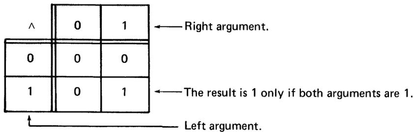
The And function is used to check for two conditions being true.
