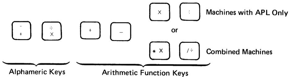
Four commonly used built-in functions (+ - x ÷) perform the normal arithmetic operations when they are used. These symbols are located on the top row of the alphameric keys and also to the right of the numeric keys.
