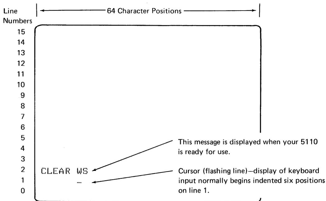
There are 128 positions available for input from the keyboard; that is, there are 64 positions available on line 1 and 64 positions on line 0. When position 64 of line 1 is used as you enter data from the keyboard, the cursor moves to the left margin of line 0. The cursor is then at position 65 of the possible 128 positions available for input.
