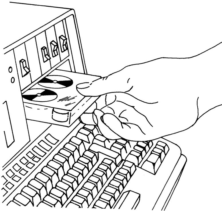
Figure 7. Inserting a Cartridge Into the 5110 Model 1
