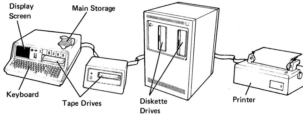
**Figure 2. 5110 Model 1 Computing System Data Processing Elements**
